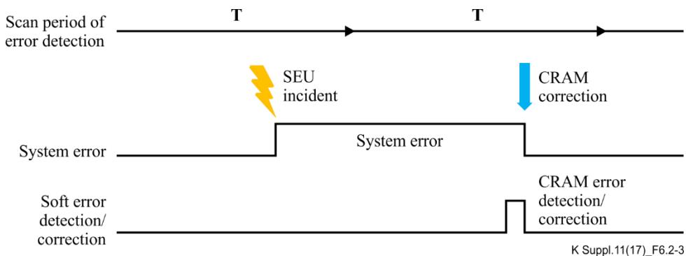
**Figure 6.2-3 – Example of an operation when a soft error occurs**
