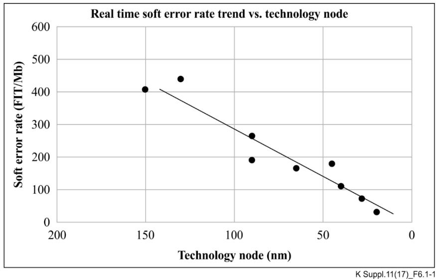
**Figure 6.1-1 – Example of CRAM soft error rate vs. feature size (technology node)**
