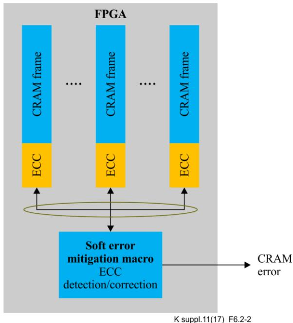
**Figure 6.2-2 – Example of soft error reduction macro configuration
