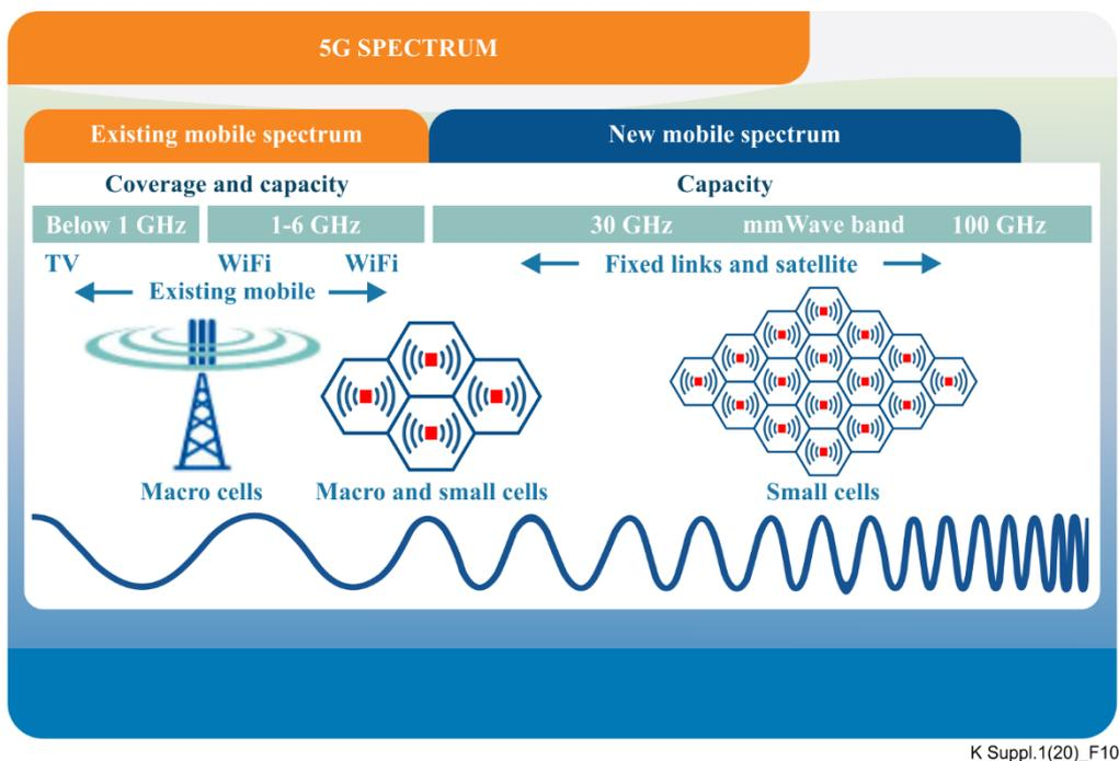
Figure 10 – Spectrum used by mobile communication
