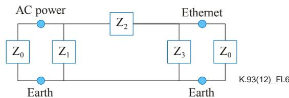
\*  $Z_0 = 150 [\Omega]$ : internal impedance of CDN
