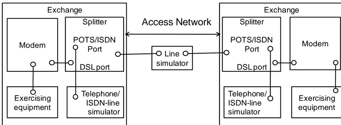
**Figure A.1 – DSL access system configuration**
