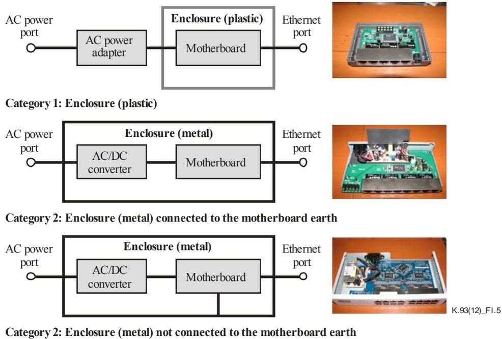
Figure I.5 – Categories of IP-based communication devices
