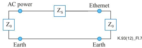
\*  $Z_0 = 150 \text{ } [\Omega]$ : internal impedance of CDN
