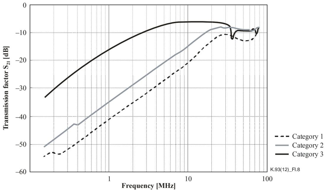
**Figure I.8 – Transmission factors  $S_{21}$  for three categorized models**
