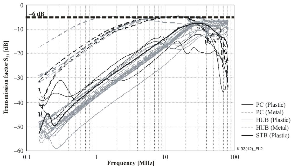
**Figure I.2 – Measured transmission factors of IP-based communication devices**
