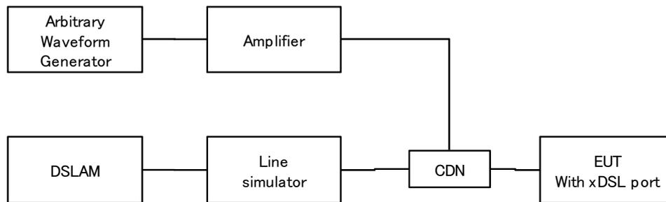
**Figure 1 – Example block diagram of the test set-up**
