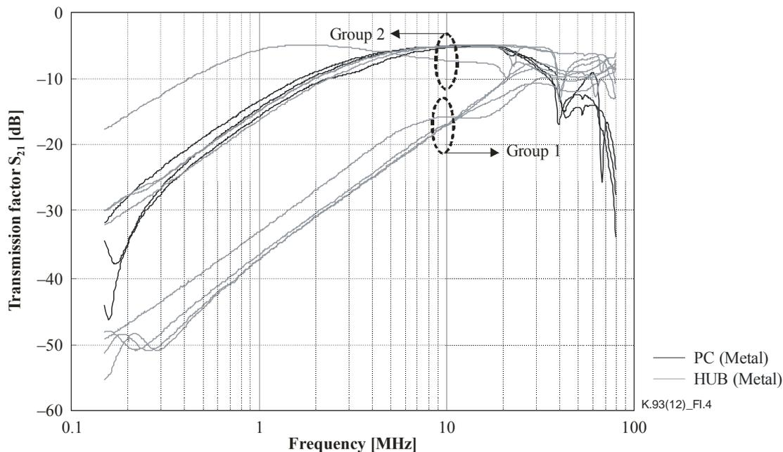
**Figure I.4 – Transmission factors for devices with metal frames**
