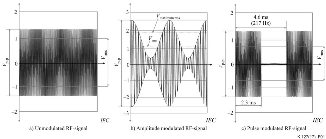
**Figure 1 – Waveforms for test level calibration and for the test (from [IEC 61000-4-39])<sup>1</sup>**
