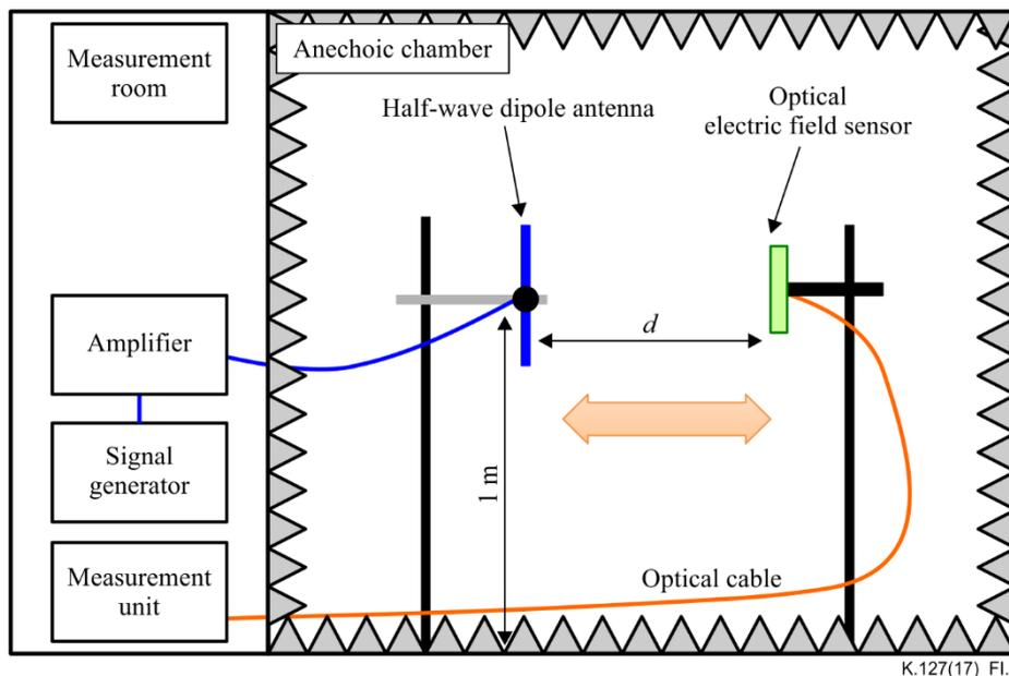
Figure I.1 – Measurement set-up for the electric field strength
