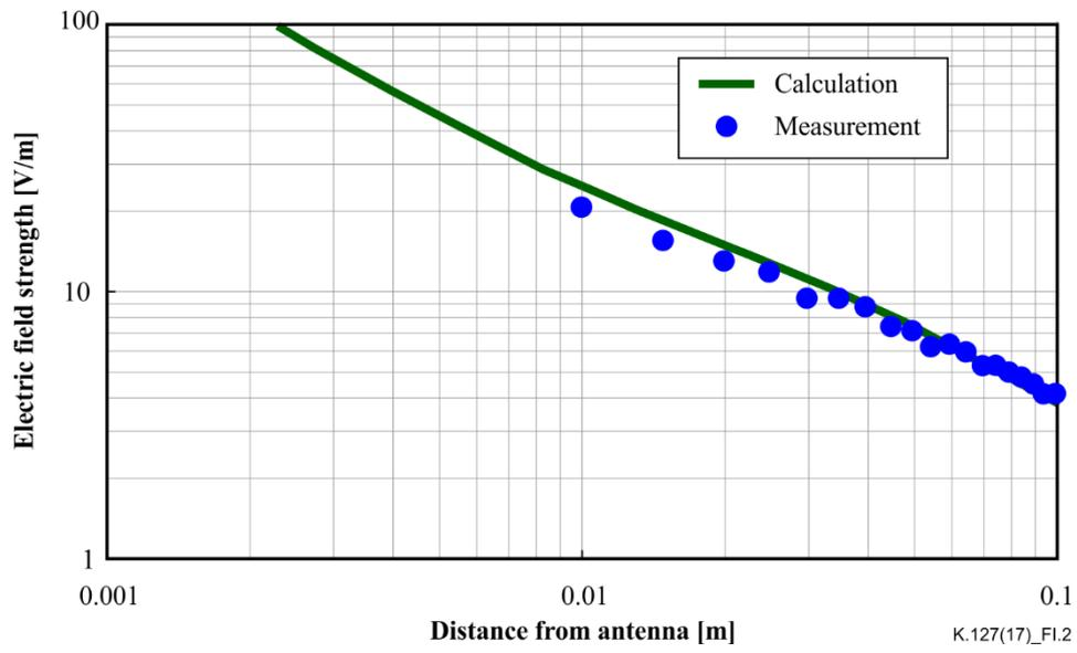
**Figure I.2 – Measurement results of electric field strength in the vicinity of the antenna**
