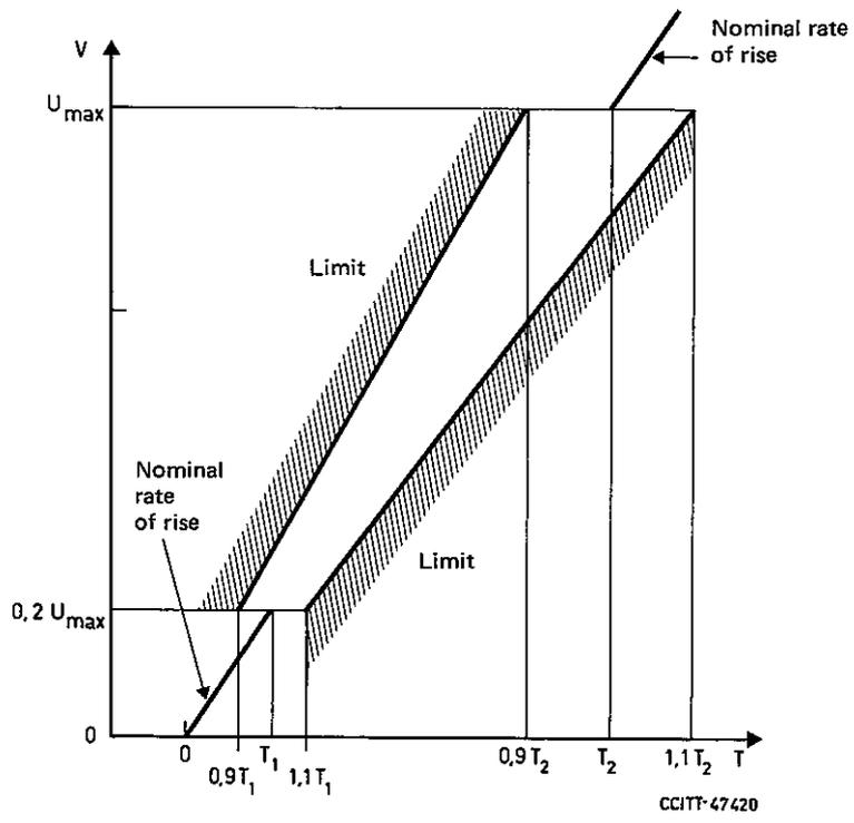
Note – Spark-over test waveform (nonconducting) must be within enclosed limits.
