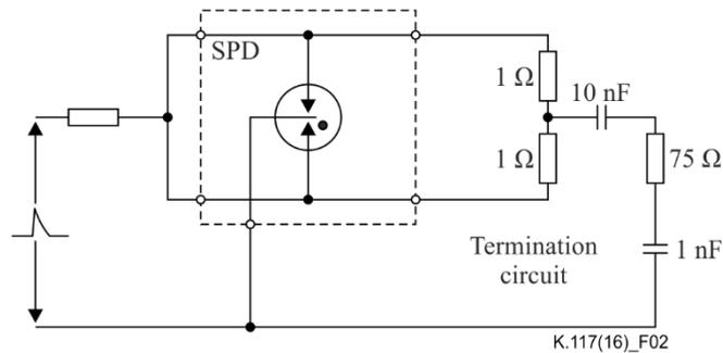
**Figure 2 – GDT common-mode voltage limiting (partial circuit for only one twisted pair)**
