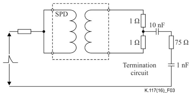
**Figure 3 – Isolating transformer common-mode voltage blocking (partial circuit for only one twisted pair)**
