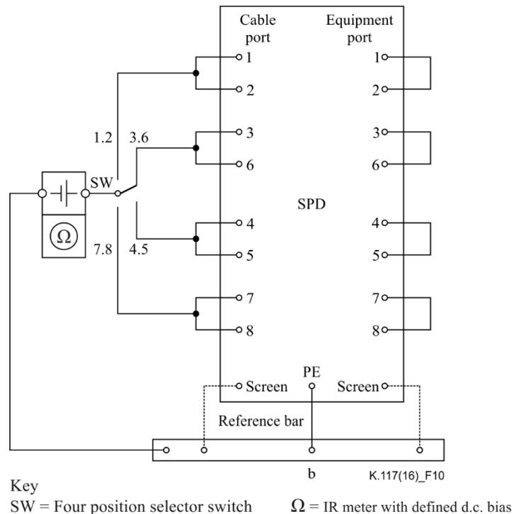
**Figure 10 – Test circuit to measure the insulation resistance of an SPD with a PE terminal or screen terminals, or both**
