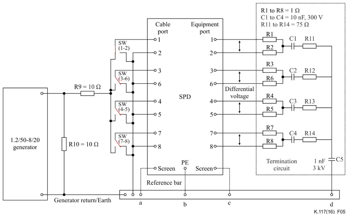
**Figure 5 – Single twisted-pair differential-mode surge test circuit**
