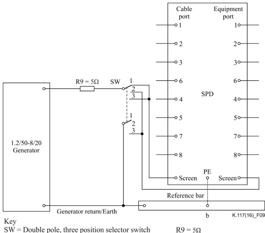
**Figure 9 – Screen bonding test**
