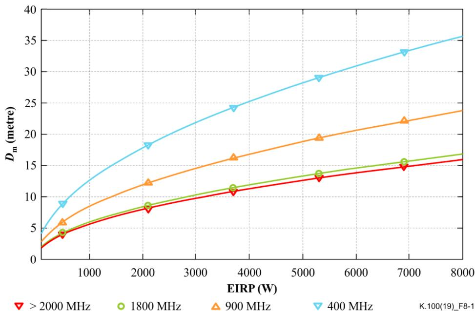
**Figure 8-1 –  $D_m$  as a function of the equivalent isotropically radiated power obtained from Equations 8-1 to 8-3**
