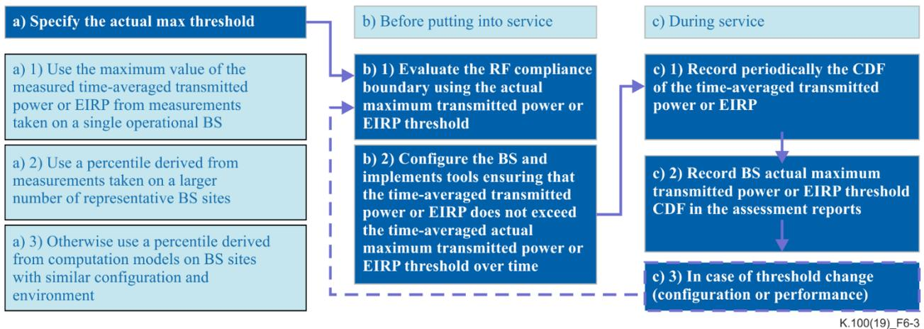
**Figure 6-3 – Flow chart for assessing compliance for a BS site sector or sub-division of a BS site sector [b-IEC TR 62669]**
