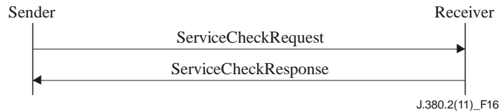
Figure 16 – Service check message exchange
