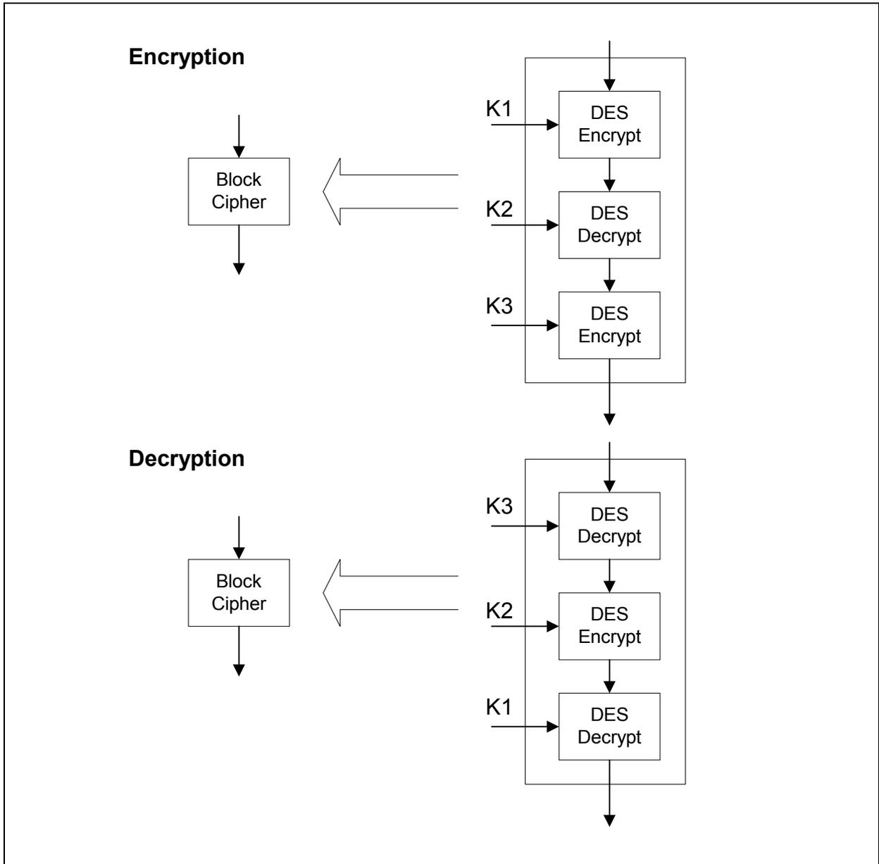
Figure 29. 3DES-EDE as Block Cipher
