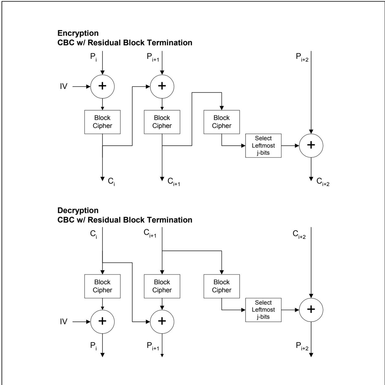
Figure 30. CBC with Residual Block Termination
