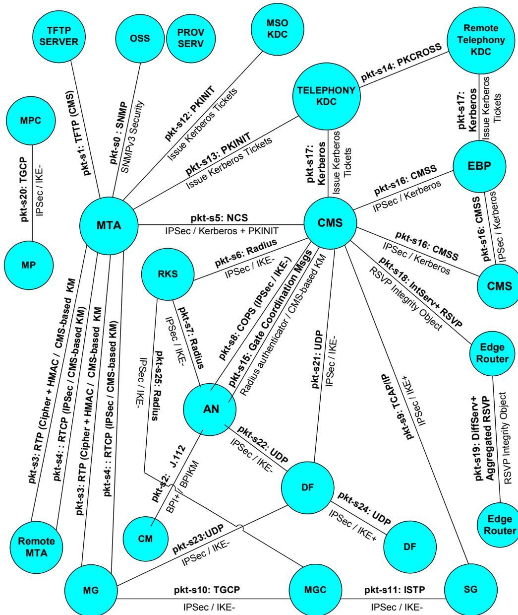
Figure 3. IPCablecom Security Interfaces with Key-Management
