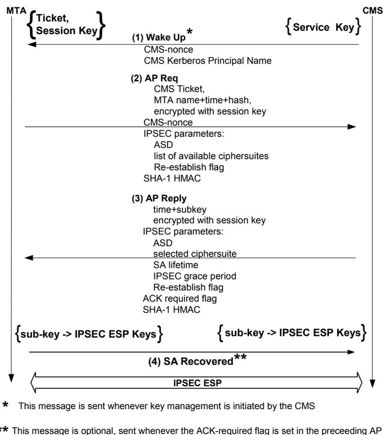
Figure 9. Kerberos AP Request / AP Reply Exchange
