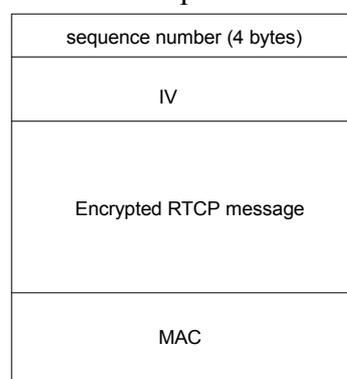
**Figure 21. RTCP Encrypted Packet Format**
