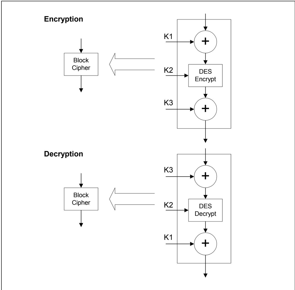
Figure 28. DESX-XEX as Block Cipher
