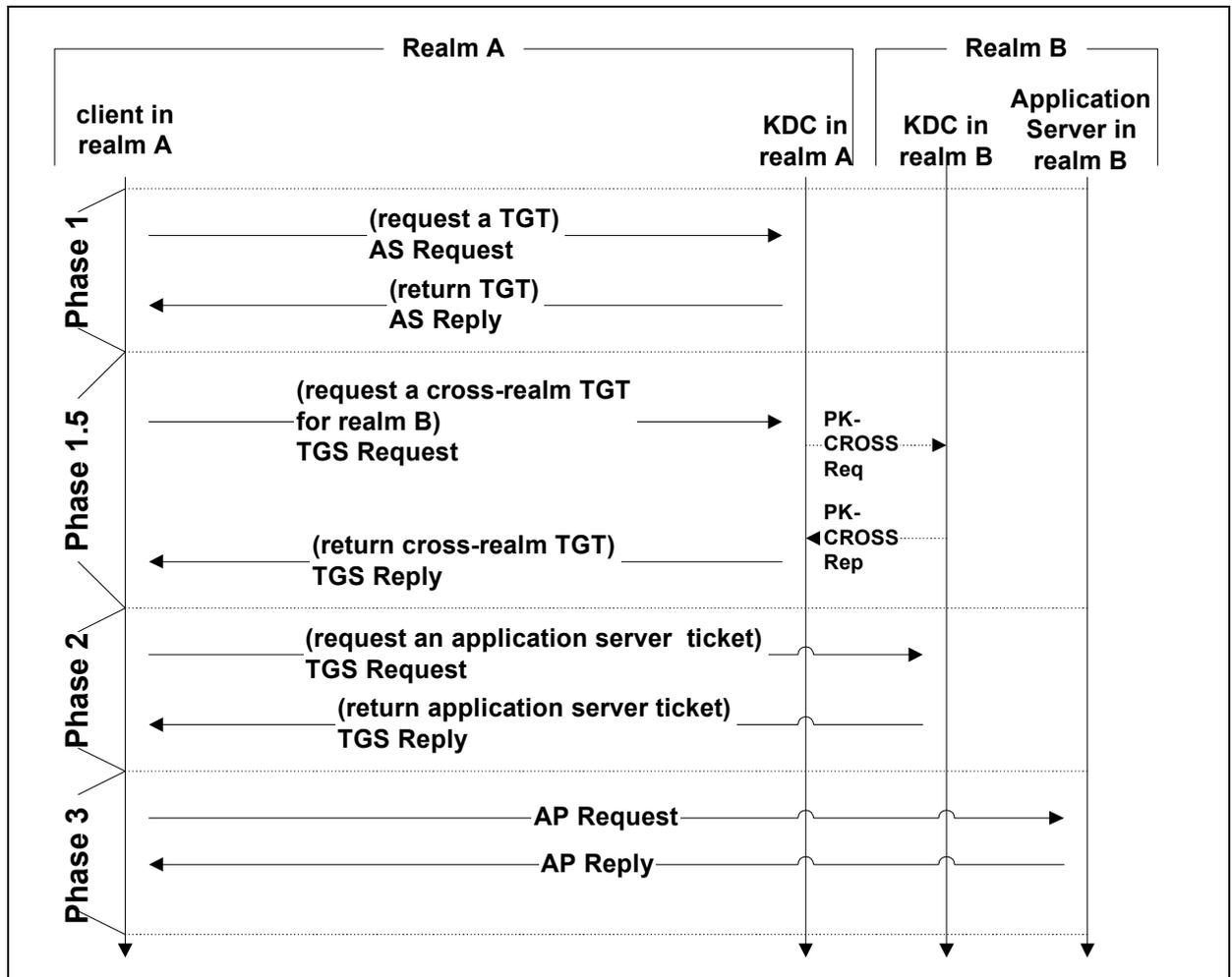
Figure 8. Kerberos Cross-Realm Operation
