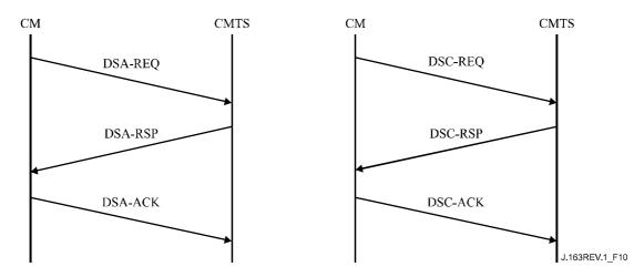
Figure 10/J.163 - DSA and DSC exchanges between CM and CMTS
