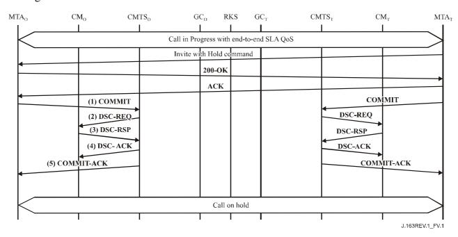
Figure V.1/J.163 - QoS signalling for Call Hold
