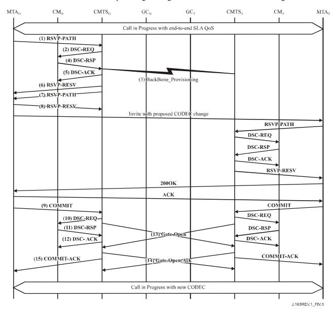
Figure IV.1/J.163 – QoS signalling for codec change
