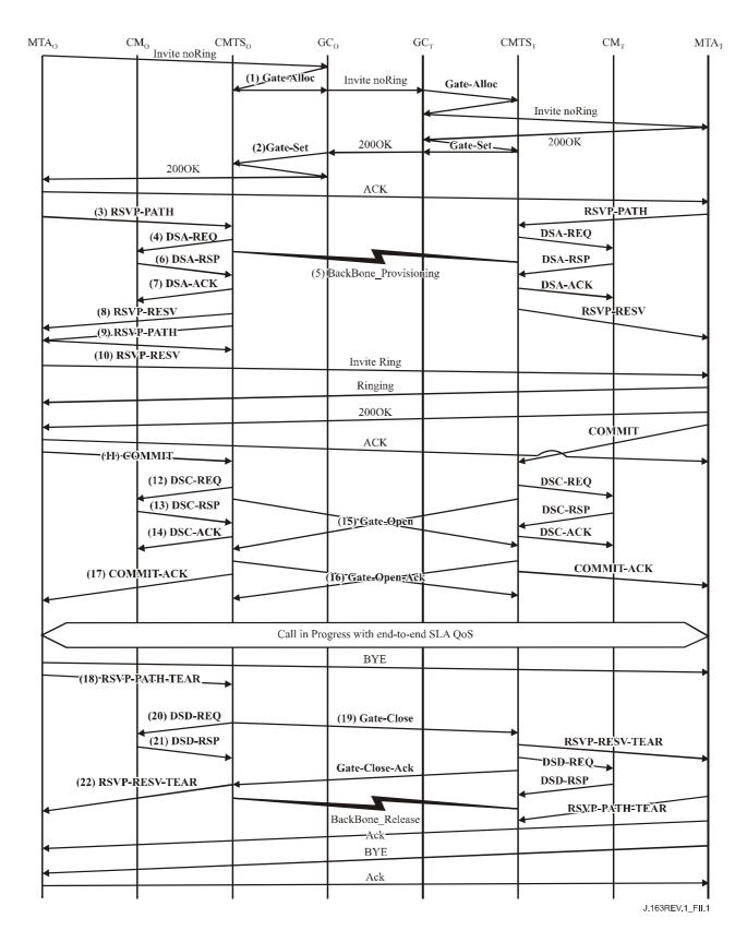
Figure II.1/J.163 - Basic call flow - DCS signalling
