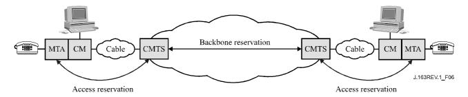
Figure 6/J.163 – Segmented signalling model
