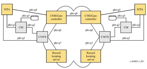
Figure 1/J.163 – QoS signalling interfaces in IPCablecom network
