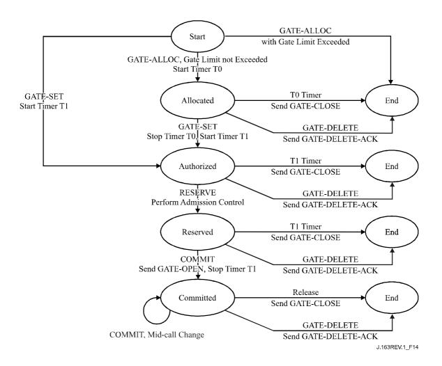
Figure 14/J.163 – Gate state transition diagram
