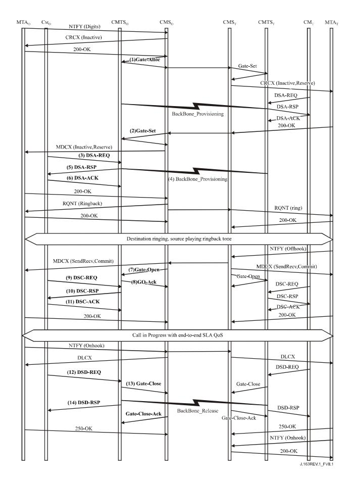
Figure VII.1/J.163 - Basic call flow - Embedded MTA
