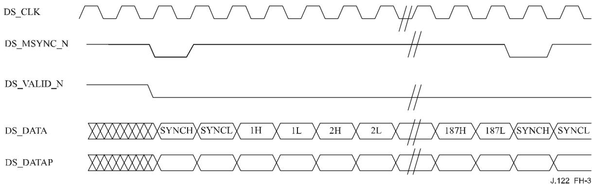
**Figure H.3 – Downstream data signal protocol for J.83 Annex B operation**
