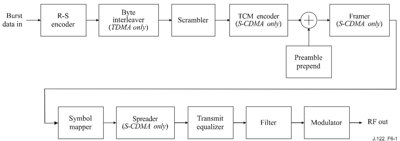
**Figure 6-1 – Upstream signal-processing sequence**
