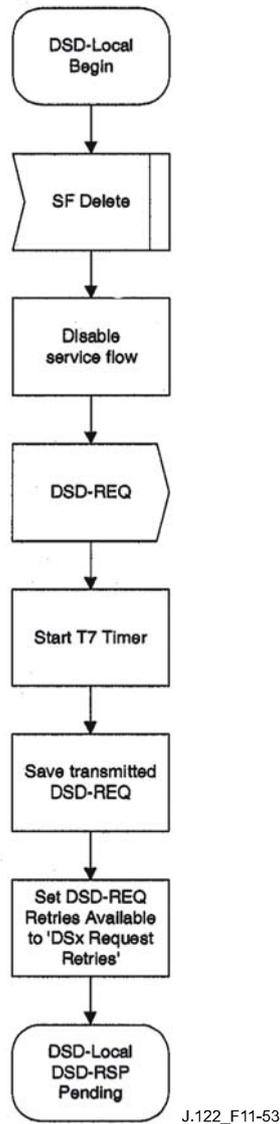
Figure 11-53 – DSD – Locally-initiated transaction begin state flow diagram
