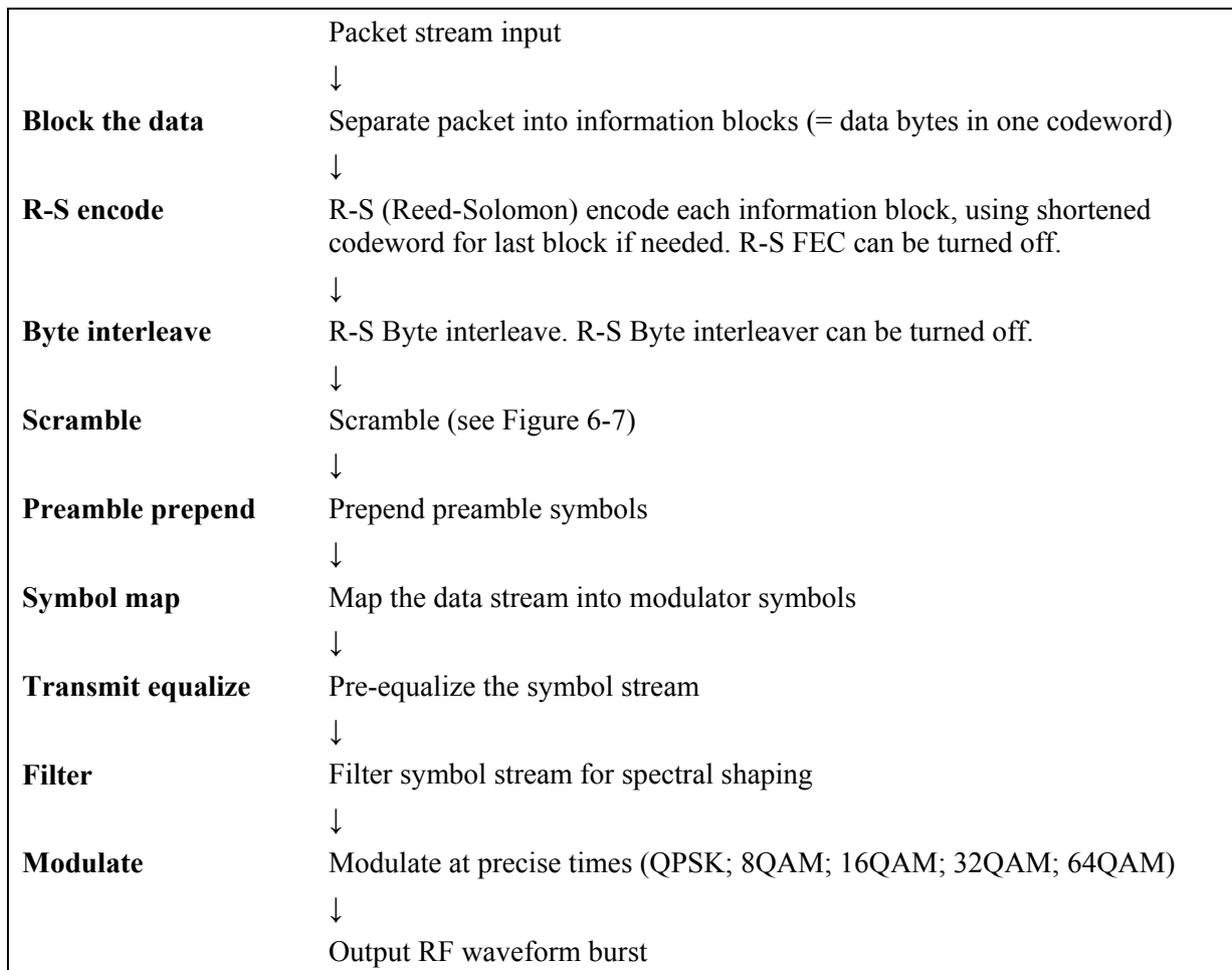
**Figure 6-2 – TDMA upstream transmission processing**
