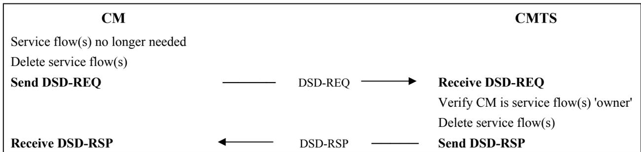
**Figure 11-51 – Dynamic service deletion initiated from CM**
