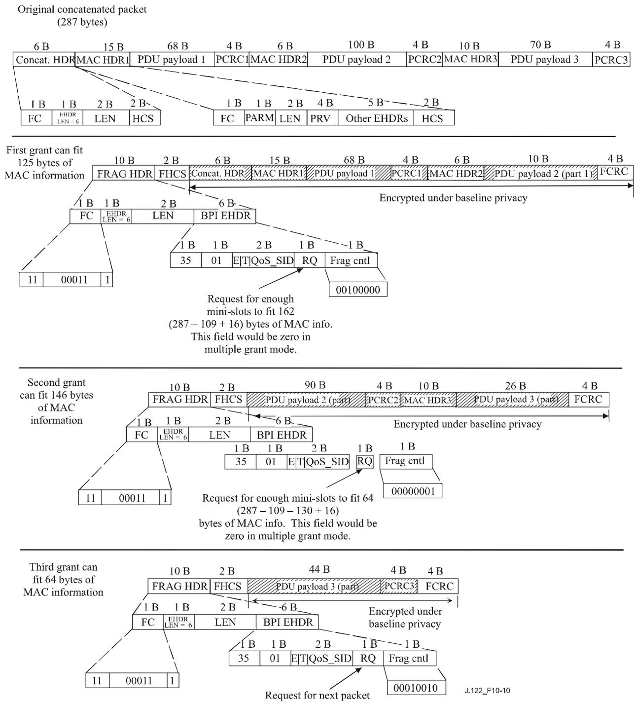
Figure 10-10 – Fragmented concatenated packet example
