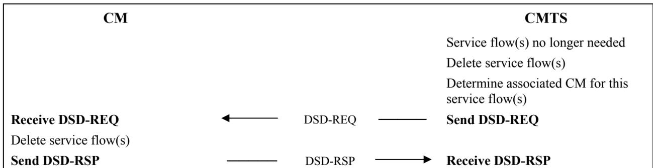
**Figure 11-52 – Dynamic service deletion initiated from CMTS**
