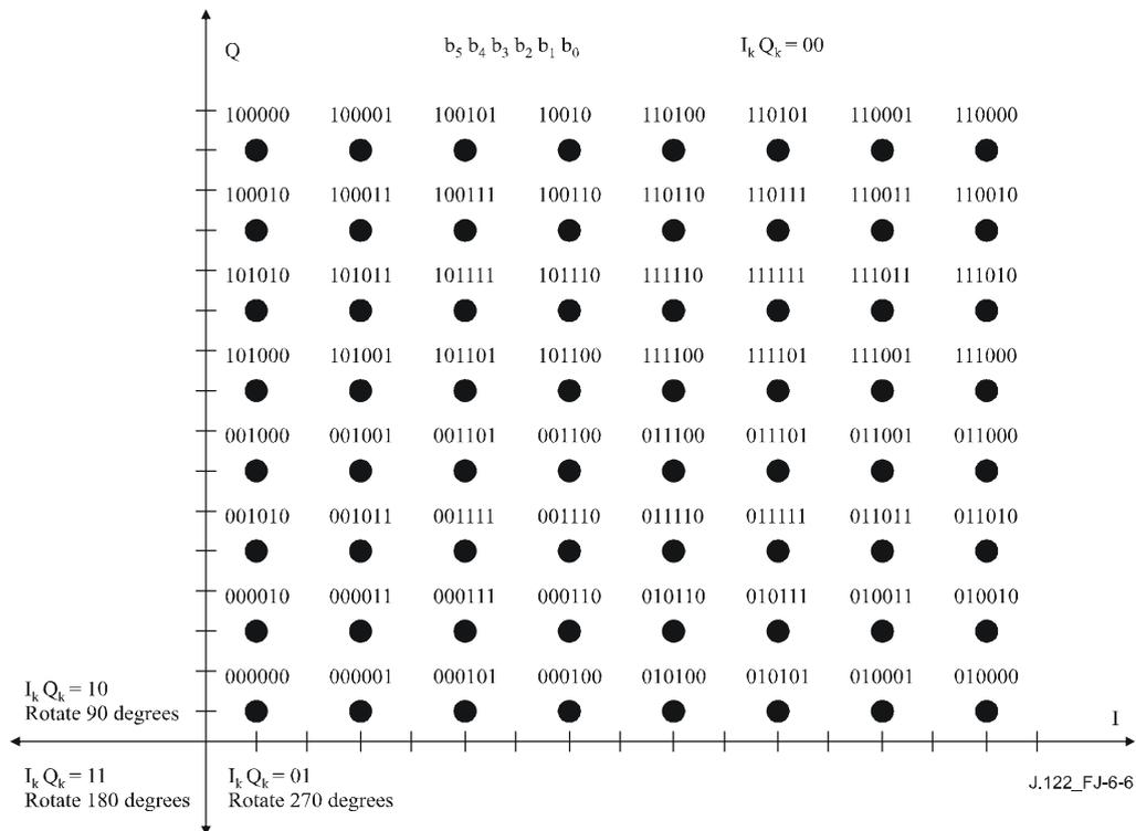
**Figure J.6-6 – 256QAM signal constellation diagram and phase shift rule (I = 12)**
