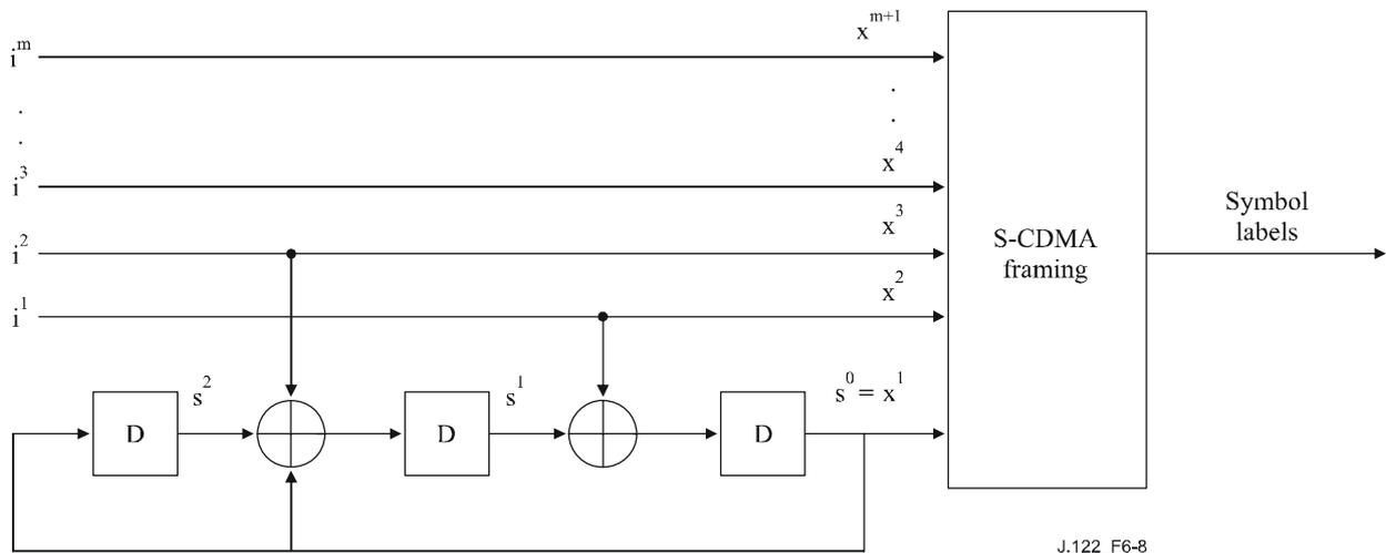
**Figure 6-8 – Convolutional encoder**
