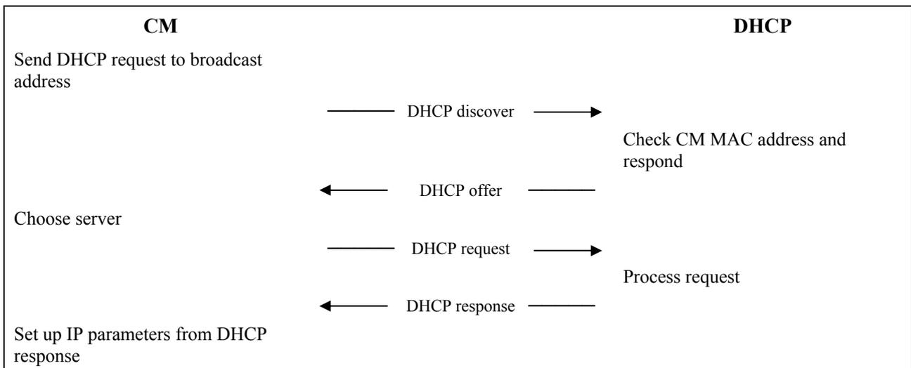
**Figure 11-10 – Establishing IP connectivity**
