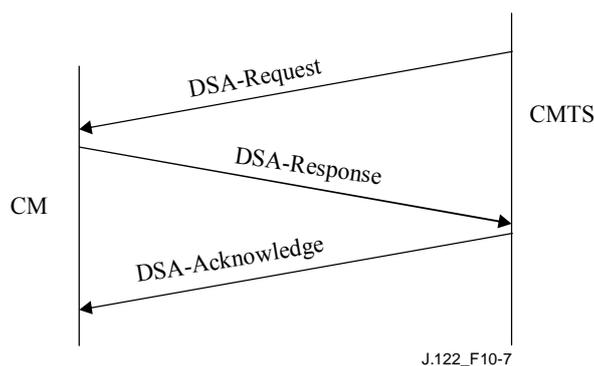
**Figure 10-7 – Dynamic service addition message flow – CMTS-initiated**
