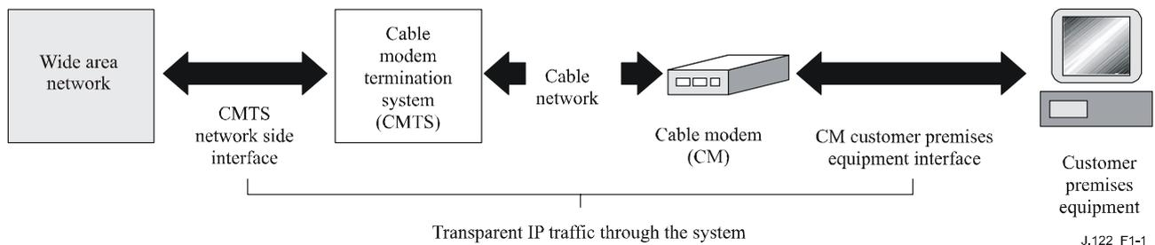
**Figure 1-1 – Transparent IP traffic through the data-over-cable system**
