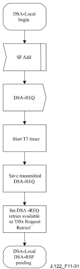
**Figure 11-31 – DSA – Locally-initiated transaction begin state flow diagram**
