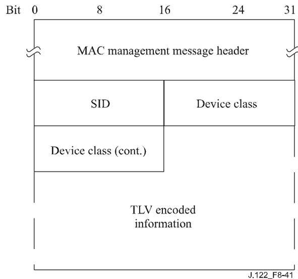
**Figure 8-41 – Device class identification request**
