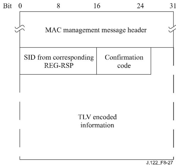
**Figure 8-27 – Registration acknowledgment**
