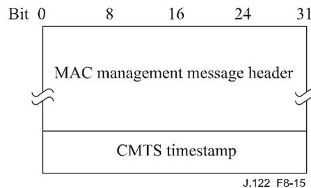
**Figure 8-15 – Format of packet PDU following the timing header**
