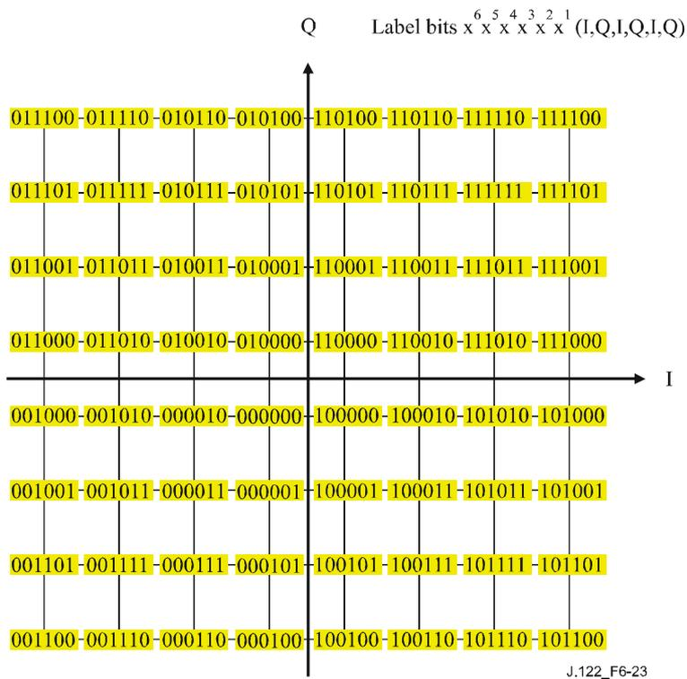
**Figure 6-23 – 64QAM symbol mapping**
