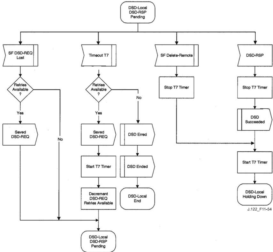
Figure 11-54 – DSD – Locally-initiated transaction DSD-RSP pending state flow diagram
