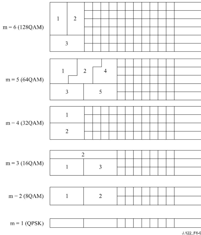
**Figure 6-9 – Repetitive patterns of byte mapping to symbol map bits for TCM**
