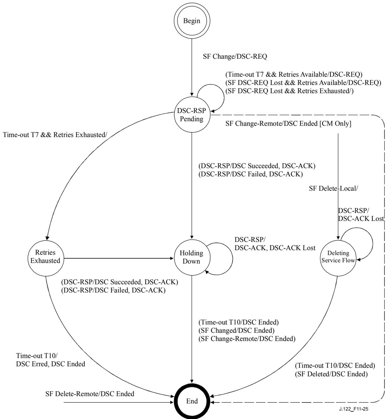
**Figure 11-25 – DSC – Locally-initiated transaction state transition diagram**
