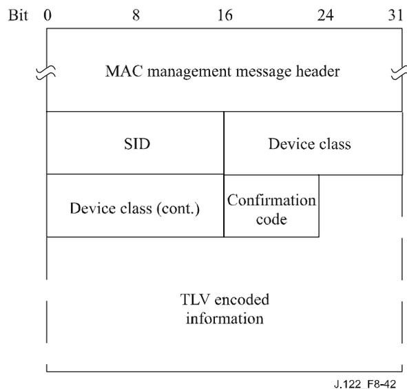
**Figure 8-42 – Device class identification response**
