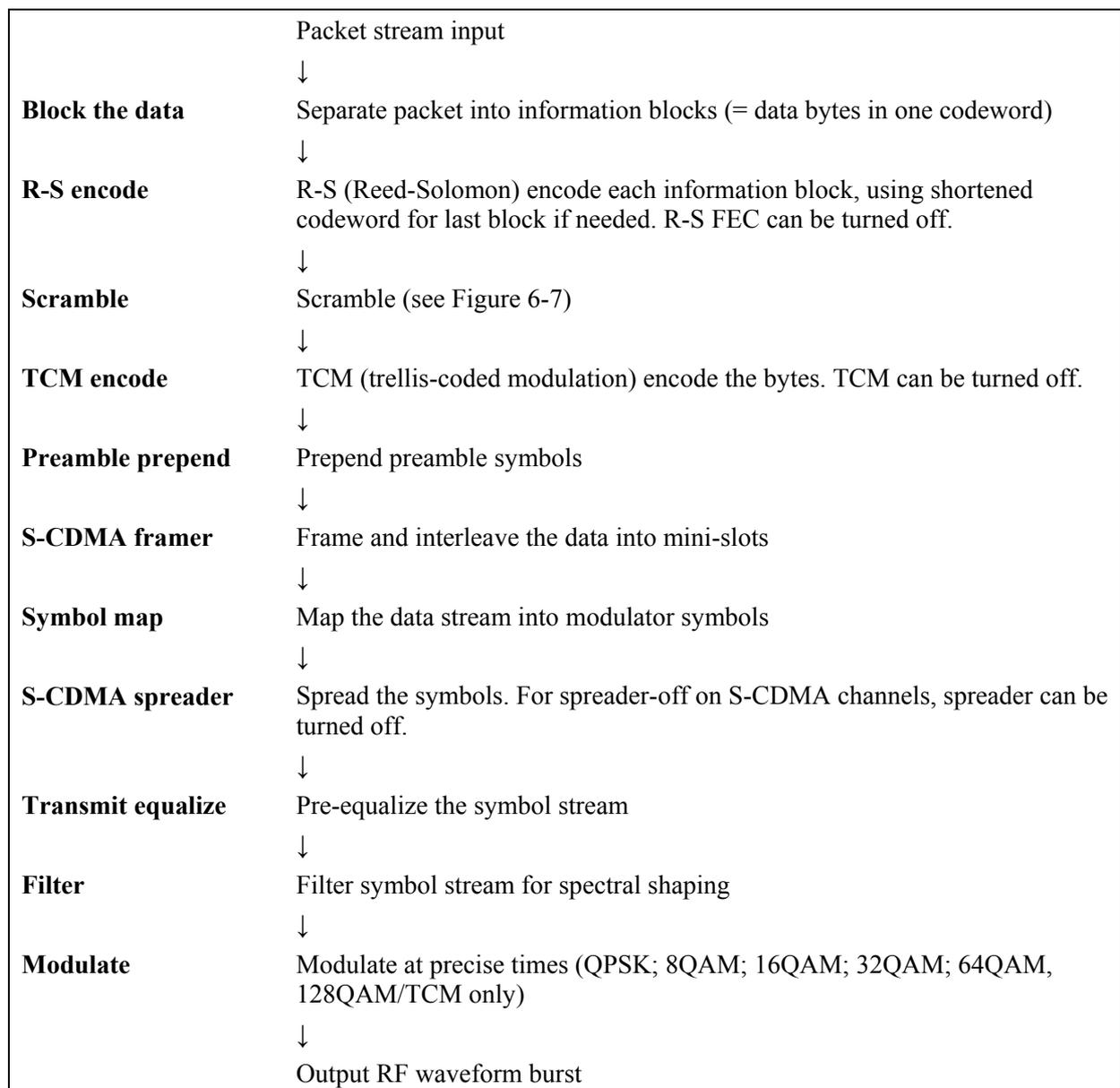
**Figure 6-3 – S-CDMA upstream transmission processing**
