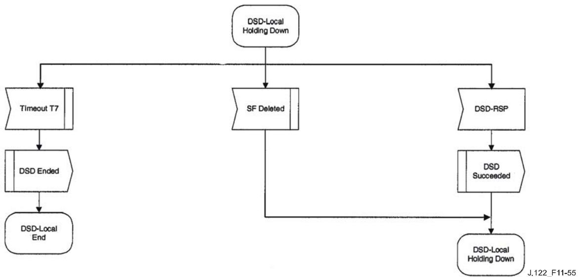
Figure 11-55 – DSD – Locally-initiated transaction holding down state flow diagram
