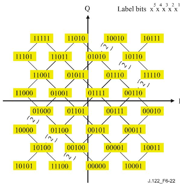
**Figure 6-22 – 32QAM symbol mapping**
