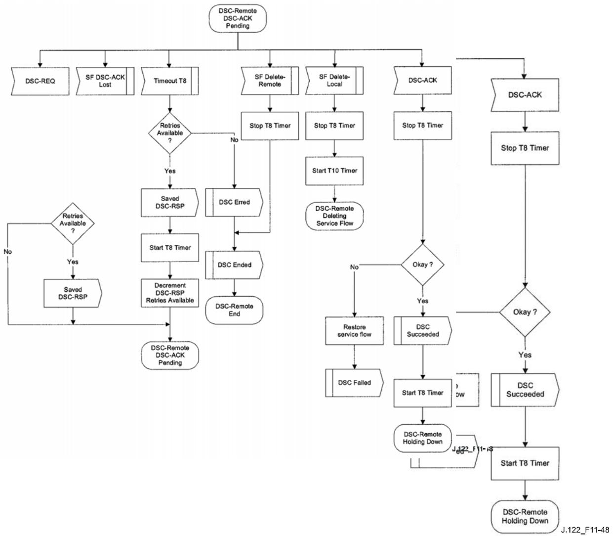
Figure 11-48 – DSC – Remotely-initiated transaction DSC-ACK pending state flow diagram
