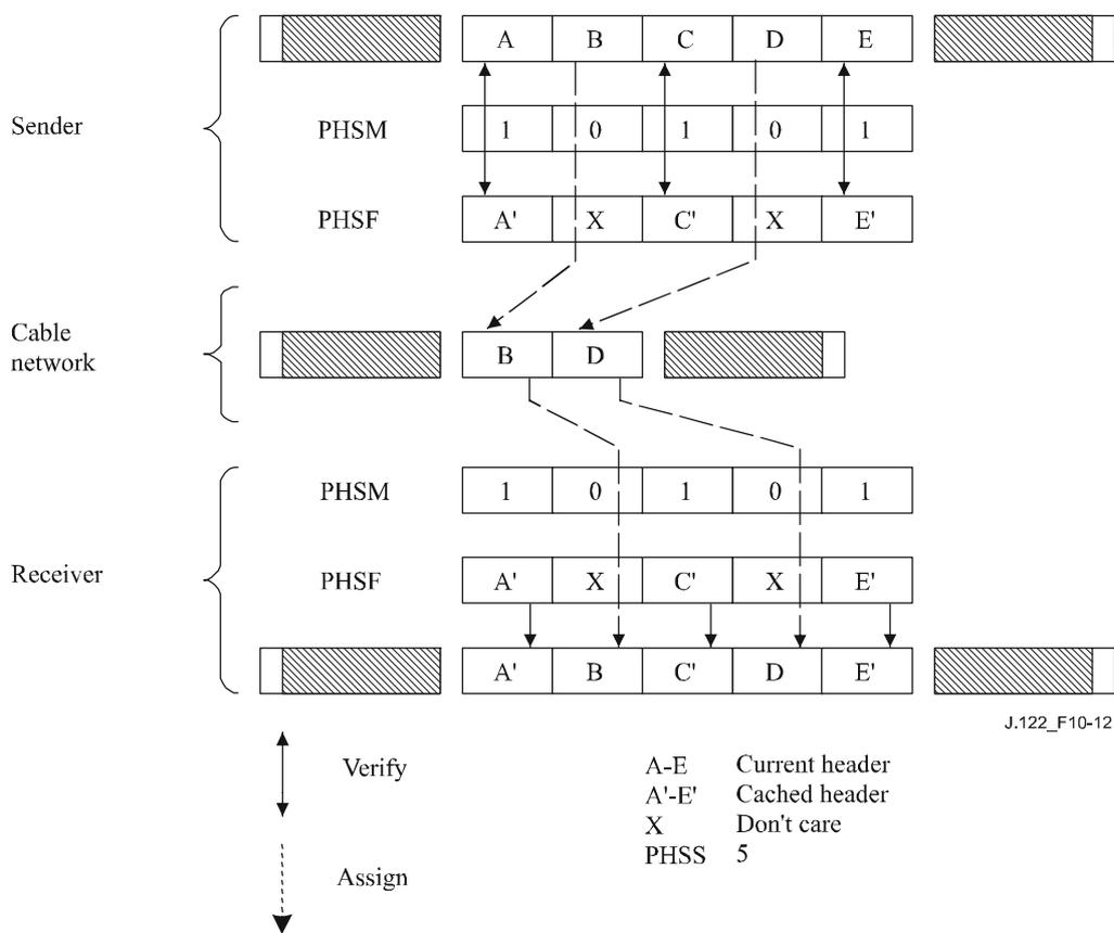
**Figure 10-12 – Payload header suppression with masking**
