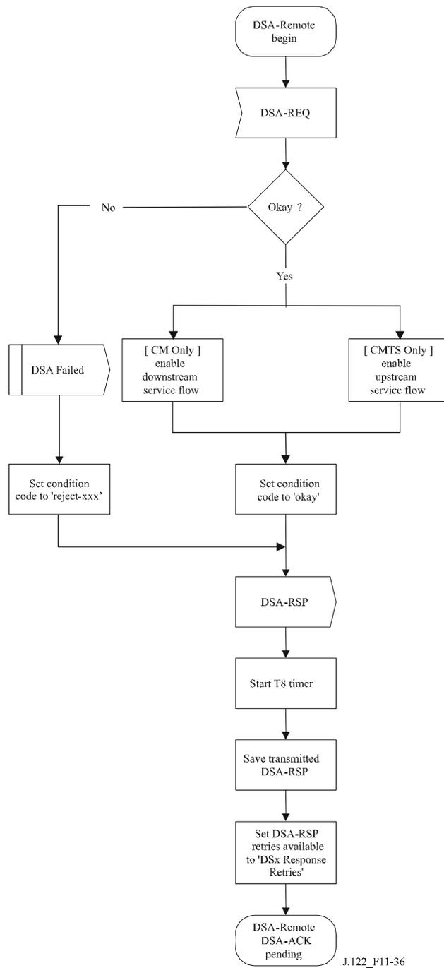
**Figure 11-36 – DSA – Remotely-initiated transaction begin state flow diagram**
