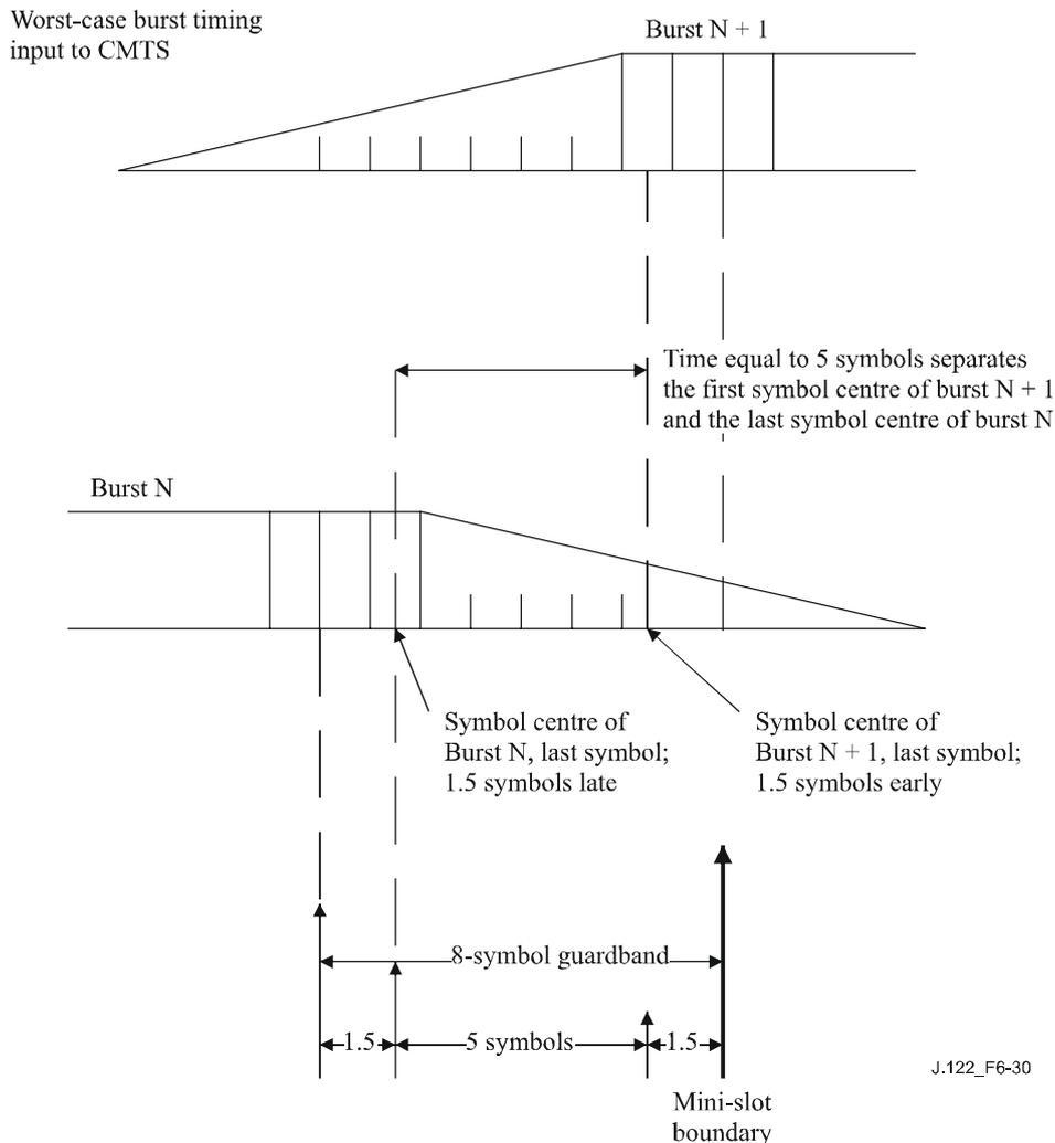
**Figure 6-30 – Worst-case TDMA burst timing**
