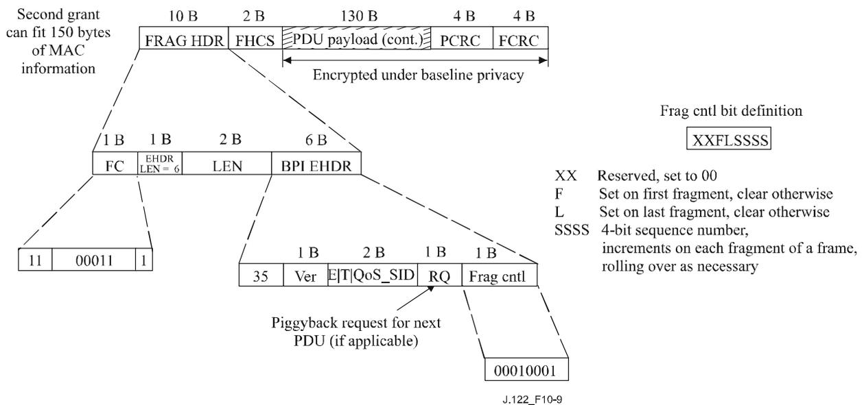
Figure 10-9 – Example of fragmenting a single packet
