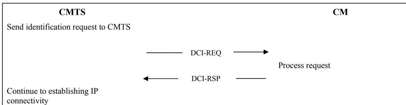
**Figure 11-9 – Device class identification**
