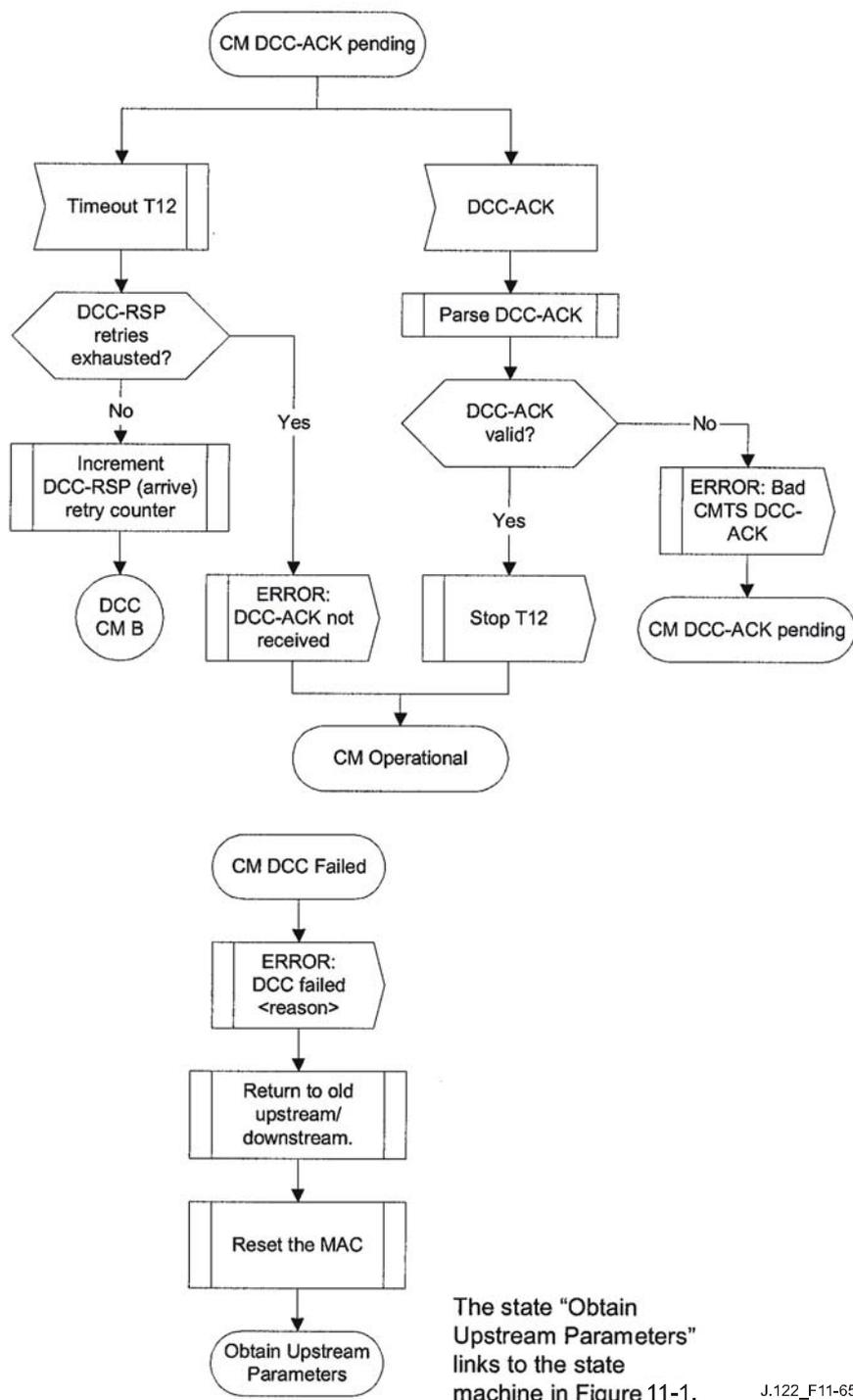
Figure 11-65 – Dynamically changing channels – CM view, part 4
