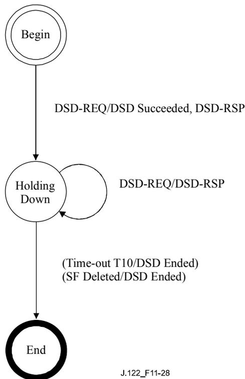
**Figure 11-28 – Dynamic deletion (DSD) – Remotely-initiated transaction state transition diagram**
