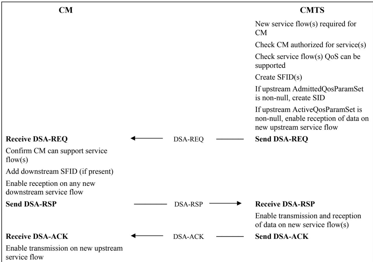
**Figure 11-30 – Dynamic service addition initiated from CMTS**
