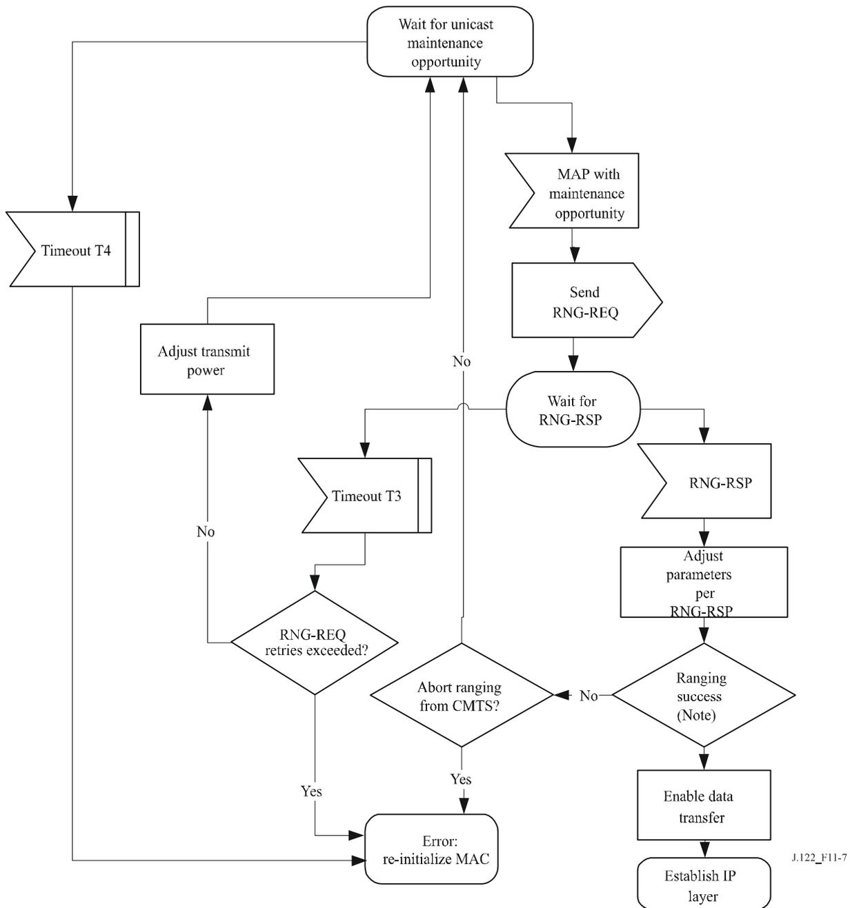
NOTE – Ranging request is within the tolerance of the CMTS.
