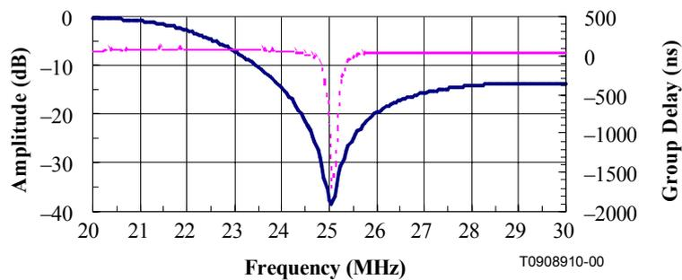
**Figure I.5/J.118 – Amplitude and group delay responses of the filter, case IV**
