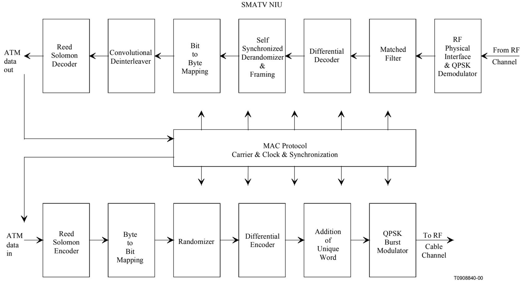
Figure 7/J.118 – Conceptual Block Diagram for the NIU OOB Transceiver
