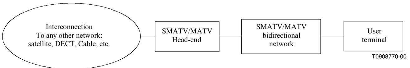
This Recommendation describes two different technological possibilities providing the specifications for the systems to be used in SMATV/MATV for interactive purposes.
