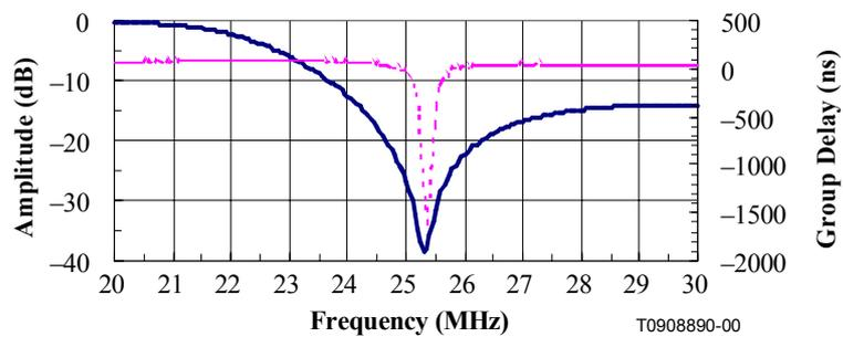
Figure I.3/J.118 – Amplitude and group delay responses of the filter, case II
