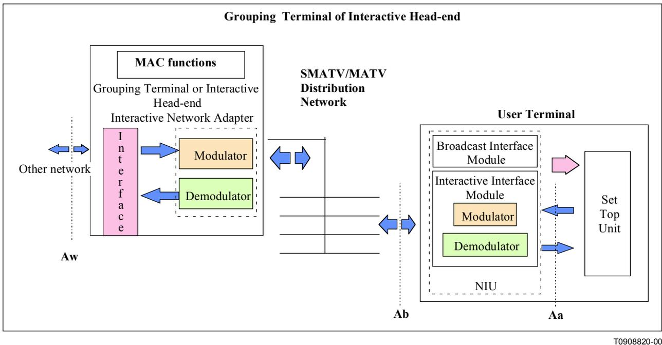
**Figure 5/J.118 – SMATV/MATV Coaxial Section Block diagram**
