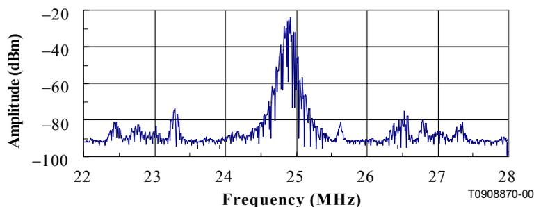
Figure I.1/J.118 – Power spectrum of the GMSK signal (Band 22-28 MHz)
