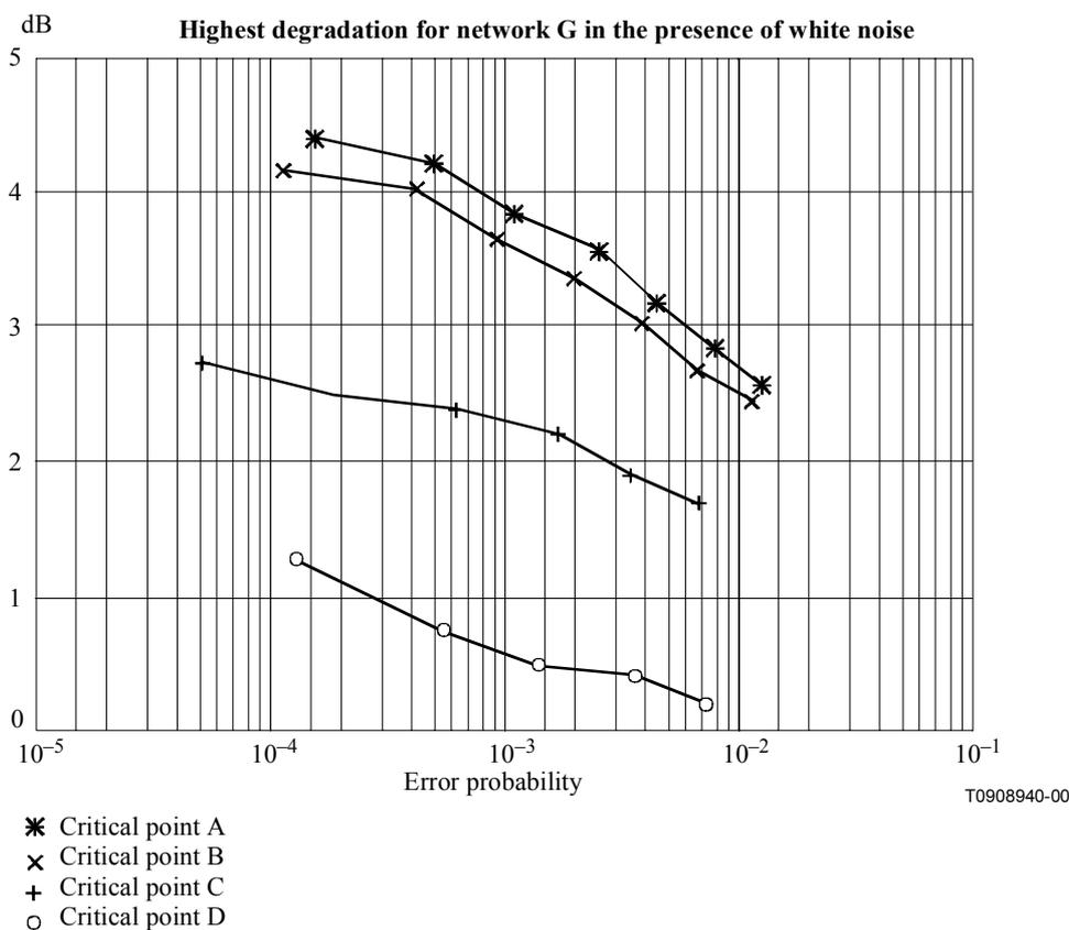
**Figure II.3/J.118 – Highest degradation in the presence of white noise due to the coaxial channel**
