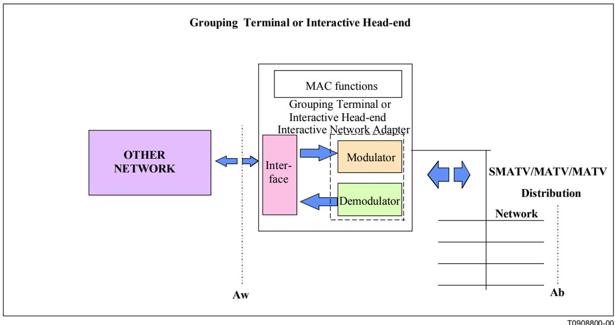
Figure 4a/J.118 – Functional block diagram for the SMATV/MATV Interactive Head-end
