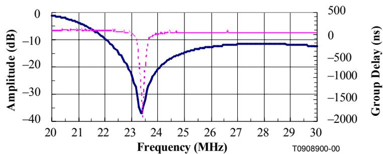
Figure I.4/J.118 – Amplitude and group delay responses of the filter, case III
