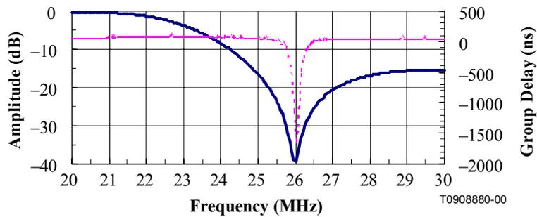
Figure I.2/J.118 – Amplitude and group delay responses of the filter, case I
