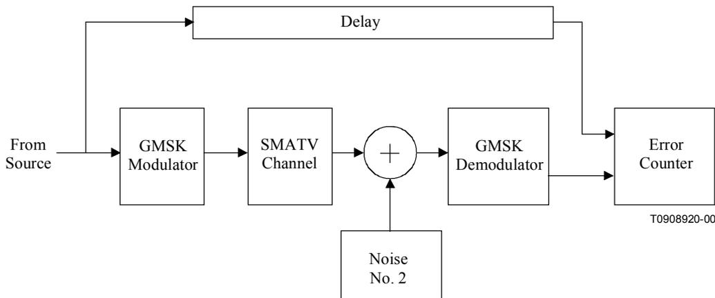
**Figure II.1/J.118 – Transmission chain adopted at the simulation**
