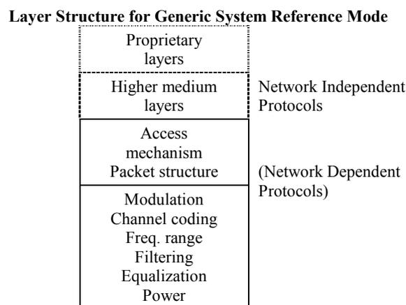
**Figure 1/J.118 – Layer Structure for Generic System Reference Model**
