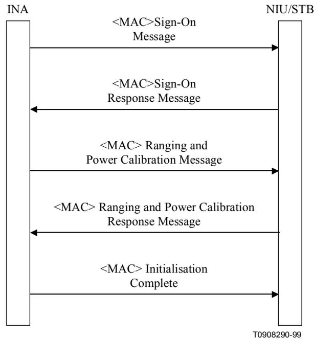
**Figure A.27/J.116 – Ranging and calibration signalling**
