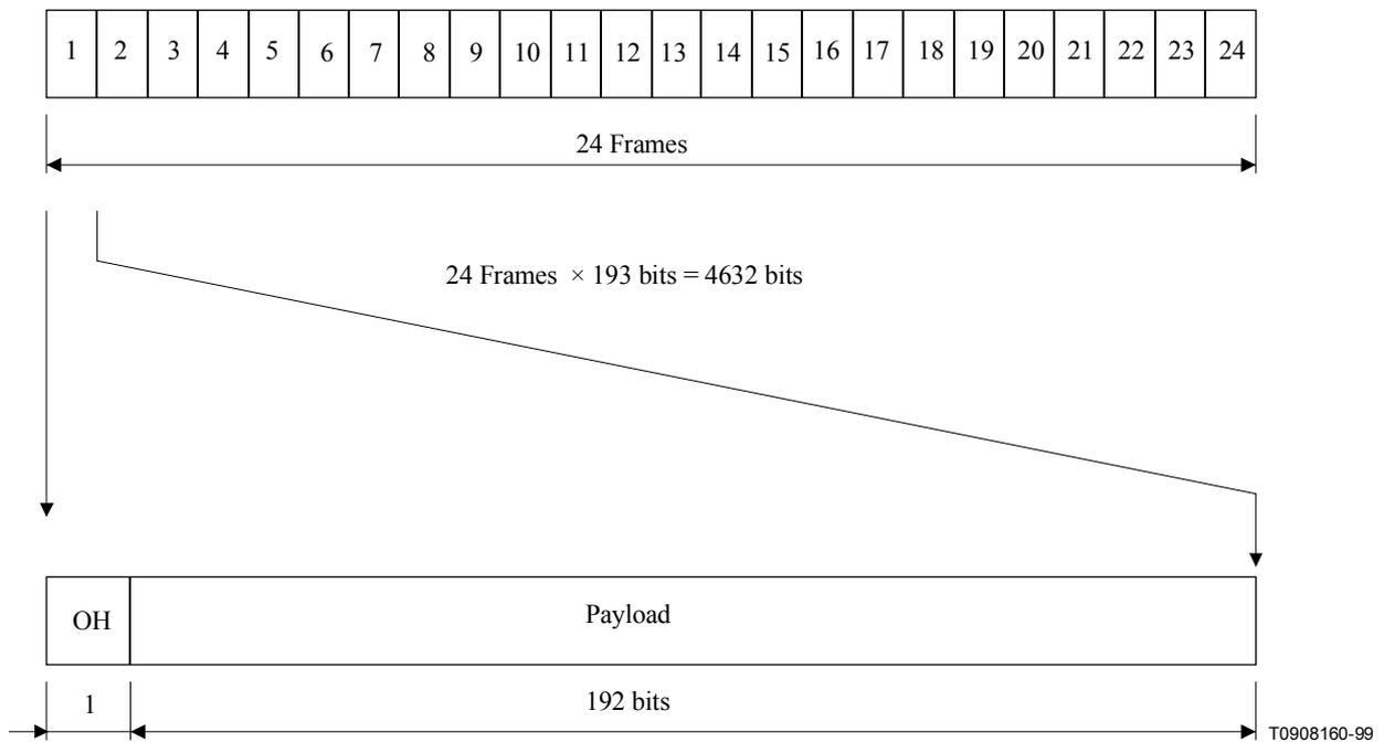
**Figure A.15/J.116 – SL-ESF frame structure**
