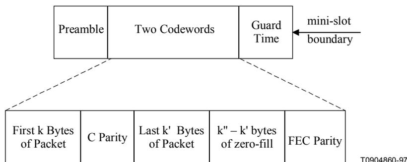
**Figure B.4-7/J.116 – Example frame structures with flexible burst length mode**
