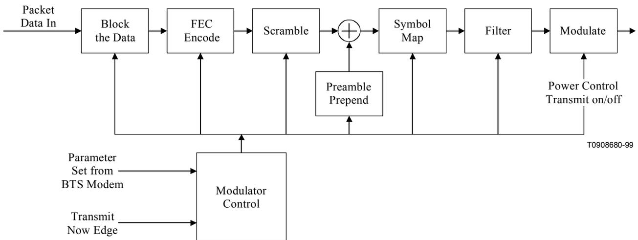
**Figure B.4-8/J.116 – Signal processing sequence**
