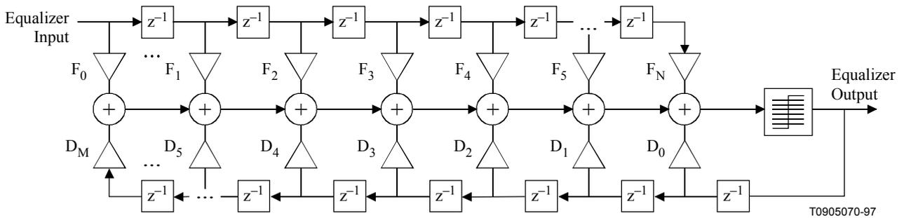
**Figure B.6-23/J.116 – BWA BTS Modem Demodulator Equaliser Tap Location Definition**
