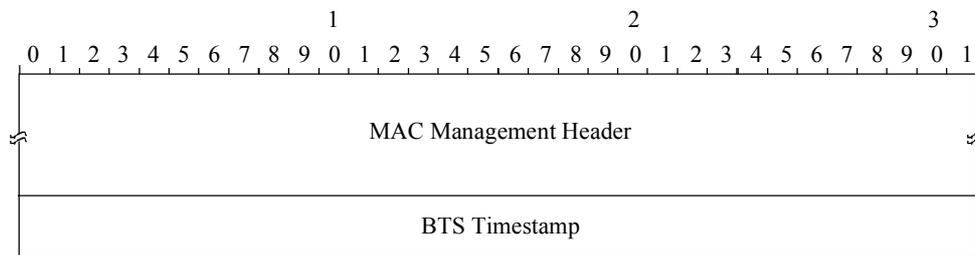
**Figure B.6-14/J.116 – Format of packet PDU following the timing header**
