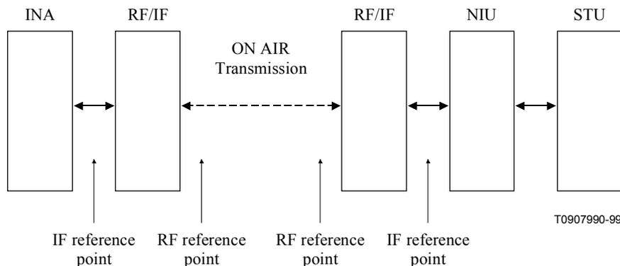
**Figure A.2b/J.116 – Position of IF and RF reference points in the particular case of LMDS networks**
