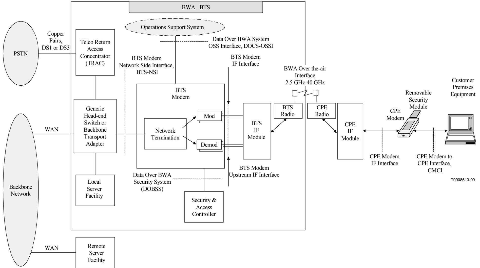
Figure B.1-2/J.116 – Data-over-BWA reference architecture
