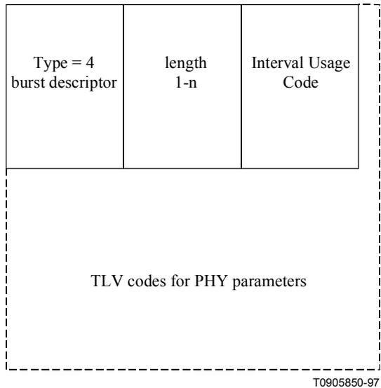
**Figure B.6-16/J.116 – Top-level encoding for a Burst Descriptor**
