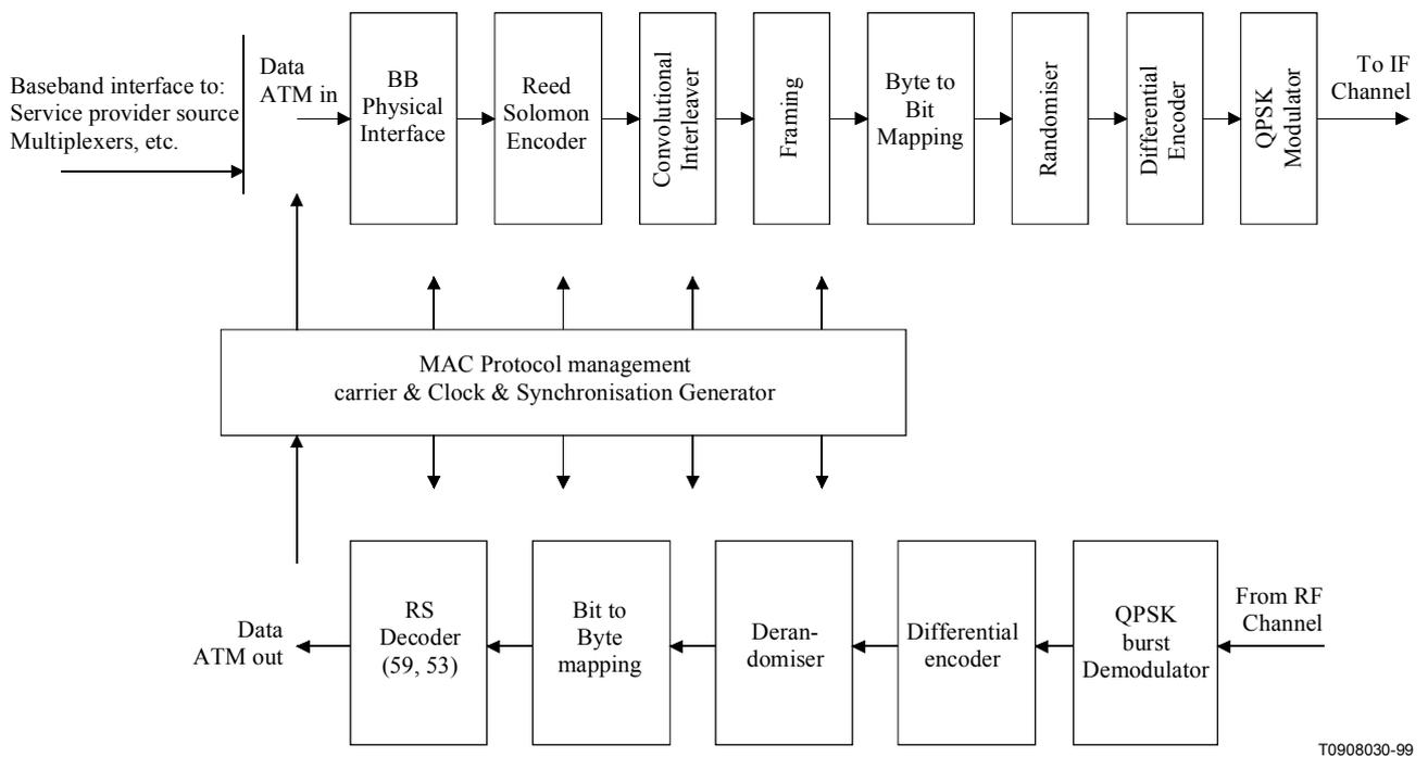
**Figure A.5/J.116 – Conceptual block diagram for the OOB head-end transceiver**
