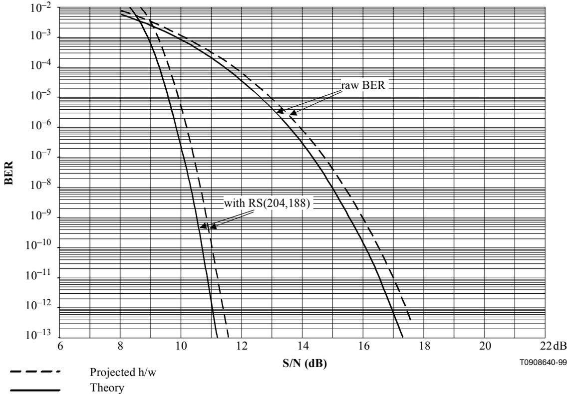
Figure B.2-3/J.116 – BER vs SNR Performance for QPSK (4-QAM)
