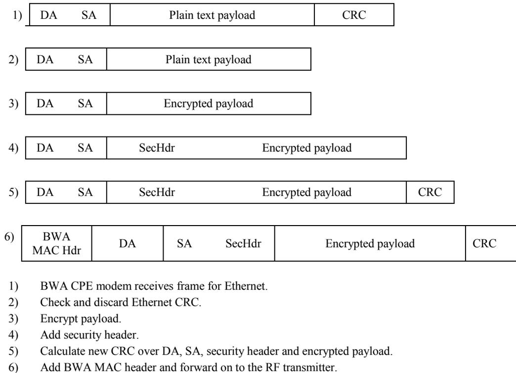
**Figure B.6-34/J.116 – Example of Security Framing at the BWA CPE modem**
