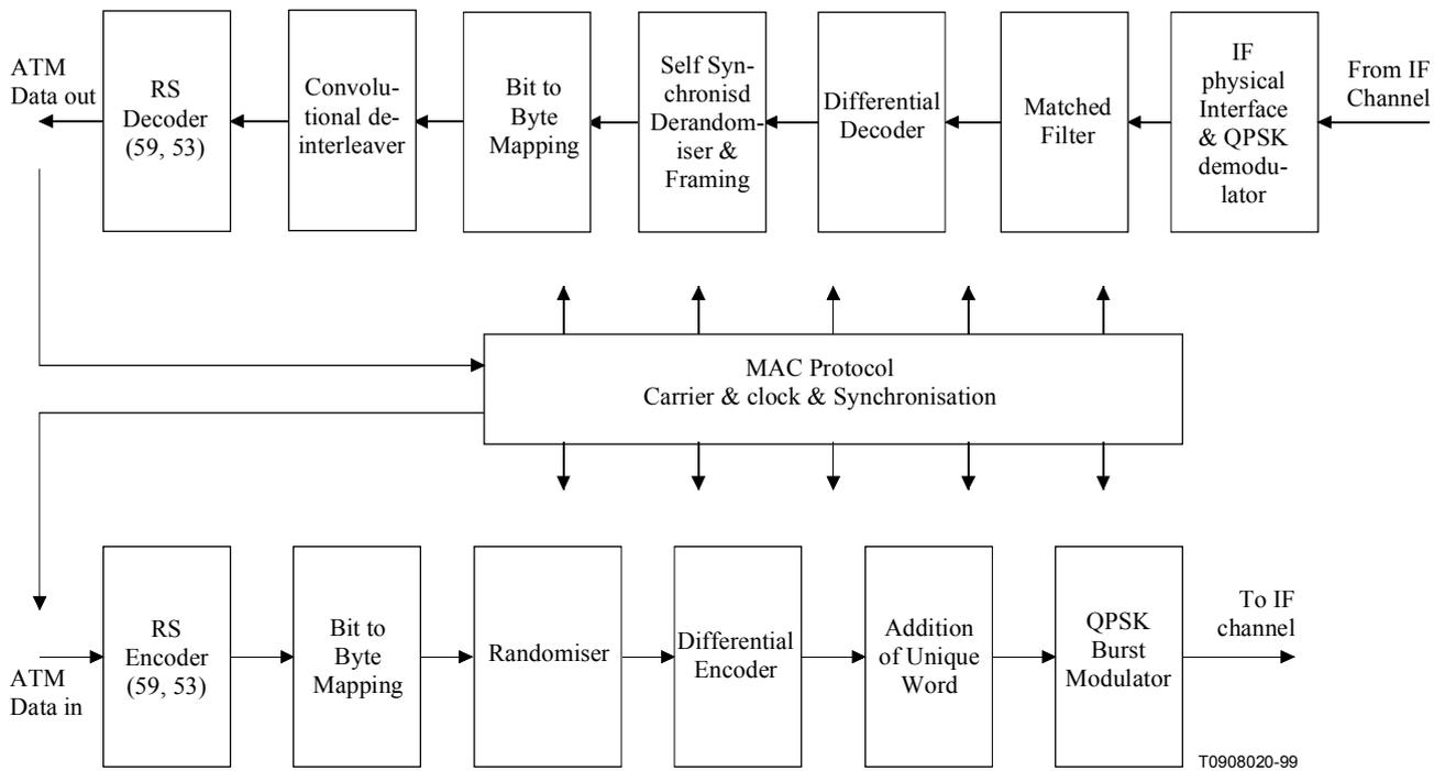
**Figure A.4/J.116 – Conceptual block diagram for the NIU OOB transceiver**
