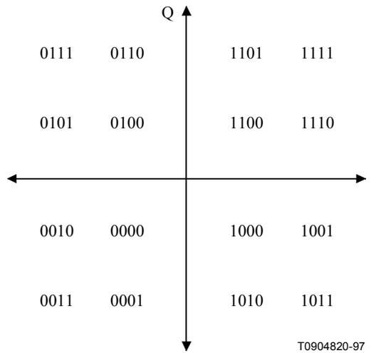
**Figure B.4-3/J.116 – 16-QAM Differential-Coded Symbol Mapping**
