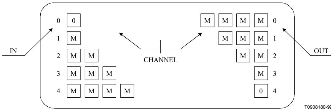
**Figure A.17/J.116 – Interleaver and de-interleaver structures**
