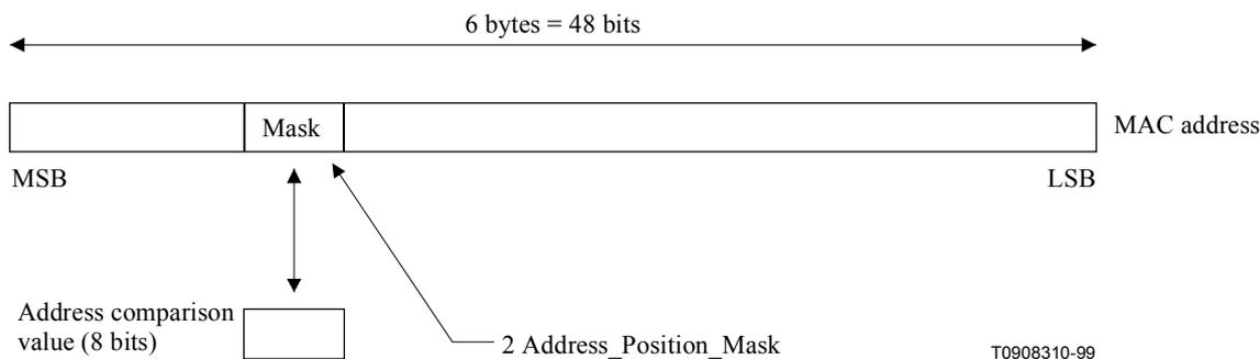
**Figure A.29/J.116 – Position of mask in MAC address**
