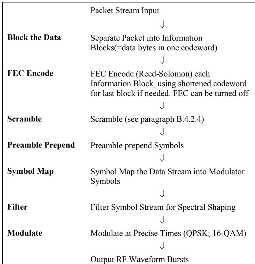
**Figure B.4-9/J.116 – TDMA upstream transmission processing**
