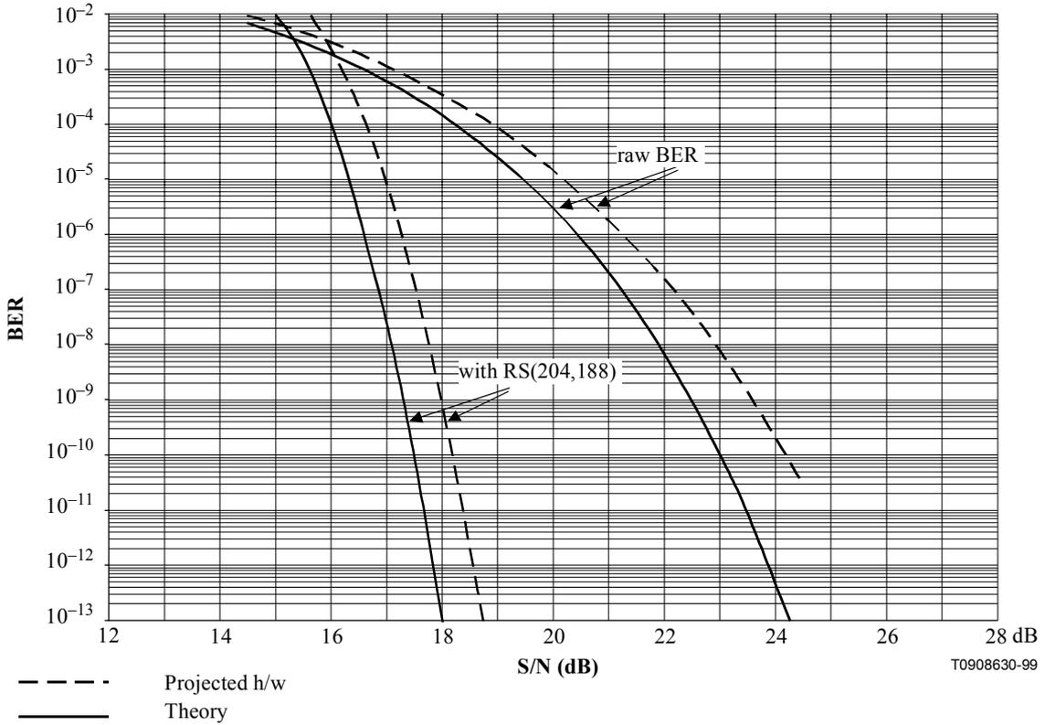
Figure B.2-2/J.116 – BER vs SNR Performance for 16-QAM
