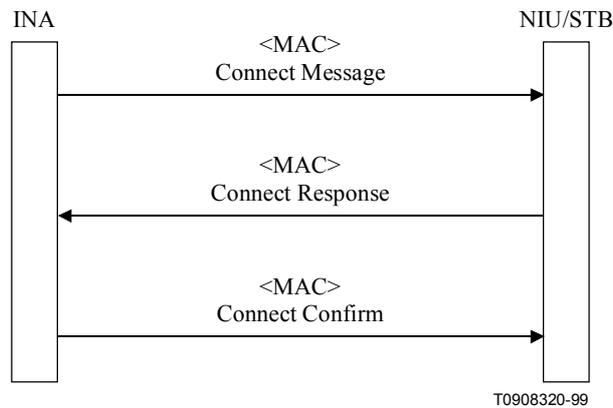
**Figure A.30/J.116 – Connection signalling**
