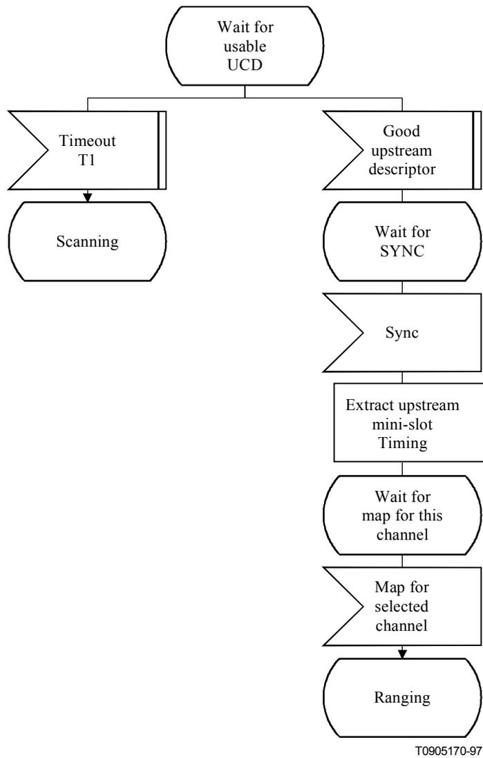
**Figure B.7-3/J.116 – Obtaining Upstream Parameters**
