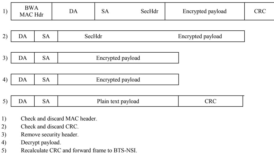
**Figure B.6-35/J.116 – Example of Security Framing at the BWA BTS**
