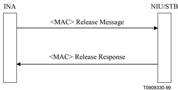
**Figure A.31/J.116 – Connection release signalling**
