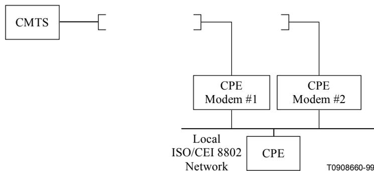
**Figure B.3-3/J.116 – Example condition for network loops**
