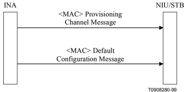
**Figure A.26/J.116 – Initialisation and provisioning signalling**
