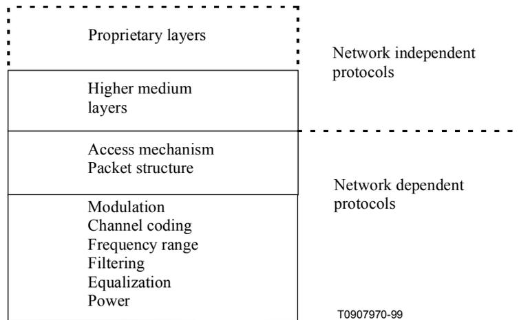
**Figure A.1/J.116 – Layer structure for generic system reference model**
