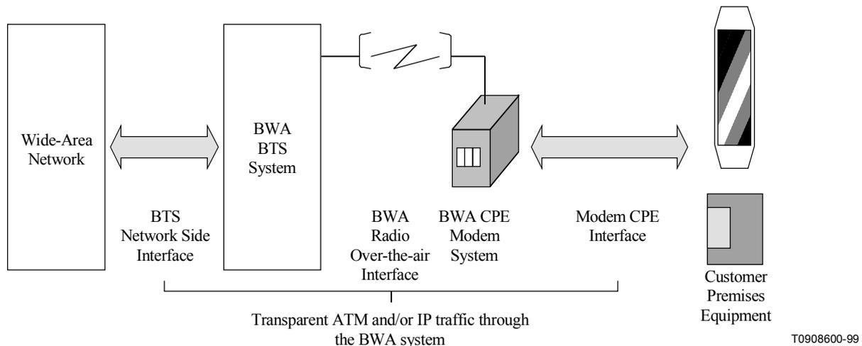
**Figure B.1-1/J.116 – Transparent ATM and/or IP traffic through the BWA system**
