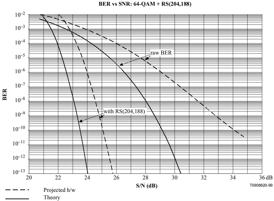
**Figure B.2-1/J.116 – BER vs SNR Performance for 64-QAM**
