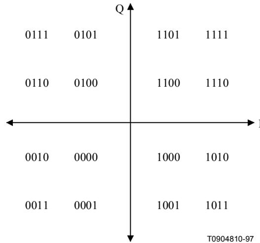
**Figure B.4-2/J.116 – 16-QAM Gray-Coded Symbol Mapping**
