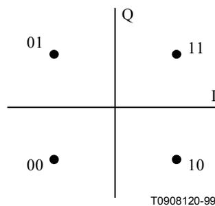
**Figure A.12/J.116 – Mapping for the QPSK constellation (upstream)**
