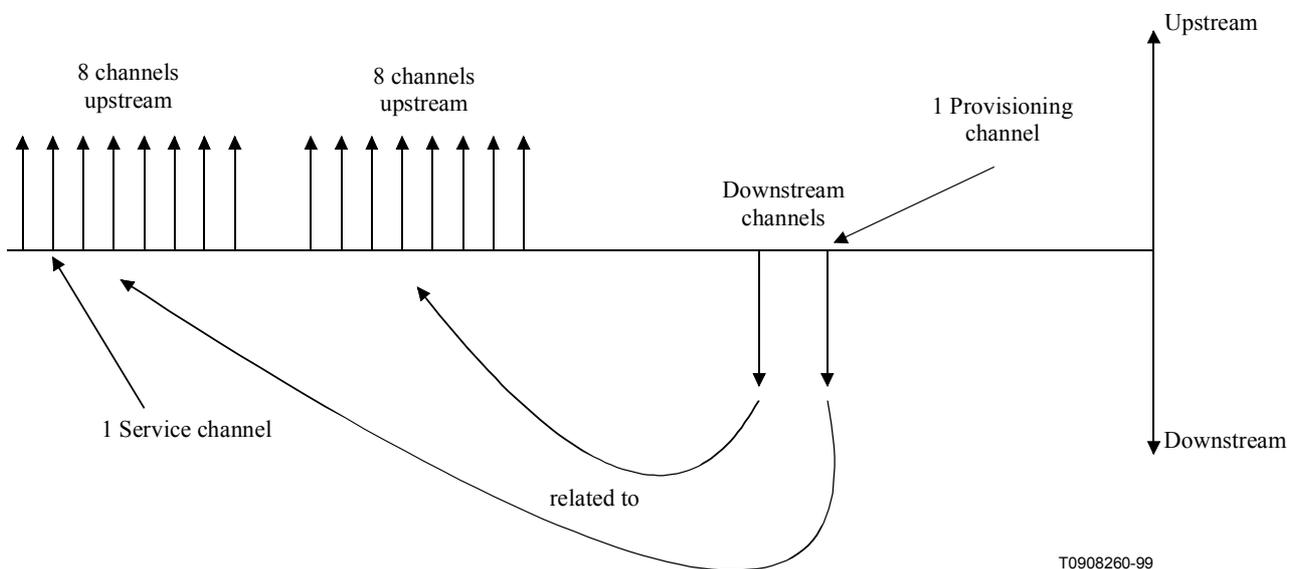
Figure A.24/J.116 – Example of frequency allocation
