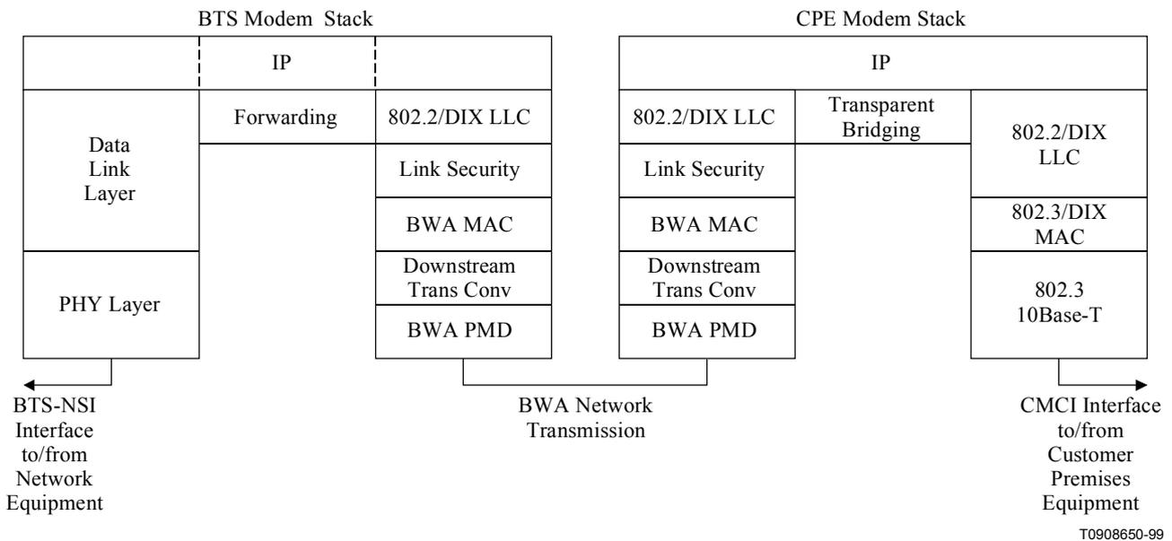
**Figure B.3-2/J.116 – Data forwarding through the BWA CPE Modem and the BWA BTS Modem**
