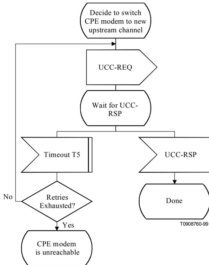
**Figure B.7-14/J.116 – Changing upstream channels: BWA BTS Modem View**
