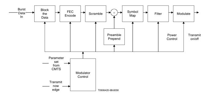
Figure B.4-8/J.112 – Signal-processing sequence
