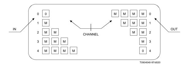
Figure A.19/J.112 - Interleaver and de-interleaver structures
