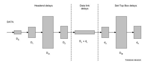
Figure A.24/J.112 – System model for timing analysis
