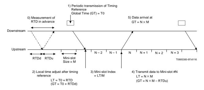
Figure C.6-3/J.112 – Global timing synchronization
