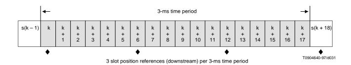
In the case where the downstream OOB rate is 3.088 Mbit/s, there are 6 slot position references downstream during the transmission of 18 upstream packets. In the case of IB downstream, packet "k" is sent when the 3-ms time marker is received.
