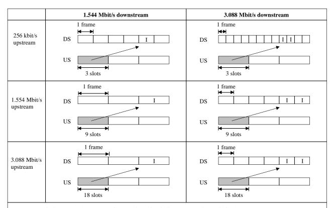
NOTE 1-T indicates the downstream frame(s) in which indicators (contained within the MAC Flag Sets) are sent. These indicators control the upstream slots in the shaded area.
