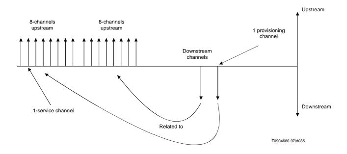
Figure A.26/J.112 – Example of frequency allocation
