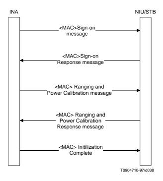
Figure A.29/J.112 – Ranging and calibration signalling
