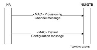
$Figure \ A. 28/J. 112-Initialization \ and \ Provisioning \ signalling$
