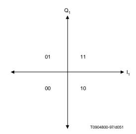
Figure B.4-1/J.112 – QPSK symbol mapping
