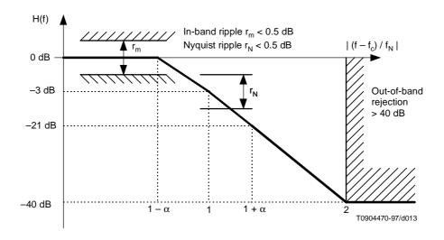
Figure A.14/J.112 – QPSK upstream transmitter Power Spectrum
