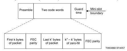
Figure B.4-7/J.112 – Example frame structures with flexible burst length mode
