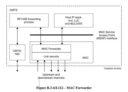
In Figure B.3-4, the LLC sublayer and link security sublayers of the upstream and downstream channels on the cable network terminate at the MAC Forwarder.
