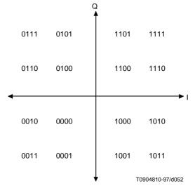
Figure B.4-2/J.112 – 16 QAM Gray-coded symbol mapping
