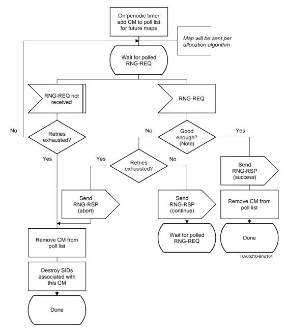
NOTE – Means Ranging Request is within the tolerance limits of the CMTS for power and transmit equalization (if supported).
