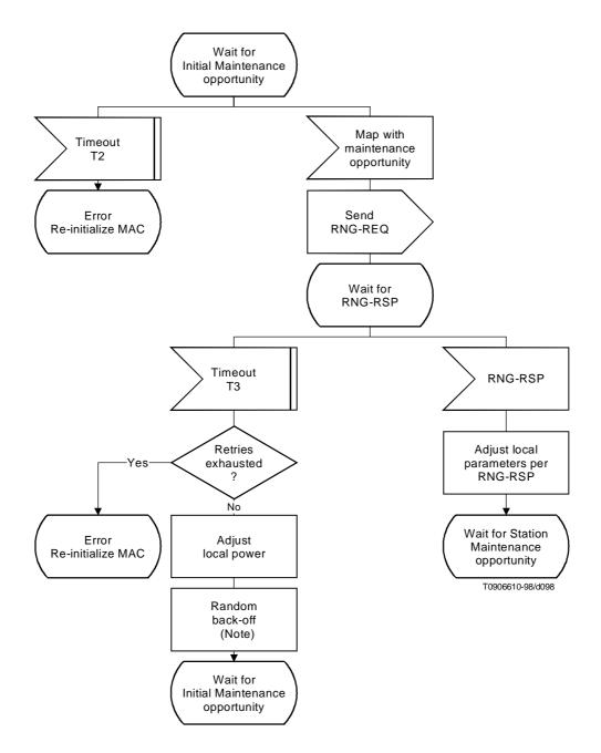
NOTE – Timeout T3 may occur because the RNG-REQs from multiple modems collided. To avoid these modems repeating the loop in lockstep, a random back-off is required. This is a back-off over the ranging window specified in the MAP.
