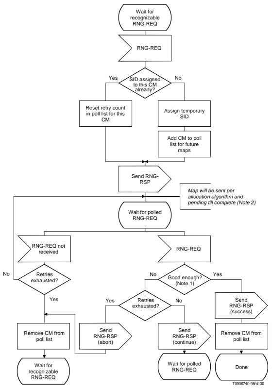
NOTE 1 – Means ranging is within the tolerable limits of the CMTS.
