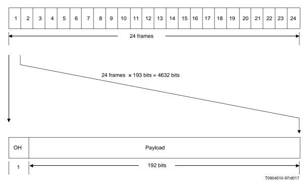
Figure A.17/J.112 – SL-ESF frame structure
