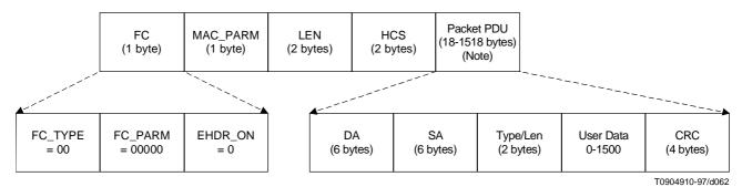
NOTE – Frame size is limited to 1518 bytes in the absence of VLAN tagging. Cooperating devices which implement IEEE 802.1Q VLAN tagging MAY use a frame size up to 1522 bytes.
