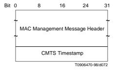
Figure B.6-14/J.112 – Format of Packet PDU following the timing Header
