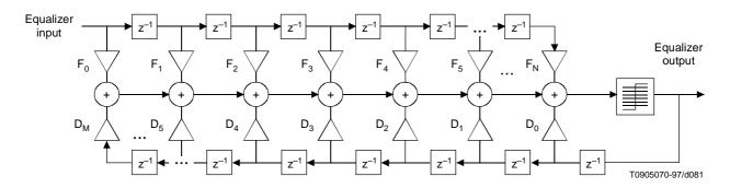
Figure B.6-23/J.112 - CMTS demodulator equalizer tap location definition
