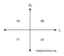
Figure C.4-1/J.112 – QPSK Signal Constellation Diagram
