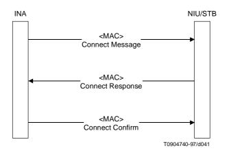
Figure A.32/J.112 – Connection signalling
