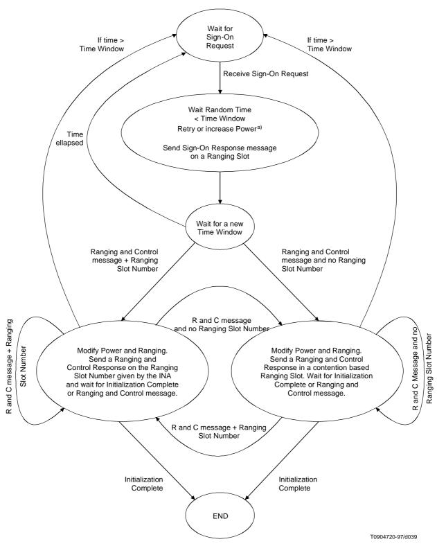
a) "Retry or Increase Power" means that the NIU should retry with the same power Sign\_On\_Incr\_Pwr\_Retry\_Count times (given by the <MAC> defaut configuration message) and then increase the power by 0.5 dB.
