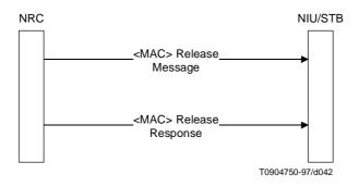
Figure A.33/J.112 – Connection release signalling
