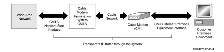
Figure B.1-1/J.112 – Transparent IP traffic through the data-over-cable system
