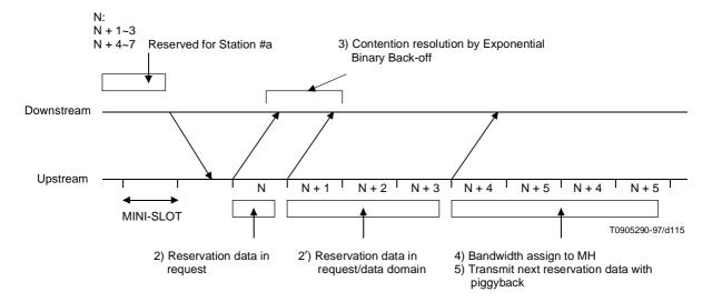
Figure C.6-2/J.112 - Bandwidth assignment by mini-slot and message
