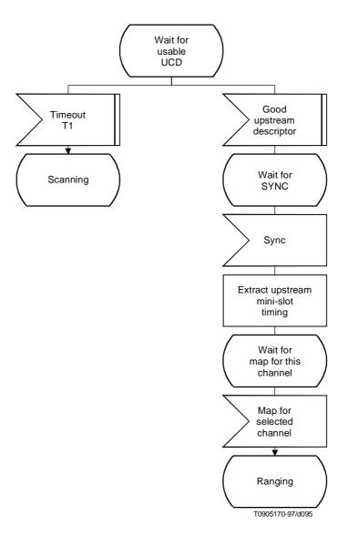
Figure B.7-3/J.112 – Obtaining upstream parameters
