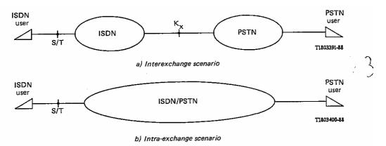
Note 1 - In part a) refer to Rec. I.324 for the definition of  $K_x$  reference point. Note 2 - Part b) illustrates the case where no clear division exists between ISDN and PSTN network components.
