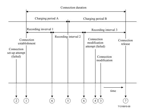
Figure 2/I.377 – Moments in time at which registration shall be performed – the numbers correspond with the bullet numbers in the text
