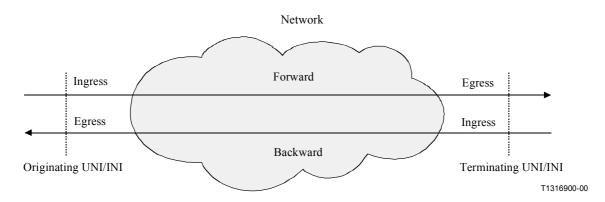
Figure 1/I.377 – Illustration of the terminology originating/terminating UNI, forward/backward direction and ingress/egress sides of one network
