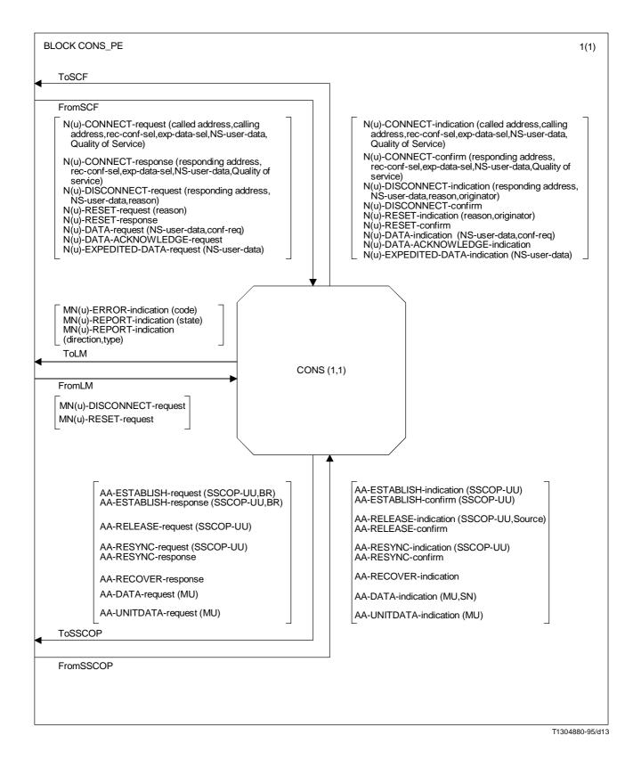
FIGURE 12/I.365.2 Block SSCF-CONS SDL diagram
