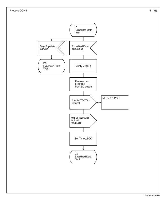
FIGURE C.3/I.365.2 (sheet 2 of 7) **Procedure SSCF-CONS – Service Expedited Data SDL diagram**
