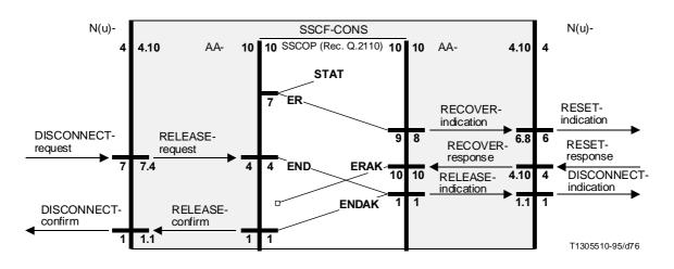
FIGURE 1.25/1.365.2 Sequences for a provider initiated reset of an N(u)-connection followed immediately by a release
