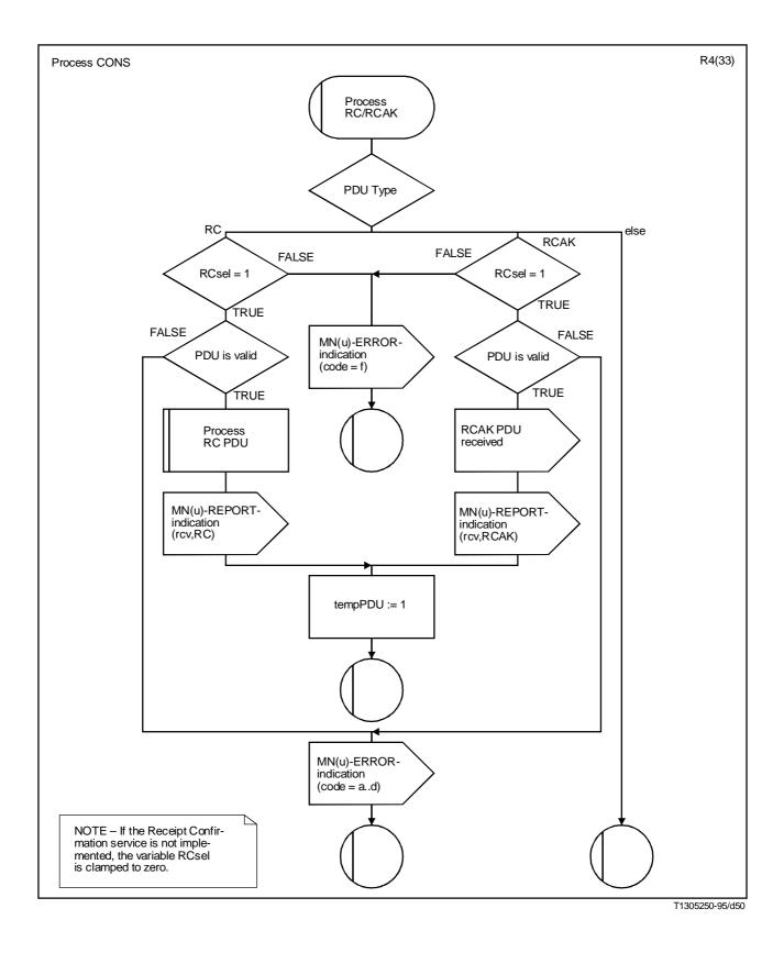
FIGURE D.3/I.365.2 (sheet 5 of 5) **Procedure SSCF-CONS – Service Receipt Confirmation SDL diagram**
