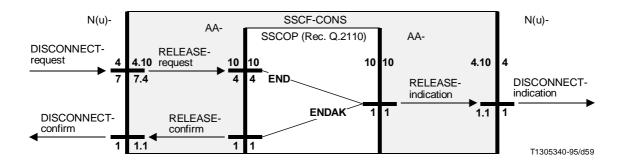
FIGURE I.8/I.365.2 Sequences for releasing an N(u)-connection
