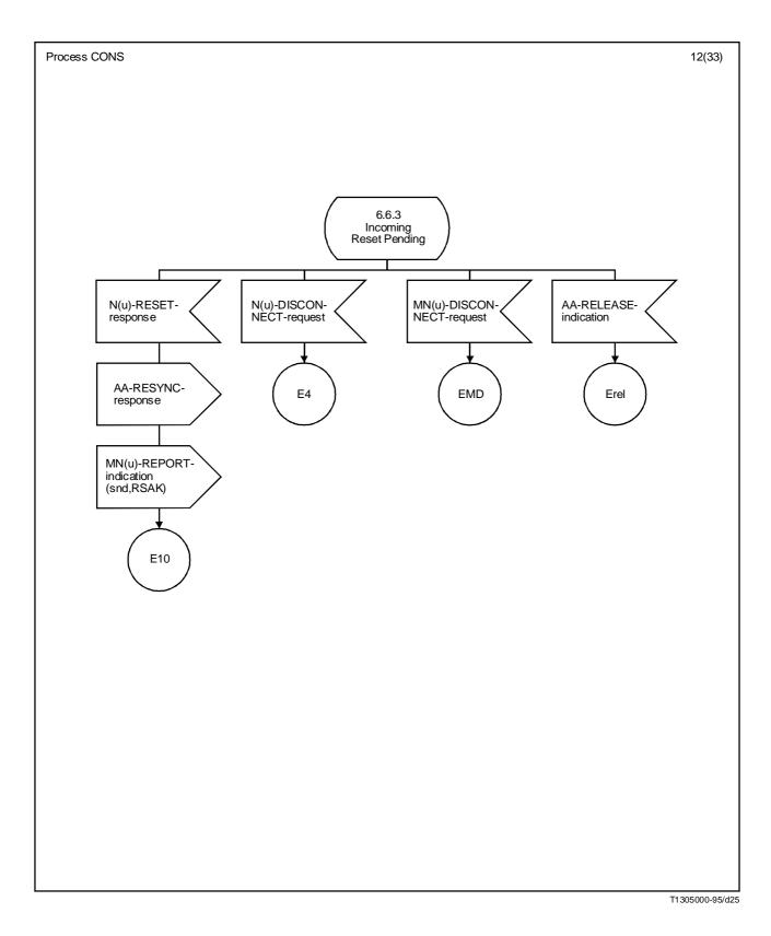
FIGURE 13/I.365.2 (sheet 12 of 21) Procedure SSCF-CONS-Main Service SDL diagram
