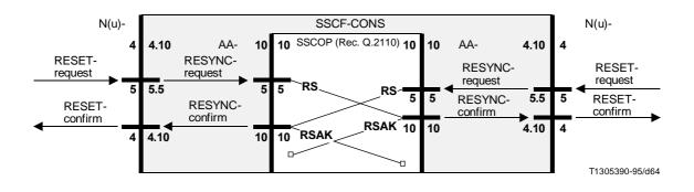
FIGURE I.13/I.365.2 Sequences for resetting an N(u)-connection with collision
