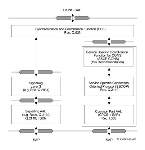
FIGURE 2a/I.365.2 Structure of the CONS provider deploying switched ATM connections
