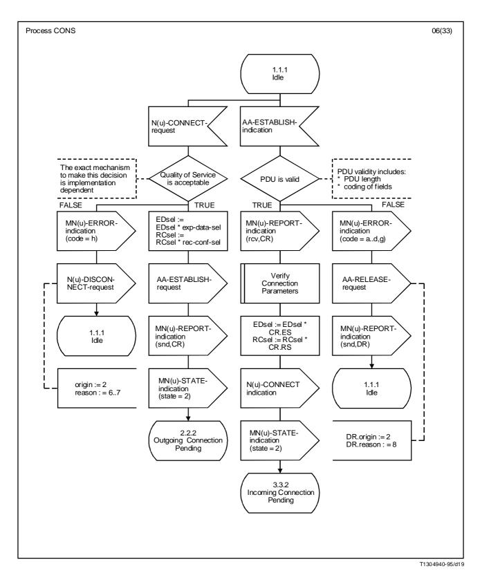
FIGURE 13/I.365.2 (sheet 6 of 21) Procedure SSCF-CONS-Main Service SDL diagram
