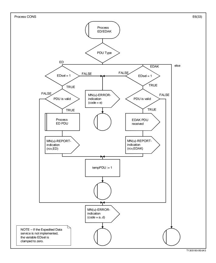
FIGURE C.3/I.365.2 (sheet 7 of 7) **Procedure SSCF-CONS – Service Expedited Data SDL diagram**
