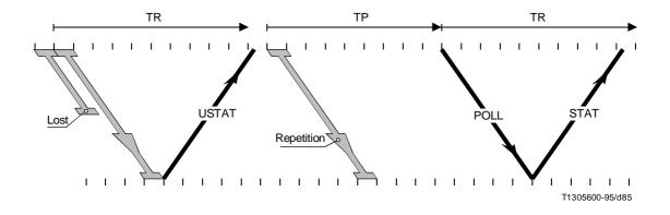
FIGURE II.3/I.365.2 Timing for single error correction (DATA PDU)
