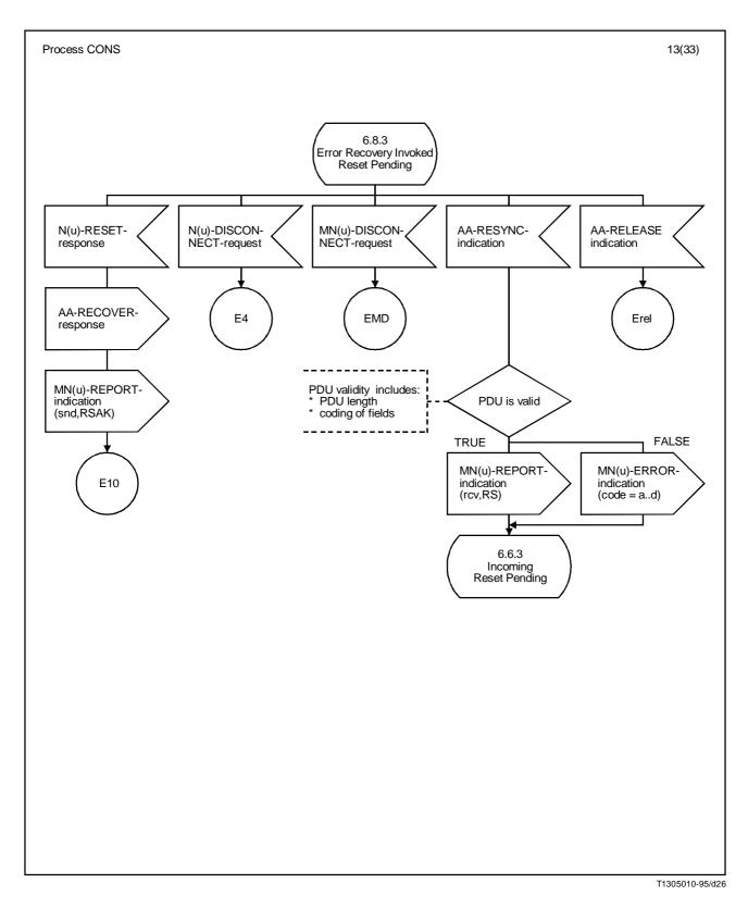
FIGURE 13/I.365.2 (sheet 13 of 21) Procedure SSCF-CONS-Main Service SDL diagram
