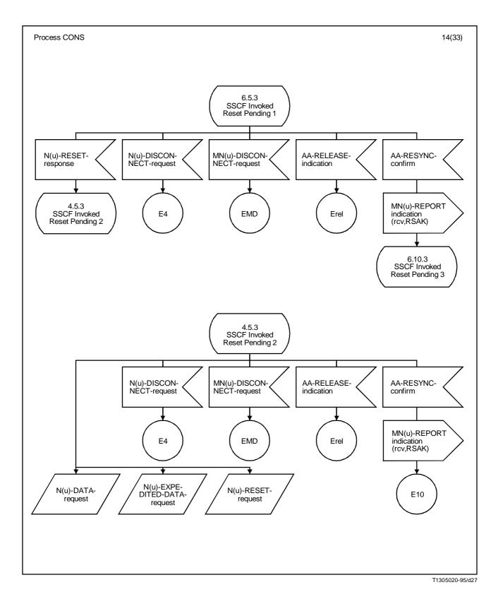
FIGURE 13/I.365.2 (sheet 14 of 21) Procedure SSCF-CONS-Main Service SDL diagram
