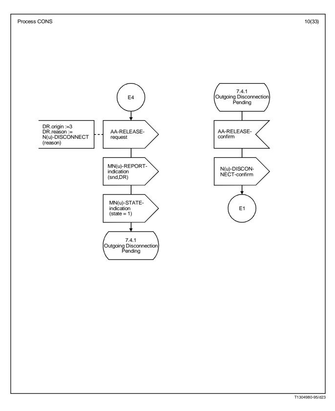
FIGURE 13/I.365.2 (sheet 10 of 21) Procedure SSCF-CONS-Main Service SDL diagram
