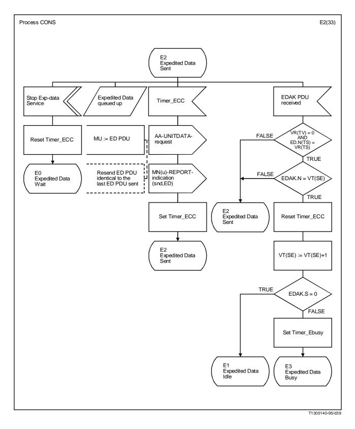
FIGURE C.3/I.365.2 (sheet 3 of 7) **Procedure SSCF-CONS – Service Expedited Data SDL diagram**
