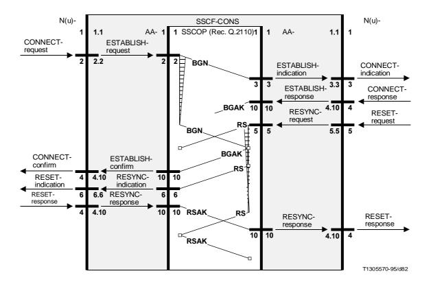
FIGURE 1.31/1.365.2 Sequences for establishing an N(u)-connection with corruption followed by a user invoked reset
