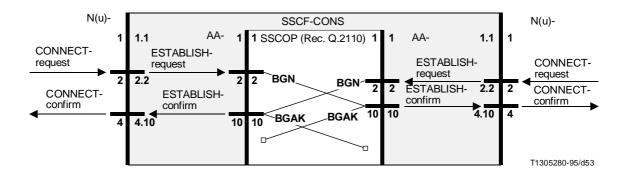
FIGURE 1.2/I.365.2 Sequences for establishing an N(u)-connection with collision
