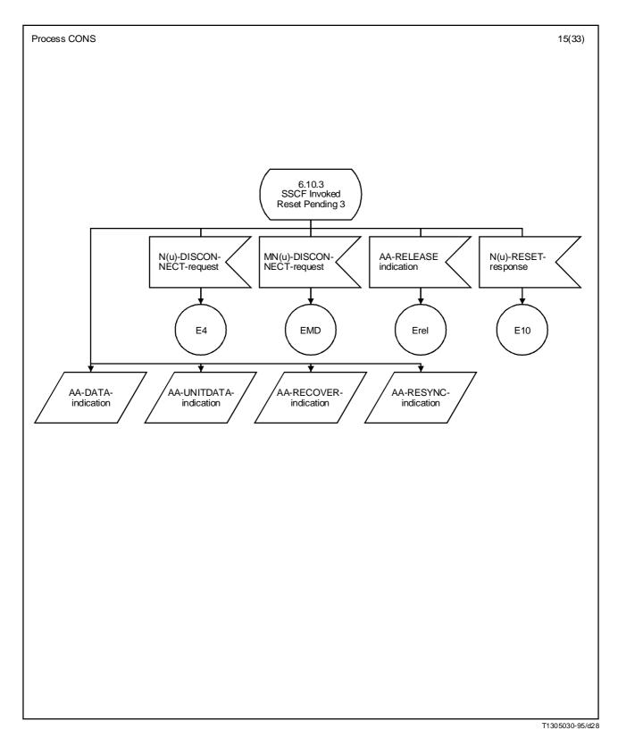
FIGURE 13/I.365.2 (sheet 15 of 21) Procedure SSCF-CONS-Main Service SDL diagram
