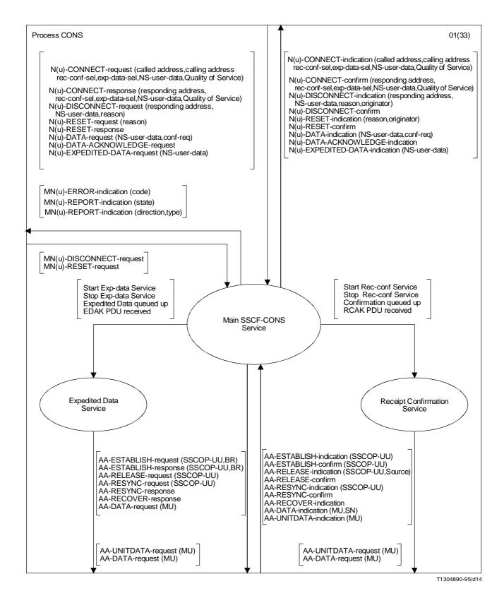
FIGURE 13/I.365.2 (sheet 1 of 21) Procedure SSCF-CONS-Main Service SDL diagram
