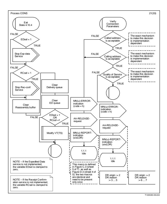
FIGURE 13/I.365.2 (sheet 21 of 21) Procedure SSCF-CONS-Main Service SDL diagram
