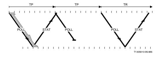
FIGURE II.4/I.365.2 Timing for single error correction (POLL PDU)
