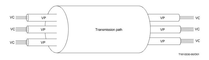
FIGURE 2/I.311 Relationship between the VC, the VP and the transmission path
