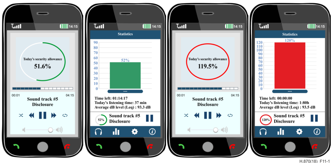
Figure 11-1 – Examples of information provided on a smartphone visual interface for safe listening
