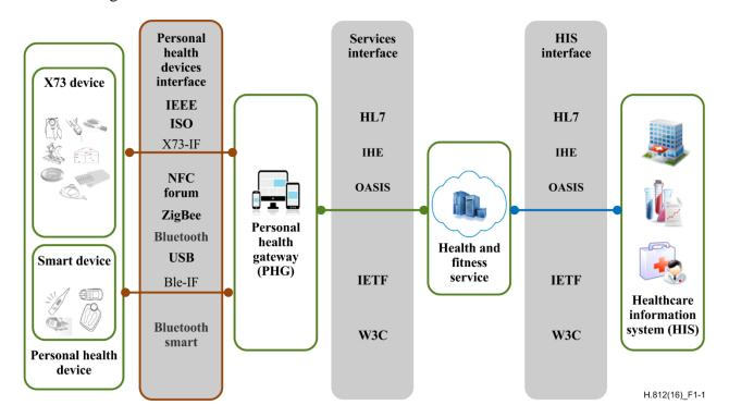
Figure 1-1 – Services interface in the Continua architecture
