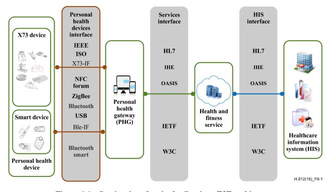
Figure 6-1 – Services interface in the Continua E2E architecture
