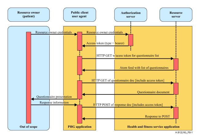
Figure 8-2 – Security behaviour for authorized RESTful CCC behaviour (Questionnaire use case is taken as an example)
