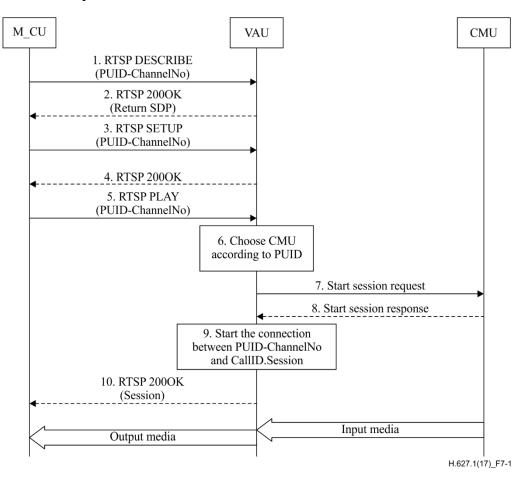
Figure 7-1 – High level procedural flows for real-time media acquisition
