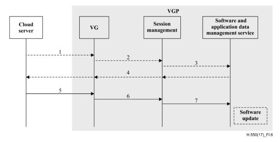
Figure I.6 – Signalling flows of the remote software update scenario
