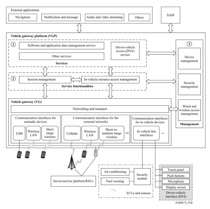
Figure 2 – High-level architecture of a VGP
