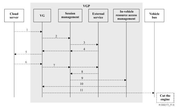
**Figure I.5 – Signalling flows of the anti-stolen scenario**
