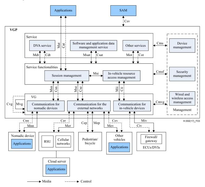
Figure 3 – Functional architecture framework of VGP
