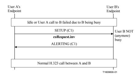
Figure 4/H.450.10 – Example message flow for SS-CO request if user B is not busy – direct routed signalling
