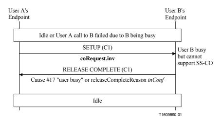
Figure 3/H.450.10 – Example message flow for unsuccessful SS-CO request – direct routed signalling
