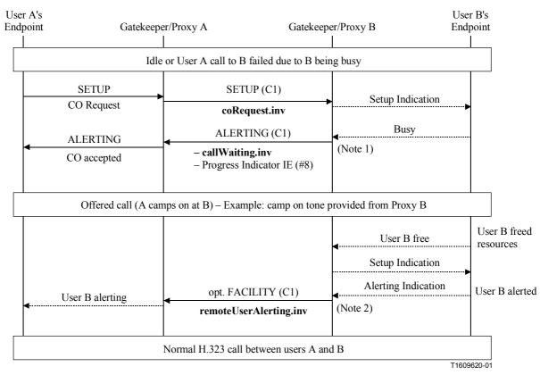
NOTE 1 – The GK/Proxy B acts on behalf of endpoint B for SS-CO upon busy detection. How the GK/proxy B detects that User B is busy depends on implementation and on the terminal protocol.
