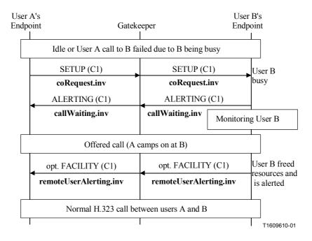
Figure 5/H.450.10 – Example message flow for successful SS-CO – gatekeeper being transparent for SS-CO signalling
