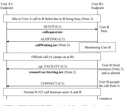
NOTE 1 – RELEASE COMPLETE received with Cause #17 *user busy* or with releaseCompleteReason *inConf.* NOTE 2 – For SS-CO, callWaiting.inv (as defined in ITU-T H.450.6) may also be sent in a PROGRESS message (e.g. if interworking requires). In such a case, an ALERTING message (without SS-CO APDU) will be sent instead of FACILITY with remoteUserAlerting.inv. NOTE 3 – E.g. by releasing another call or by putting another call on hold.
