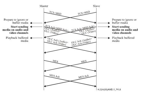
Figure K.8/H.324 – Accelerated H.245 procedures for both audio and video channels
