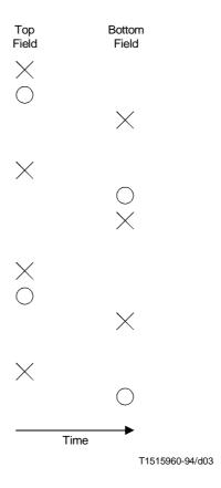
Figure 6-2 – Vertical and temporal positions of samples in an interlaced frame with top\_field\_first = 1
