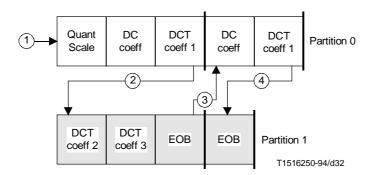
Figure 7-17 – A segment from a bitstream with two partitions, with priority\_breakpoint set to 64 (one (run, level) pair). The two partitions are shown, with arrows indicating how the decoder needs to switch between partitions
