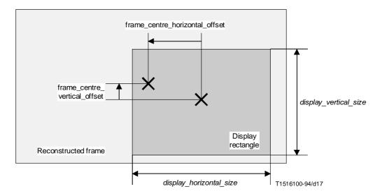
Figure 6-16 – Frame centre offset parameters
