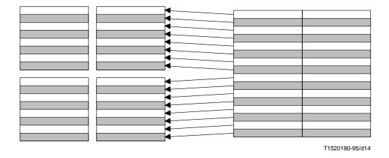
Figure 6-13 – Luminance macroblock structure in frame DCT coding
