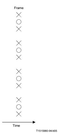
Figure 6-4 – Vertical and temporal positions of samples in a progressive frame
