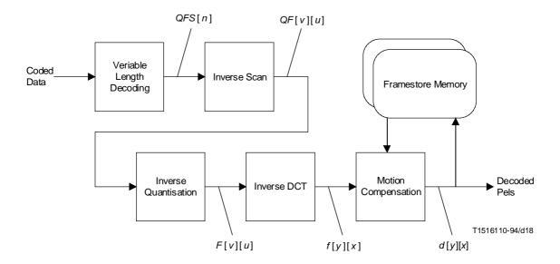
Figure 7-1 – Simplified Video Decoding Process
