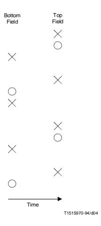
Figure 6-3 – Vertical and temporal positions of samples in an interlaced frame with top\_field\_first = 0
