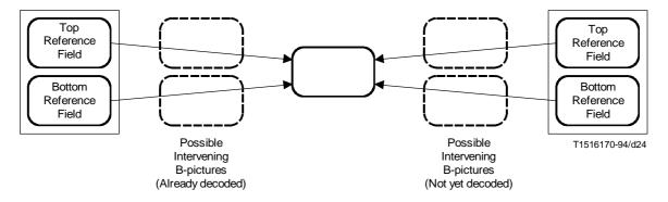
Figure 7-9 - Field-prediction of B-field pictures or B-frame pictures
