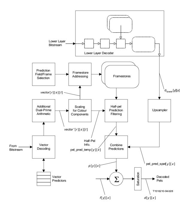
Figure 7-13 – Simplified motion compensation process for spatial scalability
