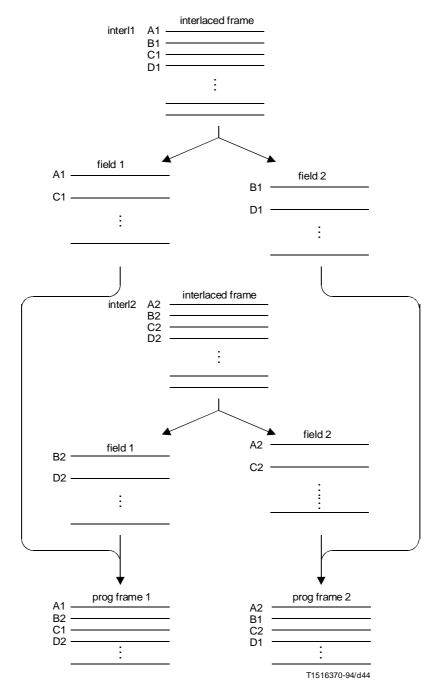
Figure D.4 – Two interlace to progressive conversion
