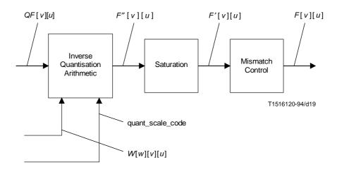
Figure 7-4 – Inverse quantisation process
