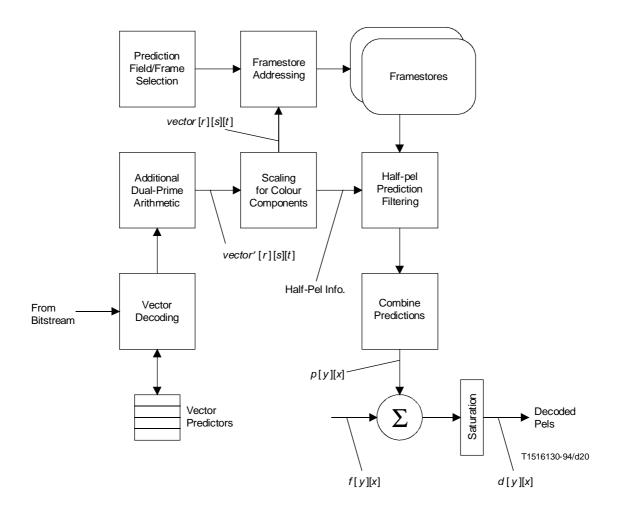
Figure 7-5 – Simplified motion compensation process
