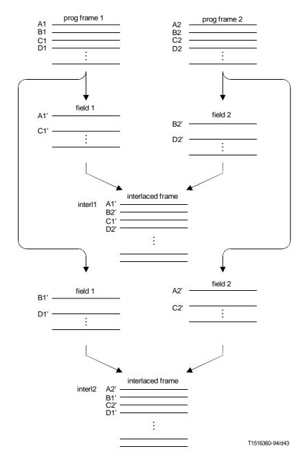
Figure D.3 – Progressive to two interlace conversion
