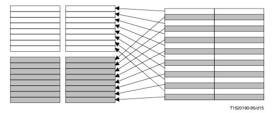
Figure 6-14 – Luminance macroblock structure in field DCT coding
