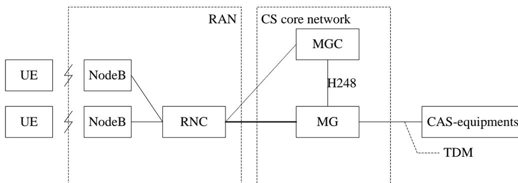
NOTE – Left side of MG: radio access network of the 3GPP defined 3G PLMN; Right side: legacy PSTN with a CAS-based NNI; Middle: 3GPP R3+ CS CN domain with Mc reference point between MSC server (MGC role) and CS-MGW.
