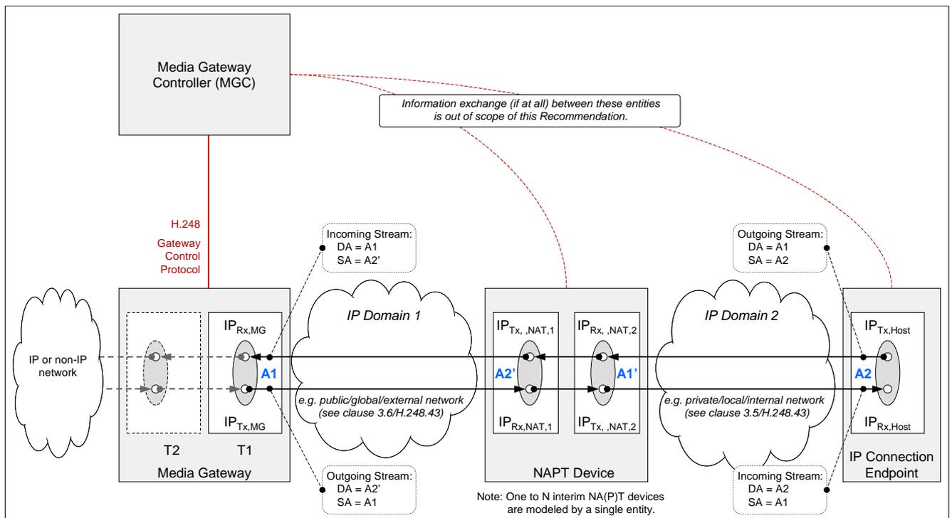
NOTE – The single H.248 stream at Termination T1 relates to the two IP flows of the bidirectional IP connection.
