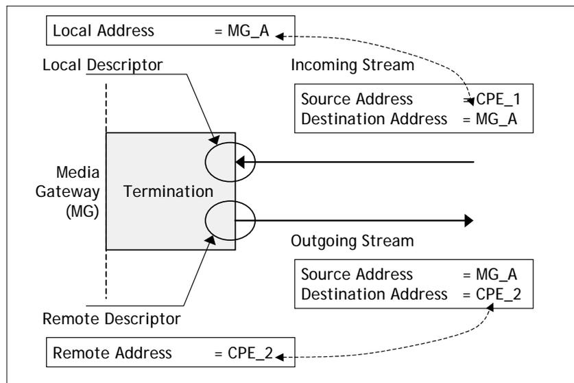
Figure 2 – NAT traversal processing OFF behaviour
