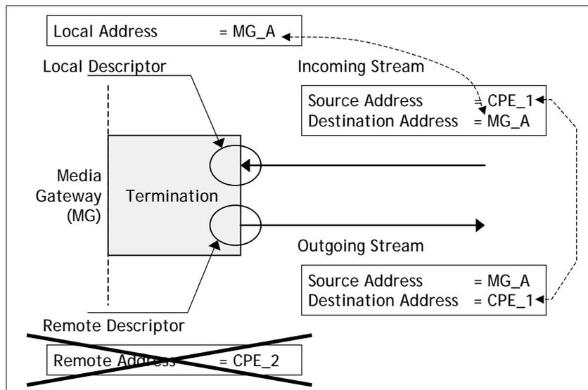
**Figure 3 – NAT traversal processing LATCH behaviour**
