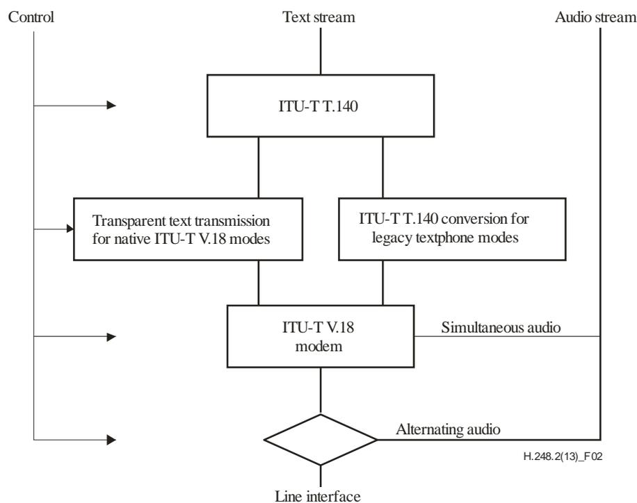
**Figure 2 – Text Telephone package functional view**
