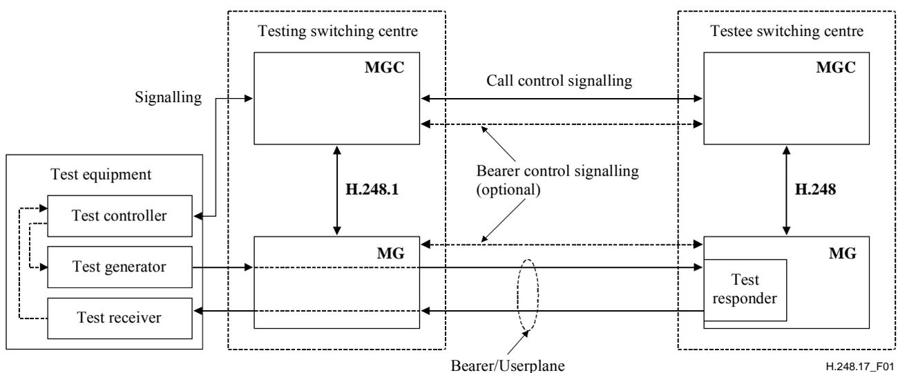
**Figure 1 – Test system architecture (TE separate)**
