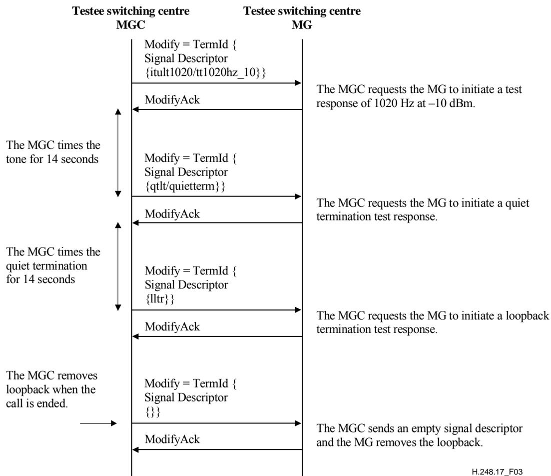
**Figure 3 – Analogue loopback test call flow**
