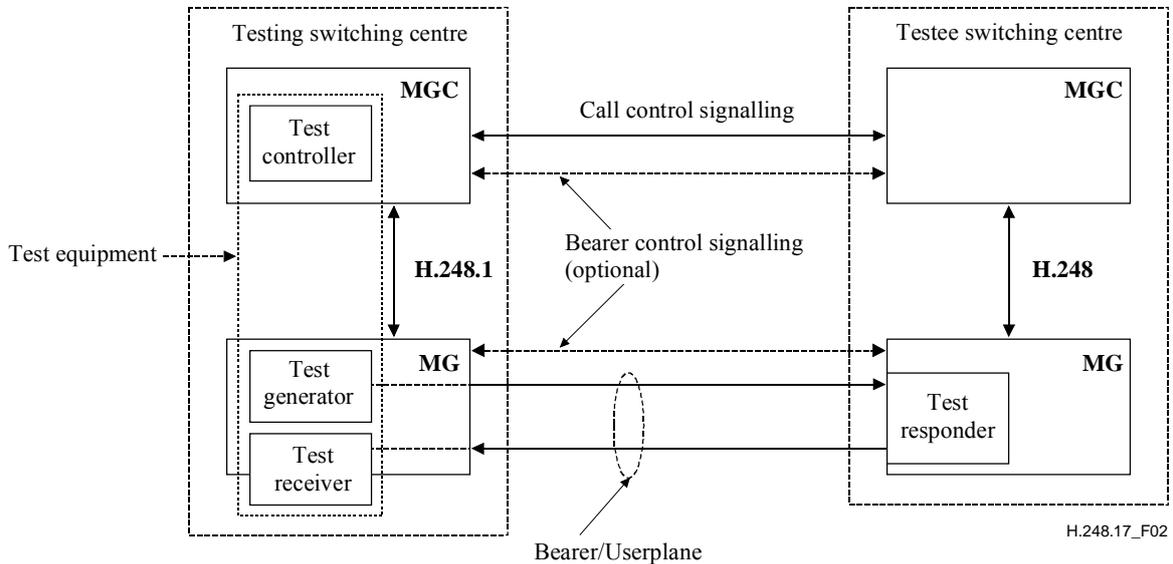
**Figure 2 – Test system architecture (TE combined)**
