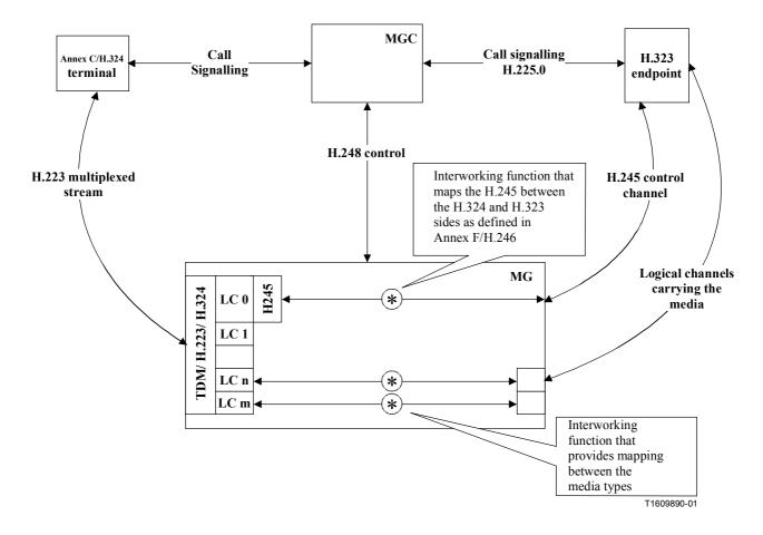
Figure 2/H.248.12 – Resource control at the MG (without fastStart/H.245 tunnelling)
