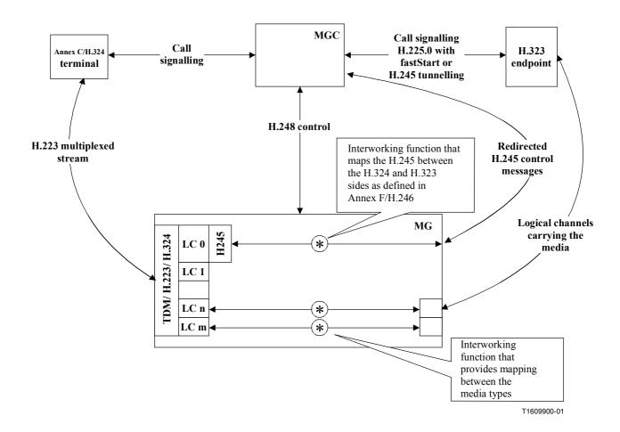
Figure 3/H.248.12 – Resource control at the MG (with fastStart/H.245 tunnelling)
