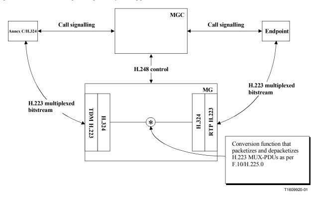
Figure 5/H.248.12 – Configuration for IP tunnelling of Annex C/H.324 bitstream
