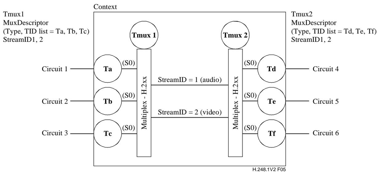
**Figure 5/H.248.1 – Multiplexed termination scenario – Circuit-to-circuit**
