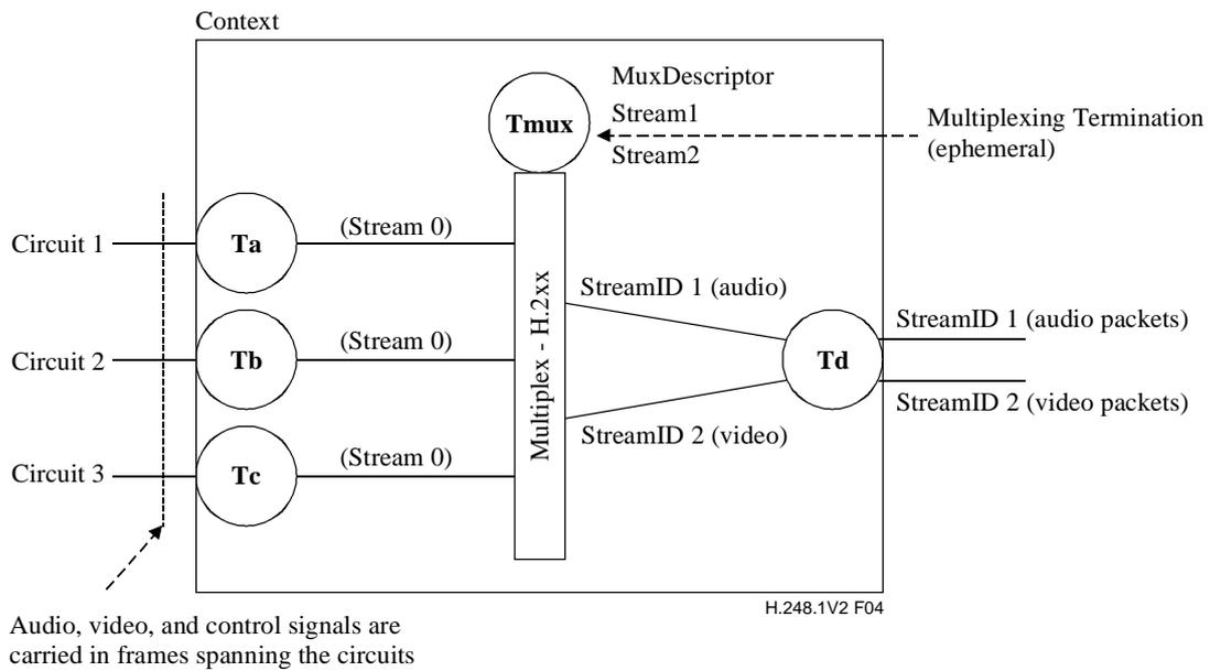
**Figure 4/H.248.1 – Multiplexed termination scenario – Circuit-to-packet**
