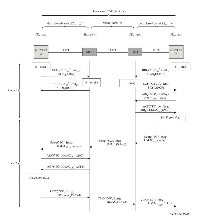
Figure G.10/H.235 – Example EP B calls EP A (multiple GK-routed) with MIKEY-PK-SIGN
