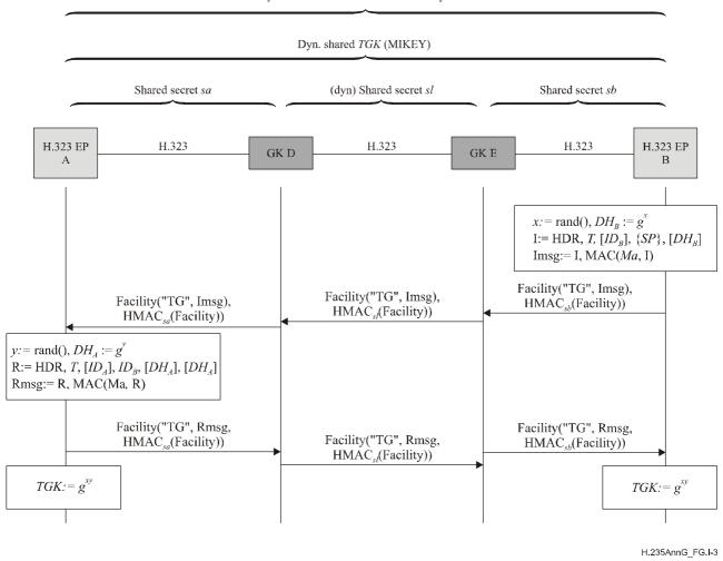
Figure G.I-3/H.235 – Example Endpoint B updating a key
