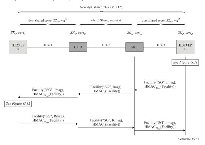
Figure G.14/H.235 – Example EP B (Initiator) initiated TGK re-keying and key update
