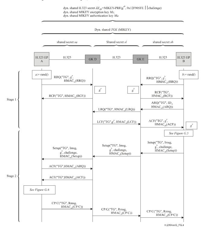
Figure G.4/H.235 – Example Endpoint B calling Endpoint A (GK-routed) with MIKEY-preshared
