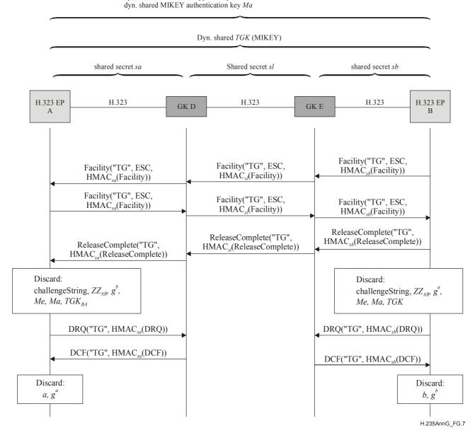
Figure G.7/H.235 – Example Endpoint B terminates a call
