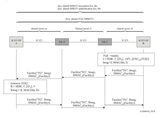
Figure G.8/H.235 – Example Endpoint B updating a key
