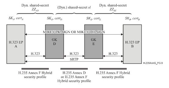
Figure G.9/H.235 – End-to-end scenario using PKI (multiple GKs)
