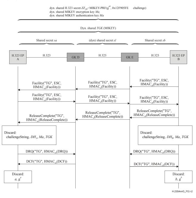
Figure G.I-2/H.235 – Example Endpoint B terminates a call
