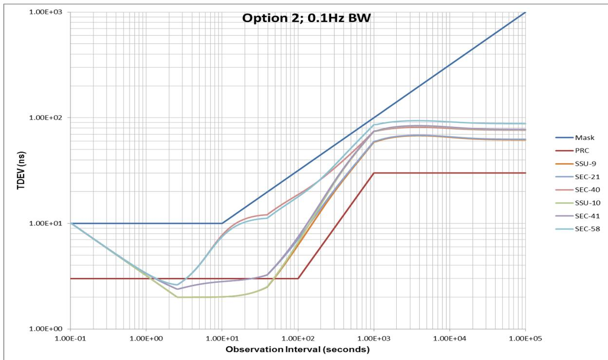
**Figure 59 – Option 2 TDEV results for PRC and selected SECs and SSUs**
