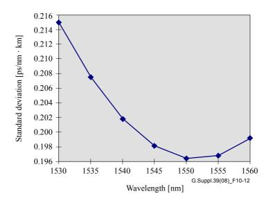
Figure 10-12 – Standard deviation of dispersion coefficient vs wavelength
