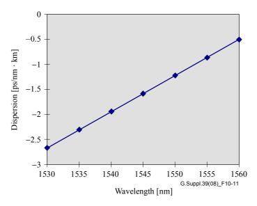
Figure 10-11 – Average dispersion coefficient vs wavelength
