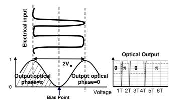
Figure 7-9 – Modulation configuration using MZM modulator for NRZ-DPSK generation
