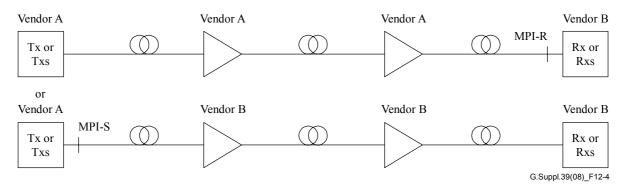
Figure 12-4 – Multi-span single interface transverse compatibility
