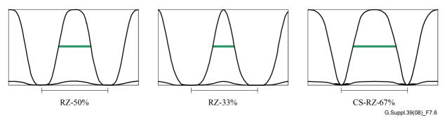
NOTE – The thin bar indicates the bit period T and the thick bar indicates the pulse width, corresponding to duty cycle.
