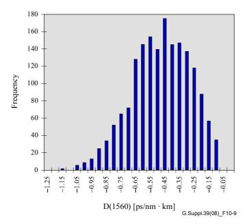
Figure 10-9 – Histogram of dispersion coefficient values at 1560 nm
