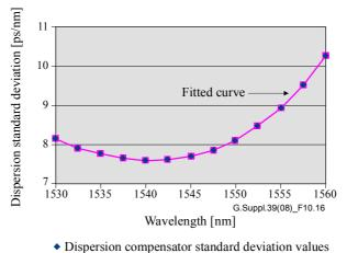
Figure 10-16 – Dispersion compensator standard deviation values
