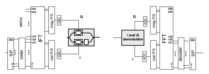
Figure 7-11 – Block diagram of Tx (left) and Rx (right) for O-OFDM
