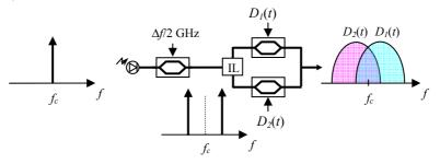
Figure 7-13 – Second transmitter scheme for two sub-carrier OFDM generation
