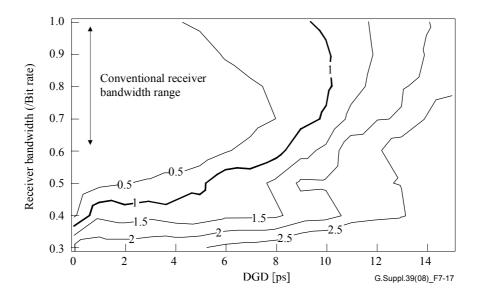
Figure 7-17 – Contour map for DGD tolerance (RZ-50%)
