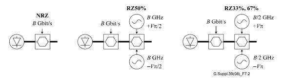
Figure 7-2 – Block diagram of NRZ and RZ format coding with MZM
