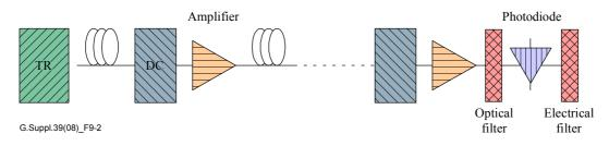
Figure 9-2 – Scheme of the system with periodic post-compensation
