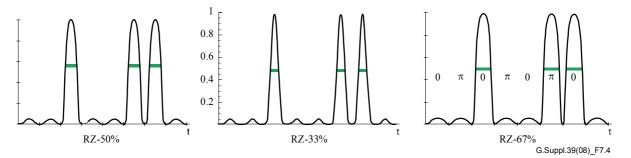
NOTE – The bar indicates FWHM and the duty cycle of the pulses.  $\pi$  and 0 indicate the phase change of RZ pulses at CS-RZ-67%.
