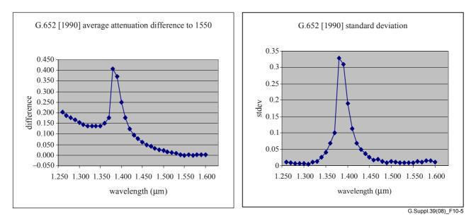
Figure 10-5 – Average and standard deviation of difference in attenuation coefficient from 1550 nm – G.652 circa 1990
