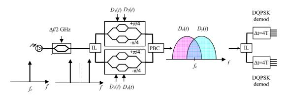
Figure 7-14 – OPFDM-DQPSK generation and detection scheme
