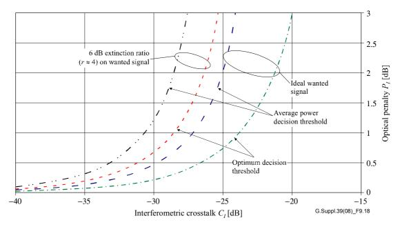
Figure 9-18 – Graph of optical penalty vs interferometric crosstalk for multiple interferers (Gaussian model)
