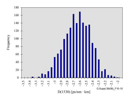
Figure 10-10 – Histogram of dispersion coefficient values at 1530 nm
