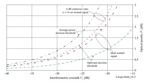
Figure 9-17 – Graph of optical penalty vs interferometric crosstalk for a single interferer (bounded model)
