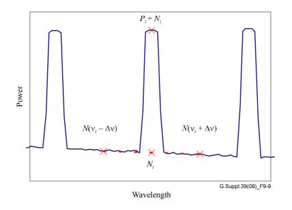
Figure 9-9 – OSNR measurement from the optical spectrum
