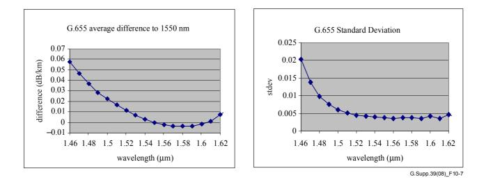
Figure 10-7 – Average and standard deviation of difference in attenuation coefficient from 1550 nm – G.655
