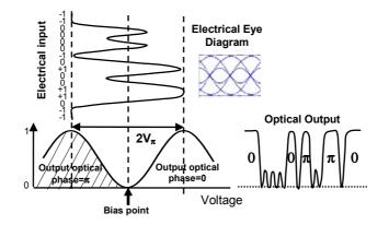
Figure 7-7 – Modulation configuration of ODB (PSBT)
