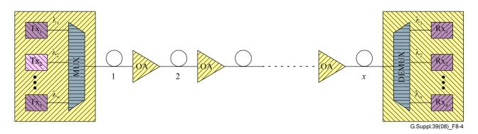
Figure 8-4 – Example of a WDM point-to-point link
