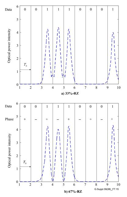
Figure 7-15 – 40-Gbit/s pulse form after accumulated dispersion of 20 ps/nm
