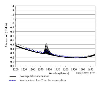
Figure 10-4 – Measured fibre attenuation and splice loss in installed G.652 A&B cable – Cables installed in 2003
