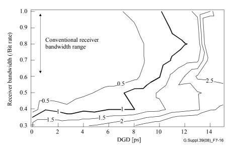
Figure 7-16 – Contour map for DGD tolerance (RZ-33%)
