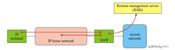
Figure 11-1 – Remote end device management configuration
