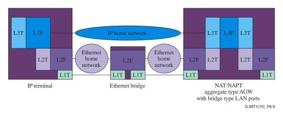
Figure 8-5 – An example of home network functional architecture
