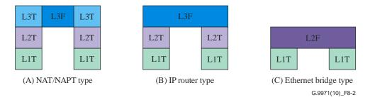
Figure 8-2 – Functional components of separate type AGW
