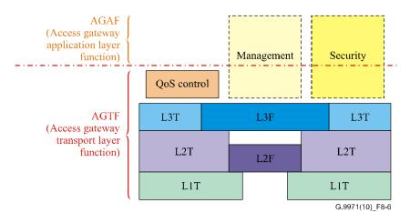
**Figure 8-6 – Functional architecture of separate type AGW**
