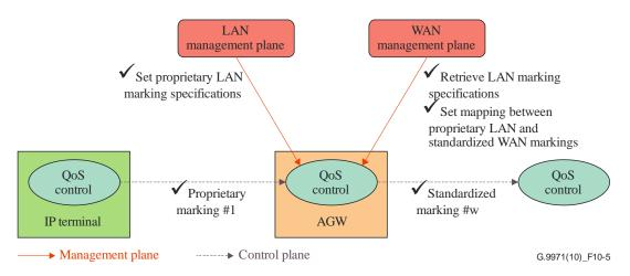
Figure 10-5 – A realization of hop-by-hop QoS guaranteed services in QoS service type 2
