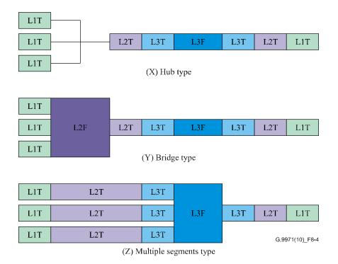
Figure 8-4 – LAN side physical ports of NAT/NAPT separate type AGW
