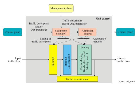
Figure 10-4 – Functional architecture for QoS control
