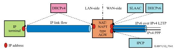
Figure 9-5 – IPv6 over L2TP over IPv4 to AGW with IPv4 to IP terminal
