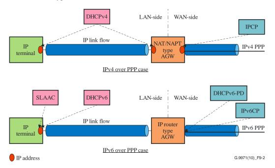
Figure 9-2 – Either IPv4 over PPP or IPv6 over PPP connection to AGW
