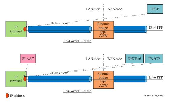
Figure 9-3 – Either IPv4 over PPP or IPv6 over PPP connection to IP terminal
