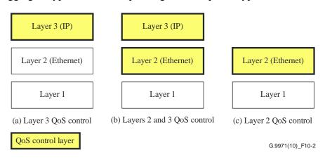
Figure 10-2 – Three device types for QoS control
