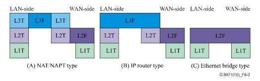
Figure 8-3 – Functional components of aggregate type AGW
