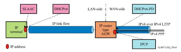
Figure 9-4 – IPv6 over L2TP over IPv4 to AGW with IPv6 to IP terminal
