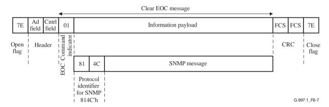
Figure 6-7 – OAM communication channel protocol over the U-interface
