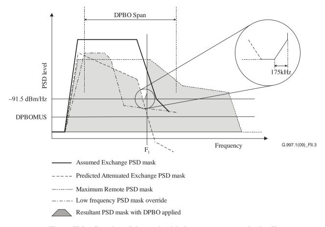
Figure II.3 - Creation of the mask with downstream power back-off
