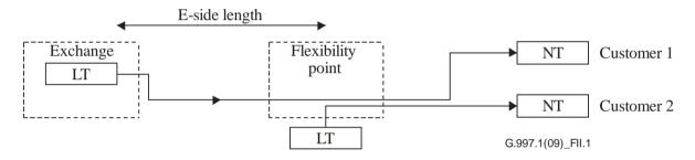
Figure II.1 – Physical layer reference model
