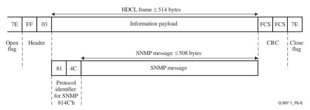
Figure 6-6 – OAM communication channel protocol over the U-interface
