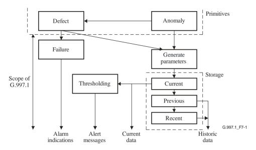
Figure 7-1 – In-service performance monitoring process
