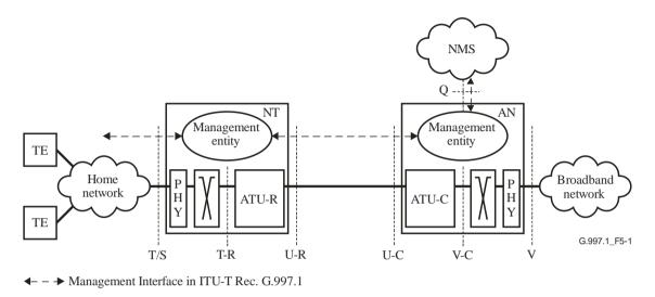
Figure 5-1 – System reference model
