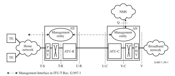
Figure 5-1 – System reference model
