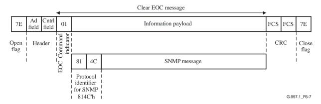
Figure 6-7 – OAM communication channel protocol over the U-interface
