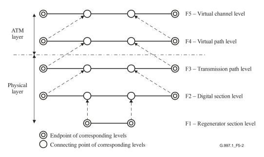
Figure 5-2 – OAM hierarchical levels and their relationship with the ATM layer and physical layer
