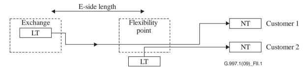
Figure II.1 – Physical layer reference model
