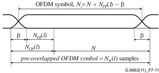
**Figure 7-11 – Structure of an OFDM symbol with cyclic extension and overlapped windowing**
