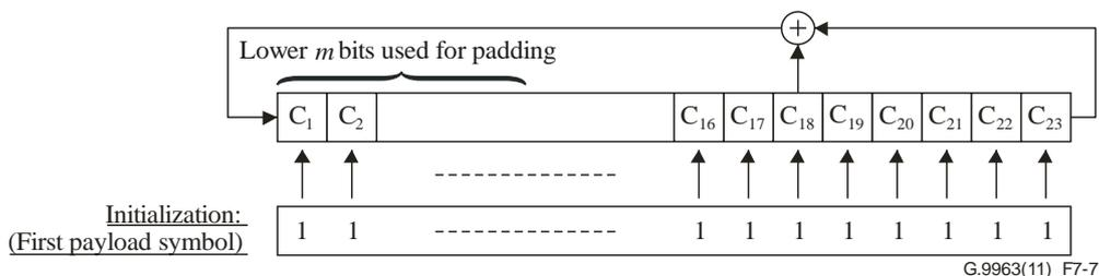
**Figure 7-7 – LFSR for modulation of unloaded and partially loaded sub-carriers for each of the two spatial streams**
