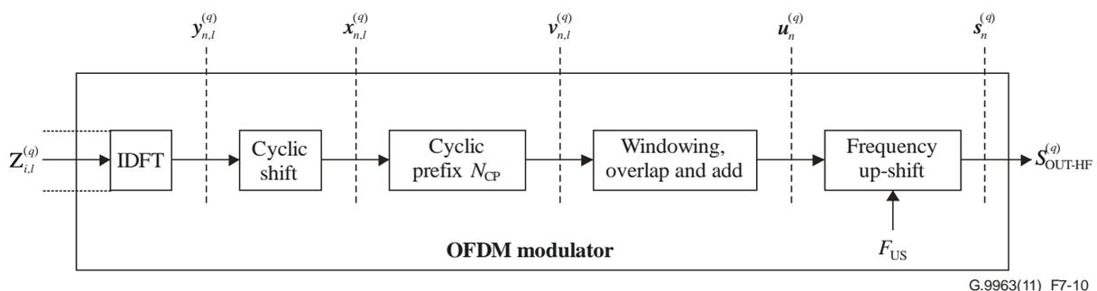
Figure 7-10 – Functional model of the OFDM modulator
