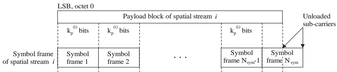
Figure 7-5 – Payload segmentation of the payload block of spatial stream  $i$  ( $i=1,2$ )
