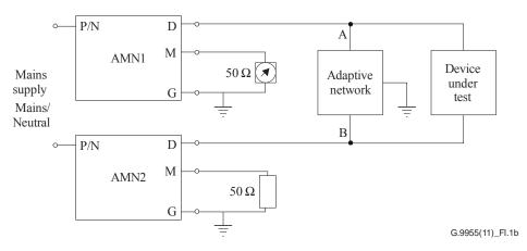
NOTE – AMN1 to AMN2 are artifical mains networks conforming to subclause 11.2 of [CISPR 16-1] (example Figure 5 / 9-148.5 kHz)
