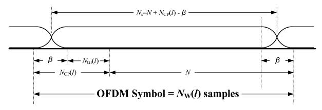
Figure 7-22 – Structure of an OFDM symbol
