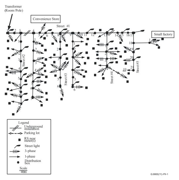
Figure II.1 – Example of neighbourhood AMI/AMM installation diagram
