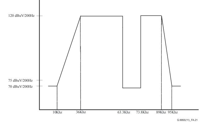
Figure A.21 – Spectrum with two notches inserted to cohabitate with S-FSK PLC modem
