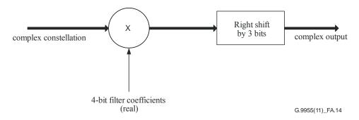
Figure A.14 – Block diagram of the pre-emphasis filter
