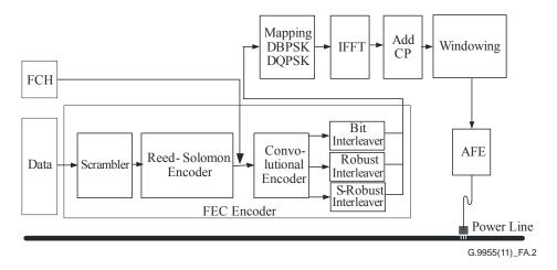
Figure A.2 – Block diagram of OFDM transceiver
