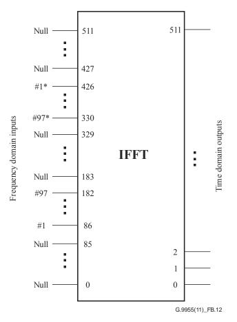
Figure B.12 – Subcarrier mapping
