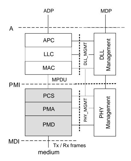
Figure 5-7 – Functional model of ITU-T G.9955 transceiver
