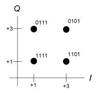
Figure 7-19 – Constellation mapping for  $b = 4 (d_3d_2d_1d_0, \text{ first quadrant})$
