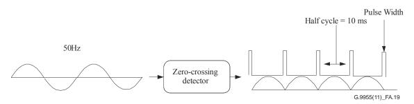
Figure A.19 – Zero crossing detector
