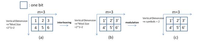
Figure A.11 – Example of interleaving with DBPSK
