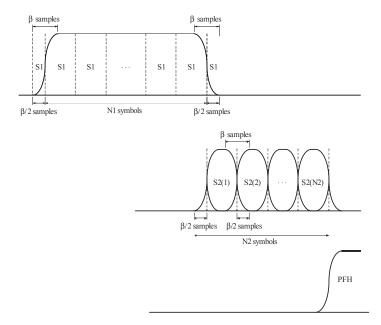
Figure M.1 – Time-domain preamble symbol generation for ERM
