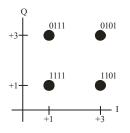
Figure E.1 – 16-QAM constellation diagram
