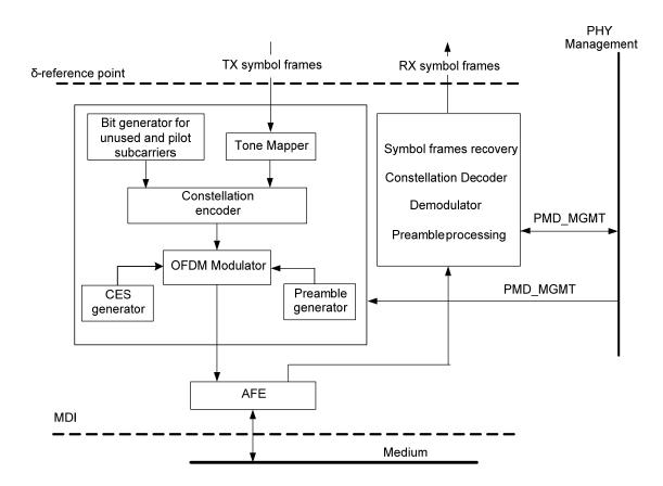
Figure 7-16 – Functional model of PMD
