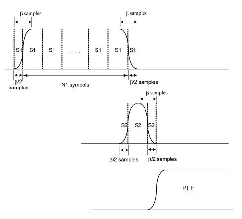
**Figure 7-25 – Preamble time-domain generation**
