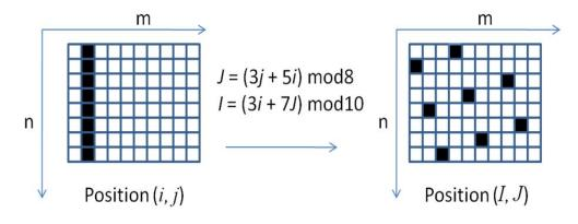
Figure A.10 – Example of spreading behaviour
