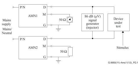
NOTE – AMN1 to AMN2 are artifical mains networks conforming to subclause 11.2 of [CISPR 16-1] (example Figure 5 / 9-148.5 kHz)
