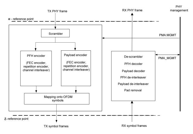
Figure 7-5 – Functional model of PMA
