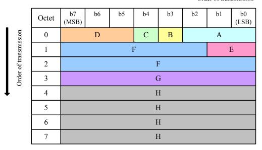
Figure 6-1 – Example of mapping fields onto groups of octets
