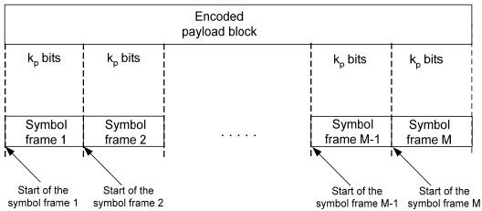
Figure 7-15 – Payload mapping
