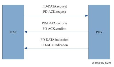
Figure A.22 – Data or ACK primitive flow
