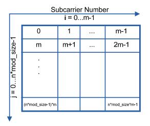
Figure A.8 – Bit order input into the input buffer
