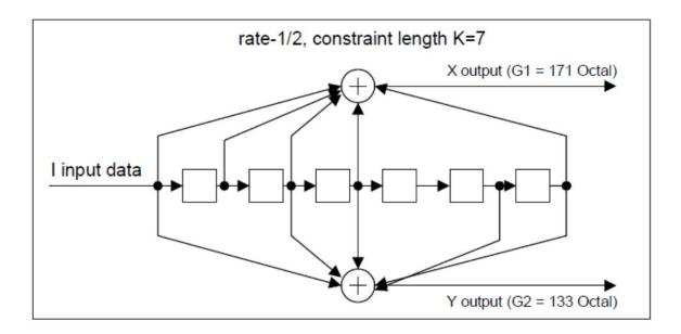
Figure 7-8 – Inner convolutional code encoder
