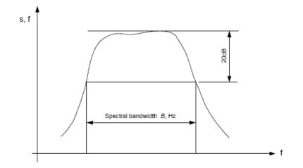
Figure 7-27 – Measurement of spectral bandwidth
