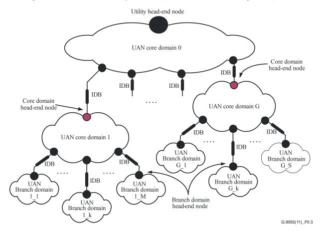
Figure II.3 – Example of UAN with multiple domains
