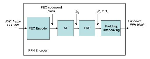
Figure 7-12 – Functional diagram of the PFH encoder
