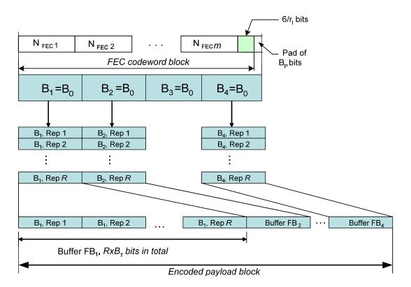
Figure 7-10 – Generation of the encoded payload block (case  $N_{\rm frg}$  = 4, cyclic shifting, interleaving and padding of fragments when in IoAC mode is not shown)
