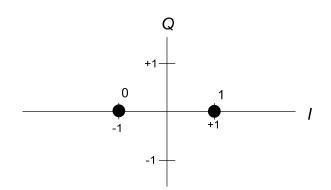
Figure 7-20 – Constellation mapping for b = 1 ( $d_0$ )
