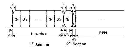
Figure 7-23 – Preamble structure ( $N_2 = 1$ )
