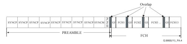
Figure A.4 – ACK/NACK frame structure
