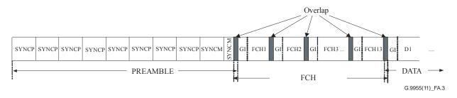
Figure A.3 – Typical data frame structure
