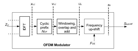
**Figure 7-21 – Functional diagram of the OFDM modulator**
