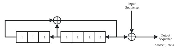
Figure B.10 – LFSR for use in the scrambler block
