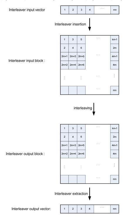
Figure 7-14 – Order of writing in and reading out of the permutation matrix
