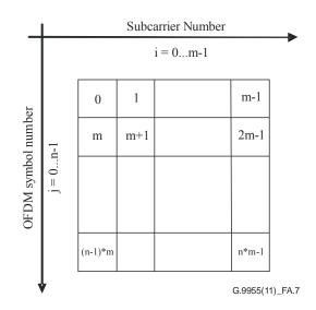
Figure A.7 – Bit order input into the Interleaver buffer
