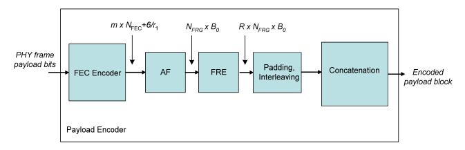
Figure 7-9 – Functional diagram of the payload encoder
