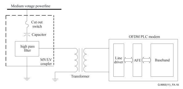
Figure A.18 – Proposed coupling circuit
