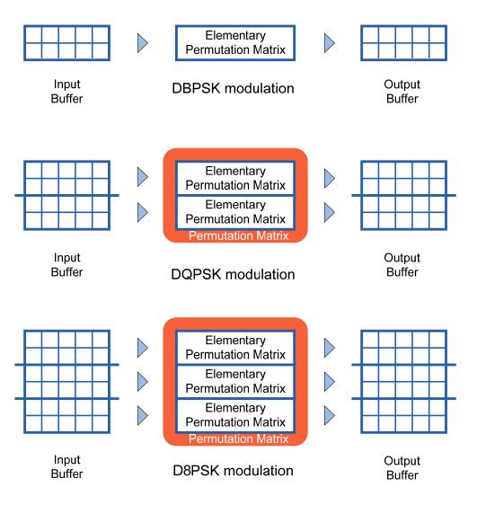
Figure A.9 – Permutation matrix used with different modulations
