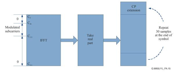
Figure A.15 – IFFT input/output and CP addition
