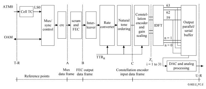
NOTE – The TTR<sub>R</sub> shall be generated in the ATU-R from the received  $TTR_C$ , and shall be locked to 690 periods of upstream sampling clock (276 kHz).
