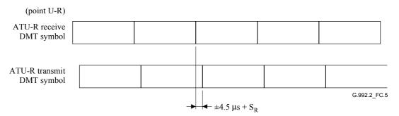
Figure C.5/G.992.2 – Loop timing for ATU-R
