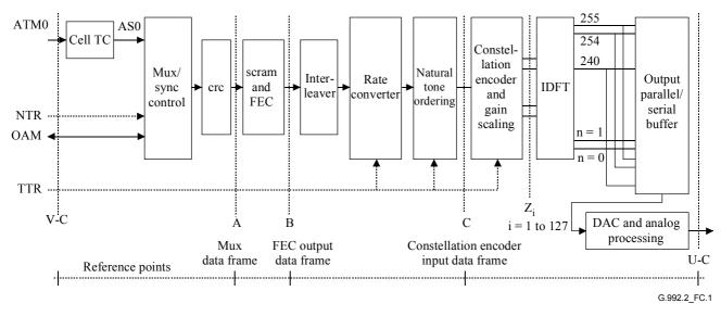
NOTE - The TTR may be generated in the ATU-C without being provided from the V-C reference point TCM-ISDN clock.
