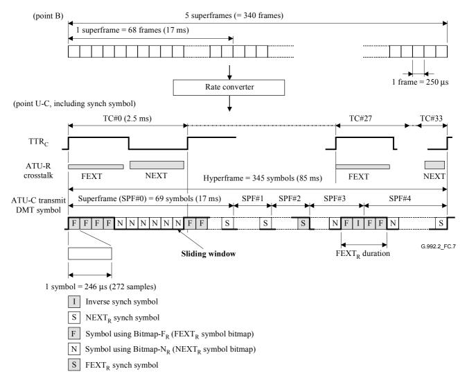
Figure C.7/G.992.2 – Hyperframe structure for downstream
