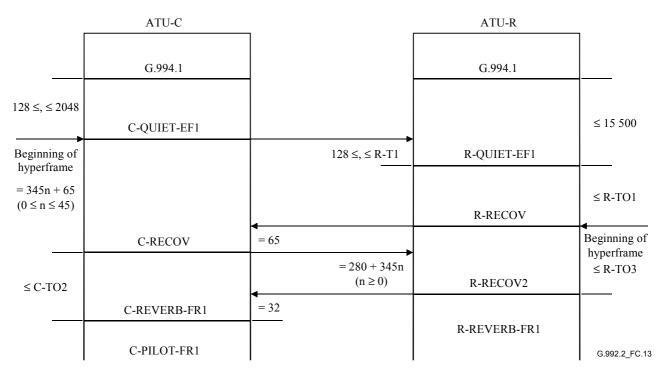
Figure C.13/G.992.2 – Timing diagram of Escape to Fast Retrain
