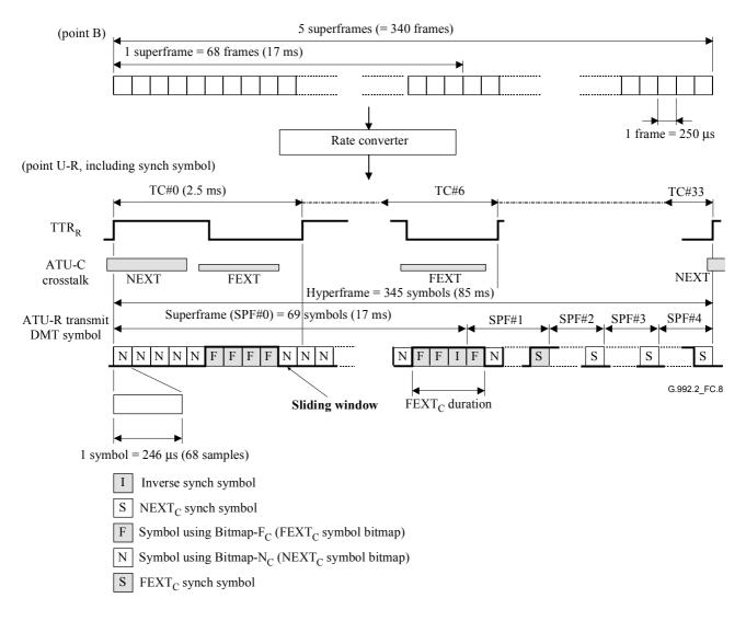
Figure C.8/G.992.2 – Hyperframe structure for upstream
