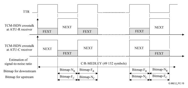
Figure C.15/G.992.2 – Estimation of periodic Signal-to-Noise Ratio
