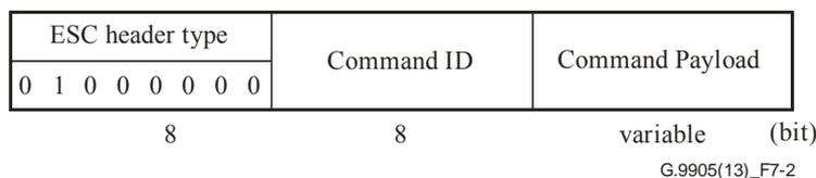
**Figure 7-2 – ADP command frame header**
