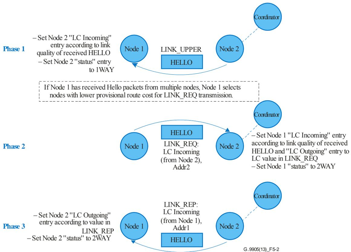
**Figure 5-2 – Establishment of 2WAY link using LINK\_REQ/LINK\_REP sub-messages**
