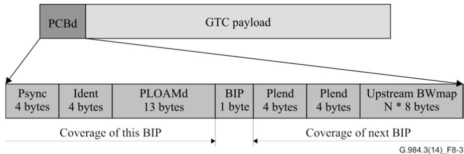
**Figure 8-3 – GTC physical control block downstream (PCBd)**
