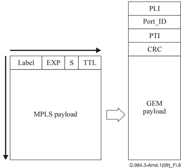
Label: Label value, EXP: Experimental use, S: Bottom of stack
