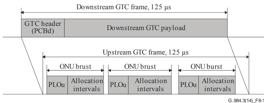
**Figure 8-1 – GTC layer framing**
