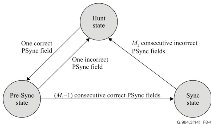
**Figure 8-4 – GTC downstream ONU synchronization state machine**
