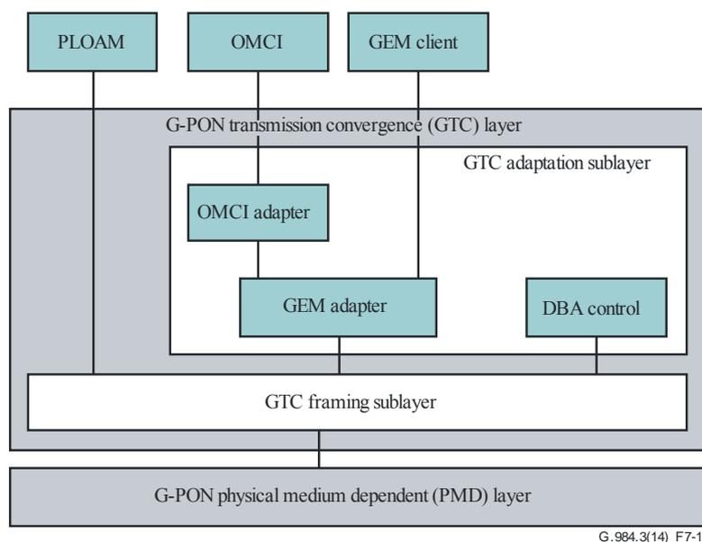
**Figure 7-1 – Protocol stack for the GTC**
