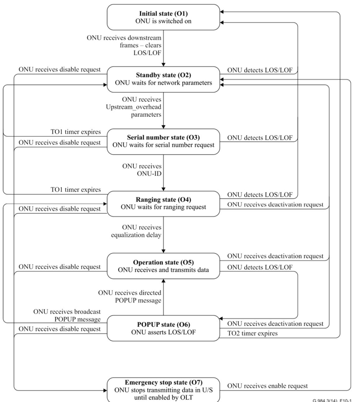
Figure 10-1 – The state diagram of the ONU
