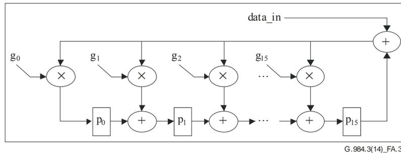
**Figure A.3 – IIR model for FEC encoder**
