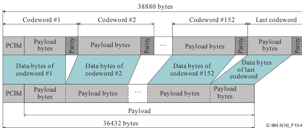
**Figure 13-4 – Payload reconstruction at the FEC decoder**
