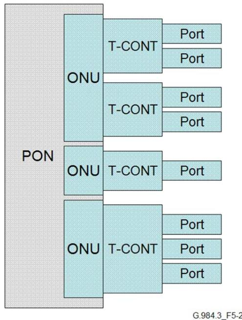
**Figure 5-2 – Upstream multiplexing**
