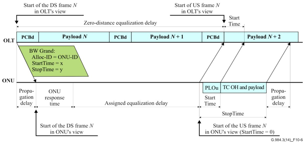
**Figure 10-6 – Timing relationships in the Operation state**
