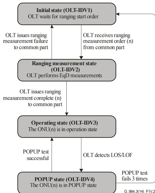
Figure IV.2 – ONU-specific part state diagram
