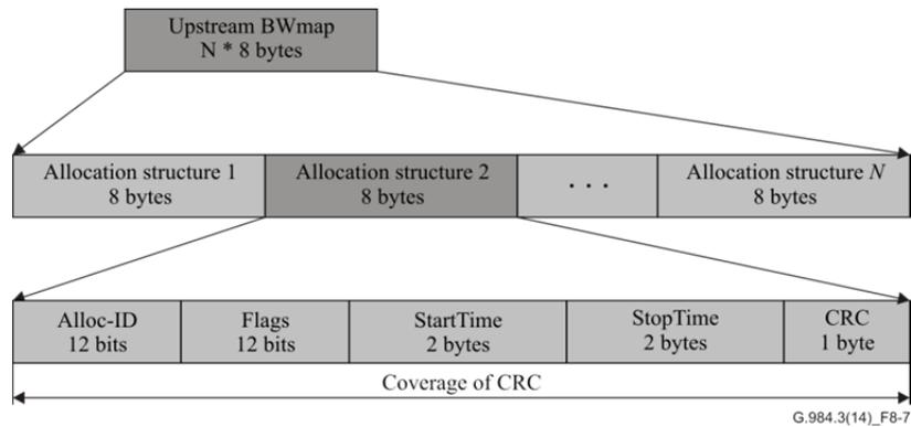
**Figure 8-7 – GTC bandwidth map allocation structure**
