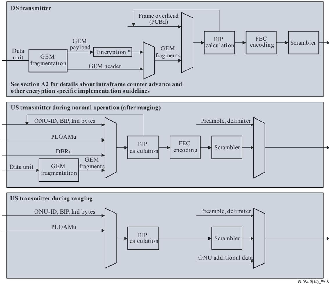
Figure A.8 – Transmitter block diagram
