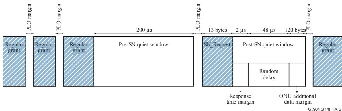
Figure A.6 – Serial number request example
