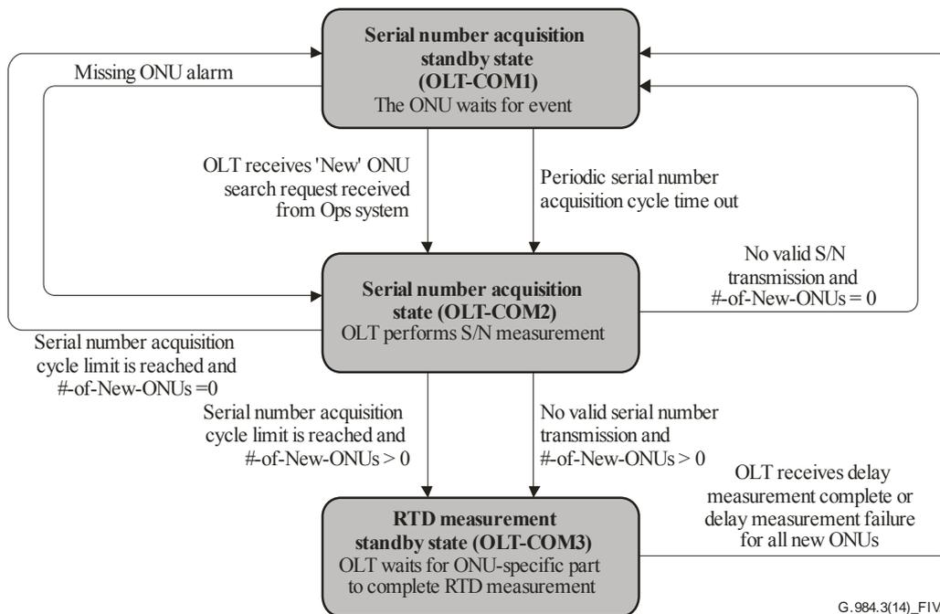
Figure IV.1 – OLT common part state diagram
