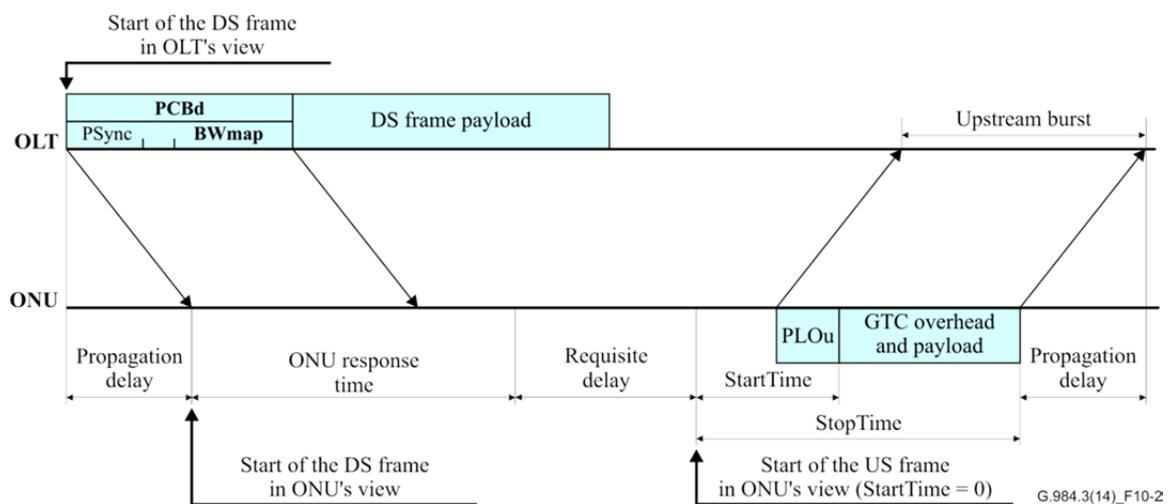
**Figure 10-2 – ONU timing diagram – General case**
