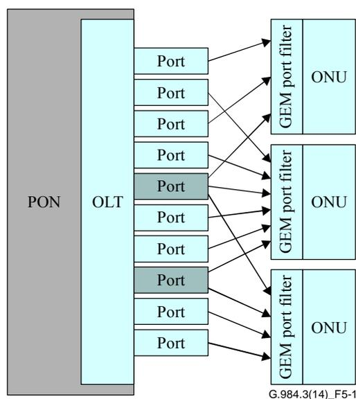
**Figure 5-1 – Downstream multiplexing (shaded GEM port indicates multicast)**
