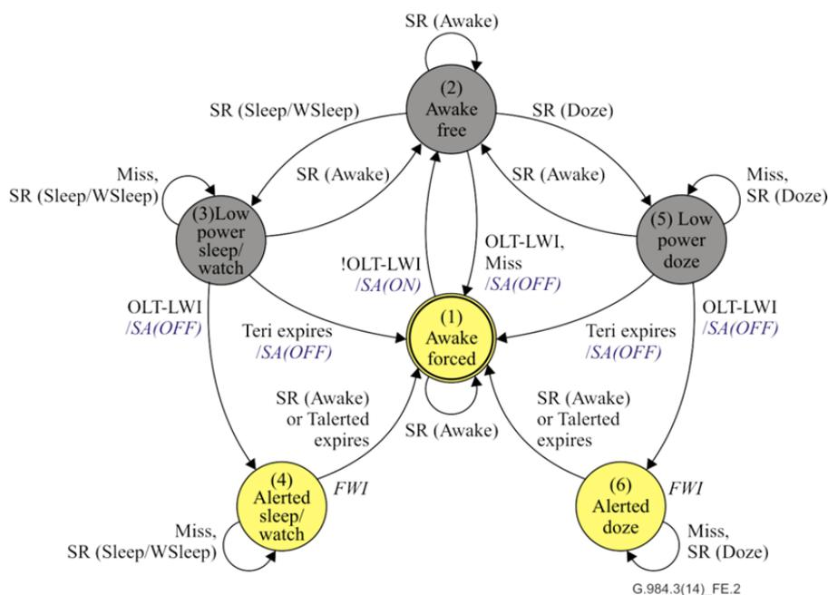
**Figure E.2 – OLT state transition diagram (initial state circled)**
