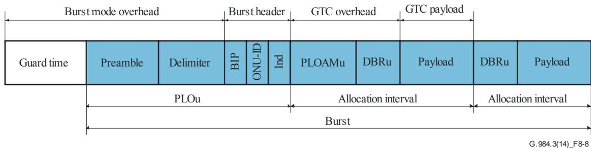
**Figure 8-8 – Details of physical and GTC layer upstream overhead**
