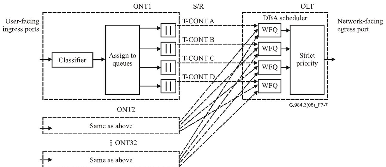
**Figure 7-7 – An example of a queuing and scheduling architecture that can be specified under the extended bandwidth assignment model**
