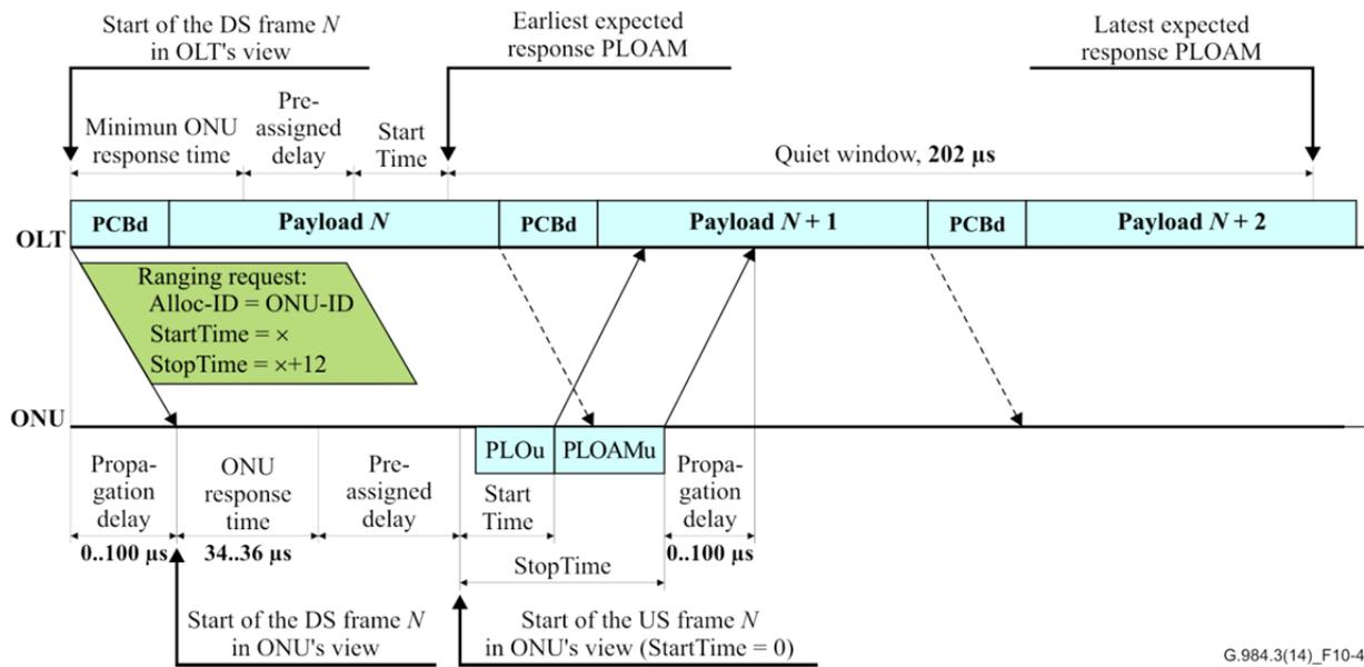
NOTE – The dash communication arrows denote the start of transmission of the subsequent downstream GTC frames (i.e., frames  $N+1$ ,  $N+2$ , etc.), whereas the solid communication arrows denote the significant instances associated with transmission of GTC frame  $N$  (in both downstream and upstream directions).
