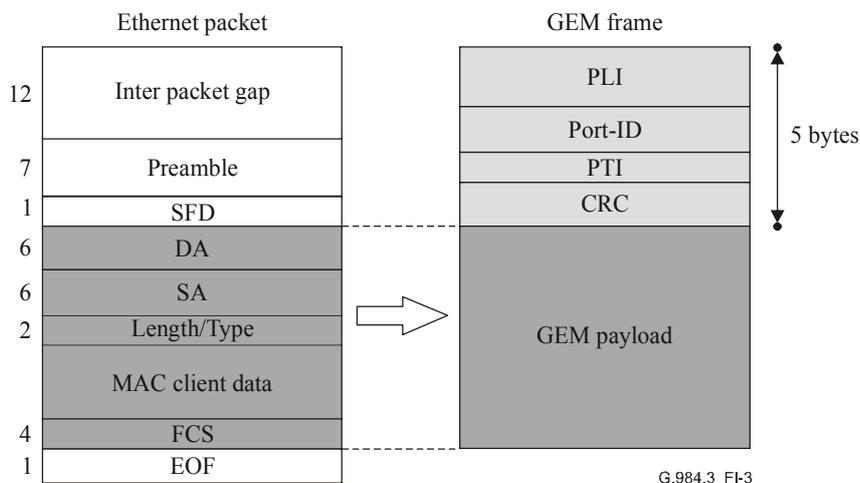
**Figure I.3 – Frame structure for Ethernet mapping into GEM frame**
