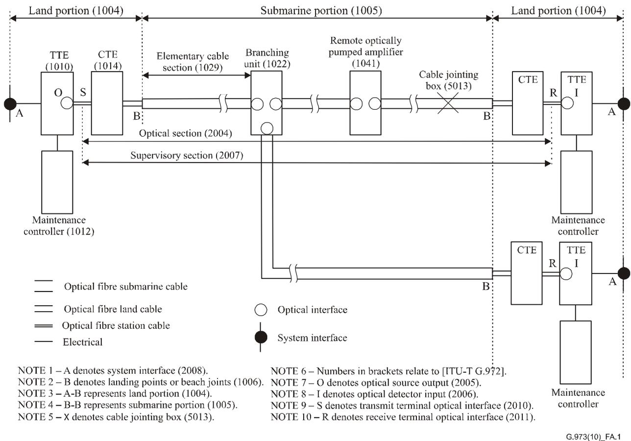
**Figure A.1 – Example of repeaterless optical fibre submarine cable system**
