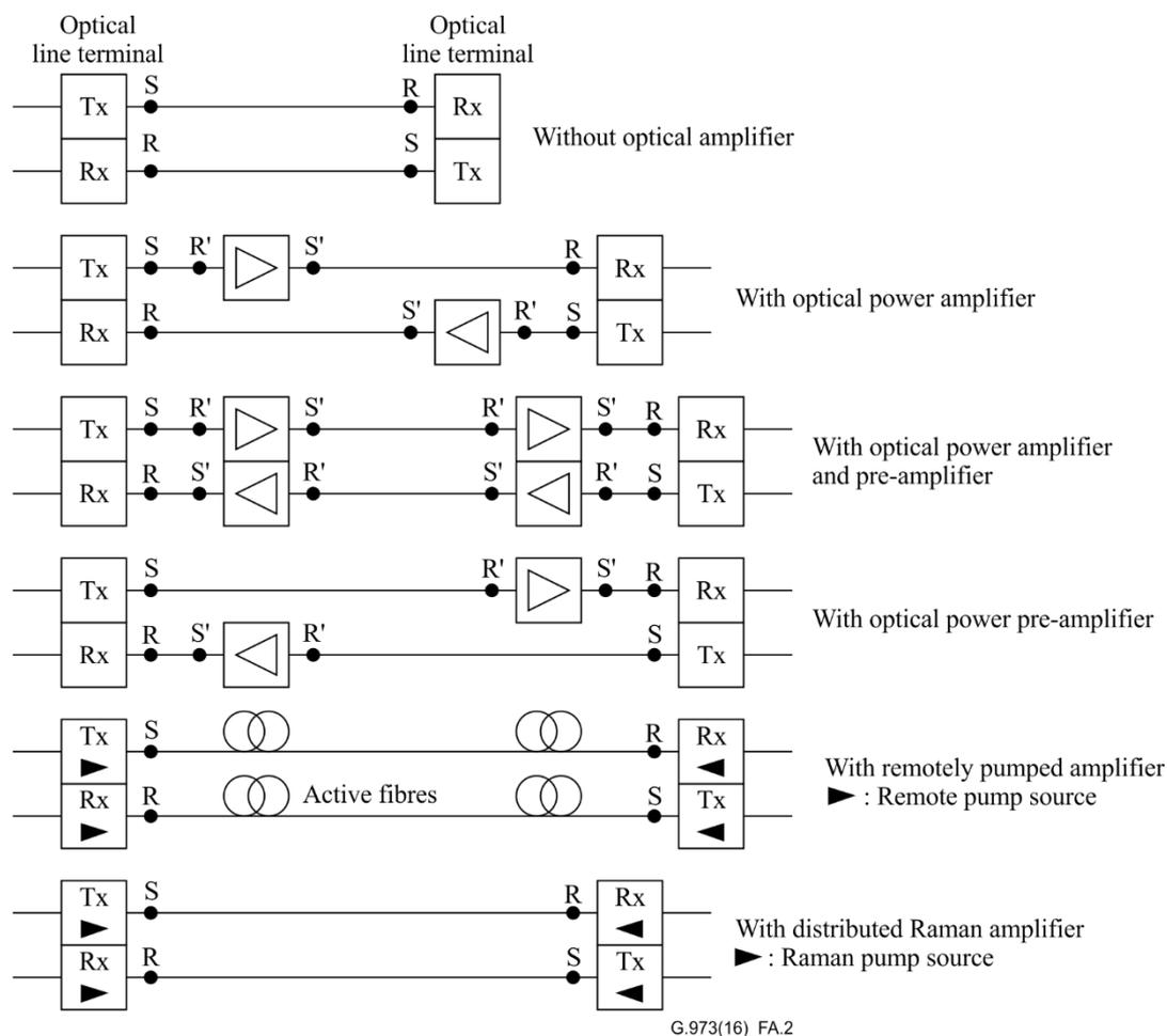
Figure A.2 – Possible system configurations
