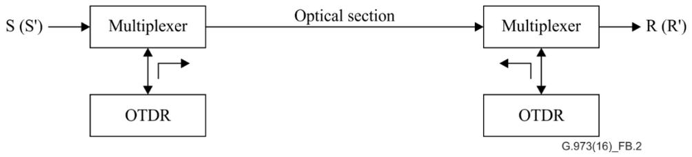
**Figure B.2 – Example of line monitoring using OTDR**
