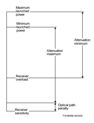
FIGURE 3/G.957 Relationship of the optical parameters
