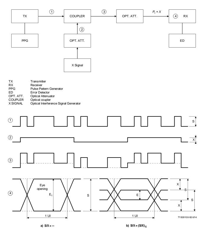
FIGURE II.4/G.957 S/X measurement configurations
