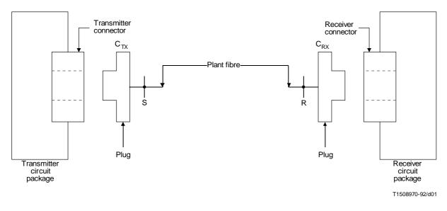
FIGURE 1/G.957 Representation of optical line system interface
