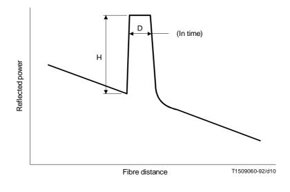
FIGURE 1.2/G.957 OTDR trace at a discrete reflector
