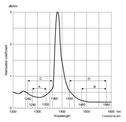
Ranges A and B are suitable for long-haul (L-N.x) applications, and ranges C and D are suitable for short-haul (S-N.x) and intra-office (I-N) applications.
