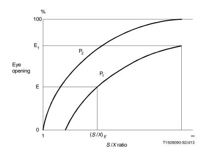
FIGURE II.3/G.957 Eye opening and *S/X* ratio parameter
