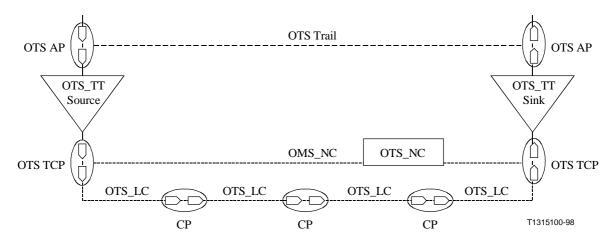
Figure 4/G.872 – OTS layer network example
