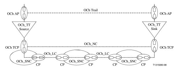
Figure 2/G.872 – OCh layer network example
