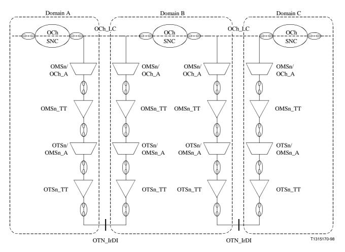
Figure 11/G.872 – Scenario 3: Interconnection of OTN subnetworks in different administrative domains via an OTN inter-domain interface supporting OCh interworking
