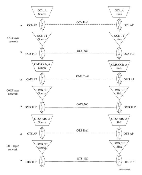
Figure 1/G.872 – Client server associations in an optical transport network
