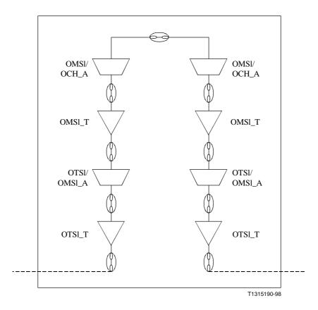
Figure I.1/G.872 – Example of optical wavelength conversion
