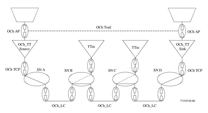
Figure 6/G.872 – Example of subnetwork connection supervision using non-intrusive monitoring
