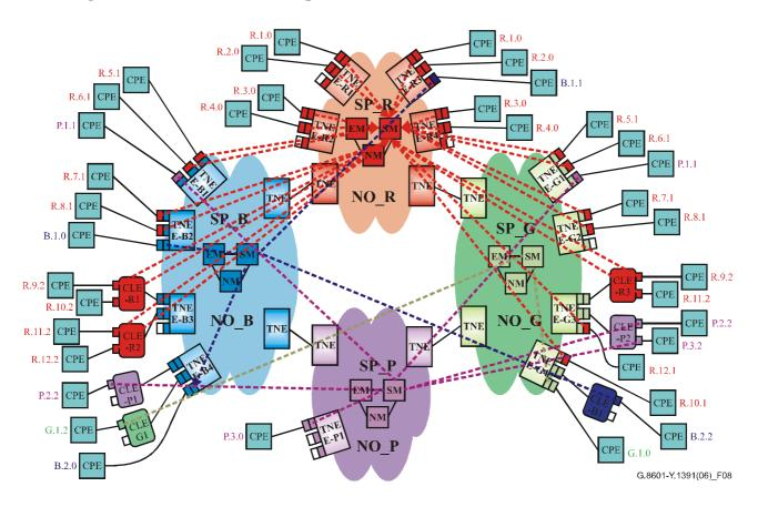
Figure 8/G.8601/Y.1391 – Composite network scenario showing service management signal flows
