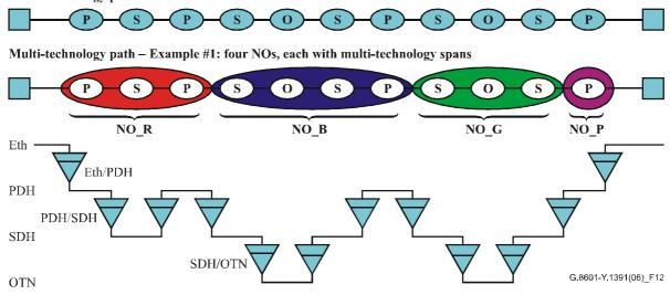
Figure 12/G.8601/Y.1391 – Multi-technology, multi-carrier transport path combinations showing dittering technology I/F at carrier boundary
