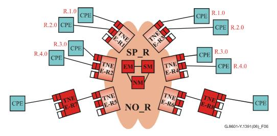
Figure 6/G.8601/Y.1391 – Single carrier scenario – Edge device is incompatible with NO management systems
