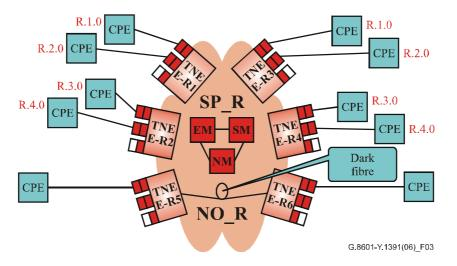
Figure 3/G.8601/Y.1391 – Single carrier (Dark fibre connection)
