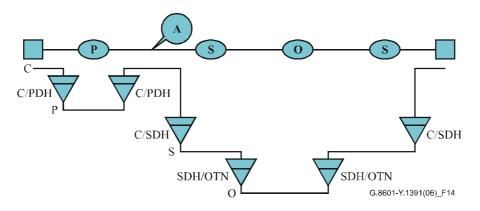
Figure 14/G.8601/Y.1391 – Example of 'Different-transport-technology' edges
