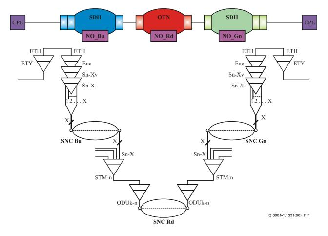
Figure 11/G.8601/Y.1391 – Functional model of SDH:OTN:SDH network
