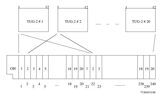
Figure 3-7/G.832 – Multiplexing of  $20 \times TUG-2$  into the 139 264 kbit/s payload capacity
