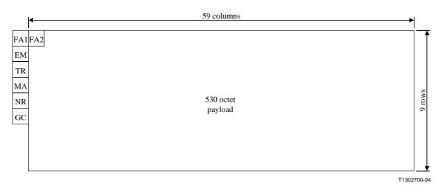
Figure 2-1/G.832 – Frame structure at 34 368 kbit/s
