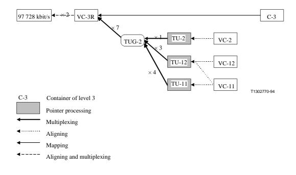
NOTE - The VC-3R is a VC-3 SDH element with reduced functionality as shown in Figure 2-4.
