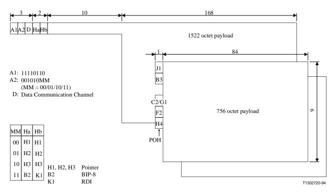
Figure 2-4/G.832 – Frame structure and overhead allocation for the 97 728 kbit/s
