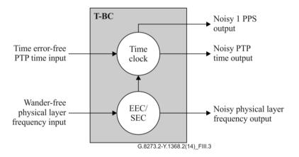
Figure III.3 – Noise generation of a T-BC
