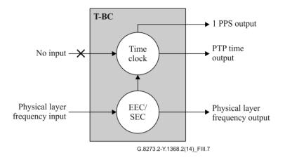
Figure III.7 – Physical layer frequency-assisted holdover
