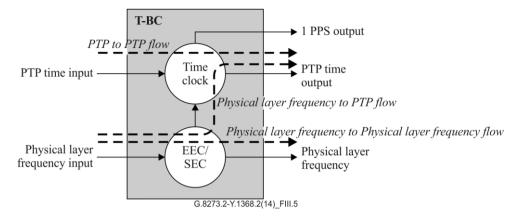
Figure III.5 – Signal flows through a T-BC
