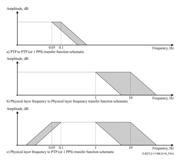
Figure III.6 – Generalized transfer function schematics of a T-BC
