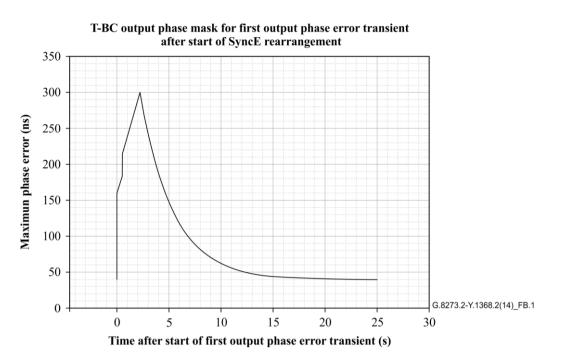
Figure B.1 – Phase error limit for first output phase error transient after the start of the SyncE/SDH rearrangement
