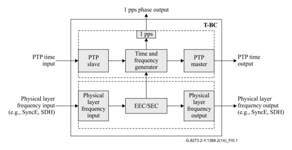
Figure III.1 – Model of T-BC showing signal flows in normal operation
