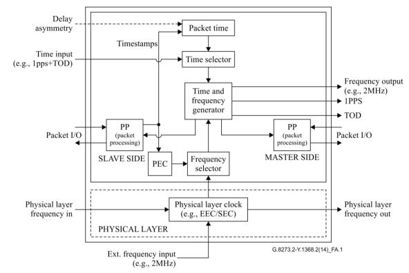
Figure A.1 illustrates a telecom boundary clock model.
