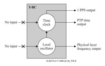
Figure III.8 – Unassisted holdover
