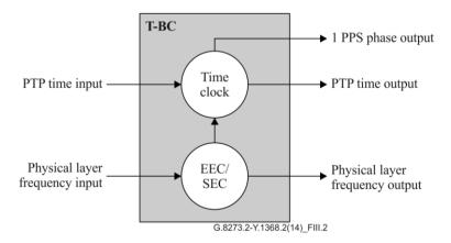
Figure III.2 – Simplified model of T-BC showing clocks
