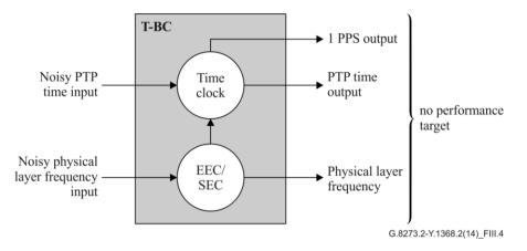
Figure III.4 – Noise tolerance of a T-BC
