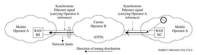
Figure 12-2 – Illustration of a timing transparent transport of the synchronous Ethernet client signals in the multi-operator context
