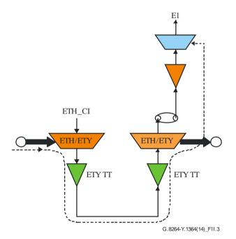
Figure II.3 – Example of using physical layer timing to provide timing to an ETH/PDH adaptation function
