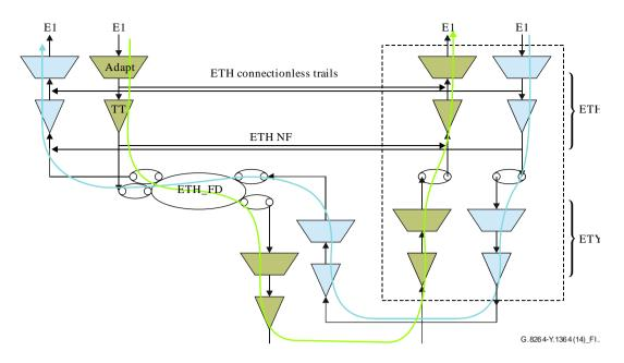
Figure I.2 – ITU-T G.8010 Ethernet network architecture showing circuit emulation and timing trails
