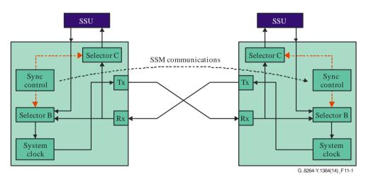
Figure 11-1 – Simplified SSM channel
