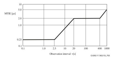
Figure 5 – Input wander tolerance (MTIE) for EEC-Option 1
