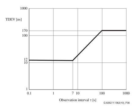
Figure 6 – Input wander tolerance (TDEV) for EEC-Option 1
