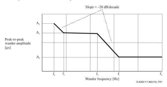
Figure 7 – Lower limit of maximum tolerable sinusoidal input wander for EEC-Option 1
