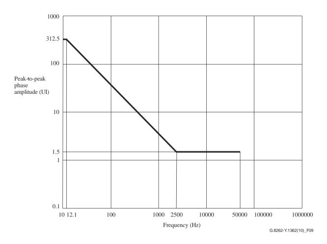
Figure 9 – 1G synchronous Ethernet wideband jitter tolerance for EEC-Option 1 and EEC-Option 2
