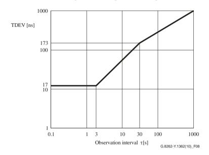
Figure 8 – Input wander tolerance (TDEV) for EEC-Option 2
